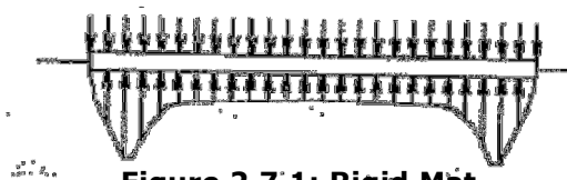
Figure 2.7.1: Rigid Mat on Cohesive Soil
