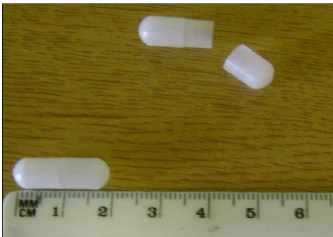
Figure 47: MRI marker pill made of polyoxymethelene. 2 half shells were glued together and hand filled with 0.4 ml 15 \mu M Gd-DOTA. The pill has the dimensions of 20 x 7 mm.
