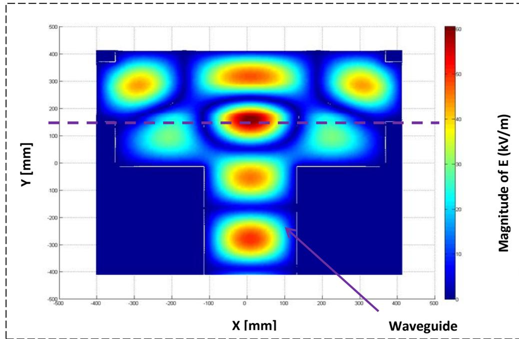
*Figure 5-20: The Electric field pattern in the 896 MHz vermiculite exfoliator system*
