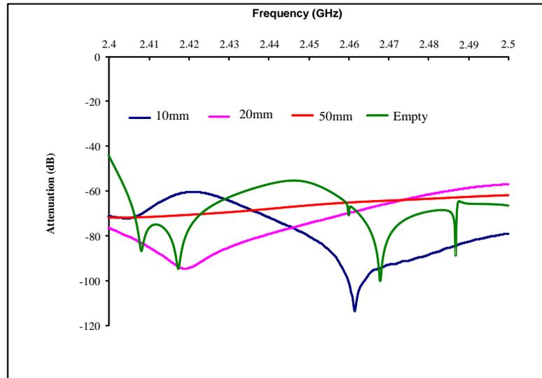
*Figure A-2: Attenuation characteristics versus frequency of the reflective choke, used in the present study. The plot shows the results generated during the design phase of the reflective choke both empty and filled with a material of complex permittivity  $\epsilon^* = 5 - j1$  at different bed heights.*
