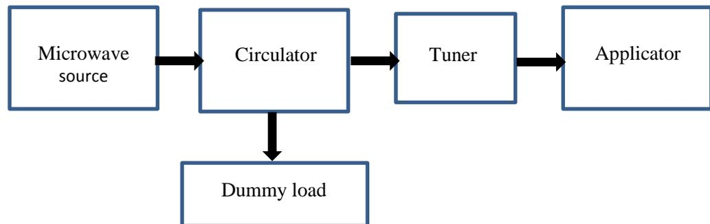
*Figure 3-13: Block diagram of microwave processing system*
