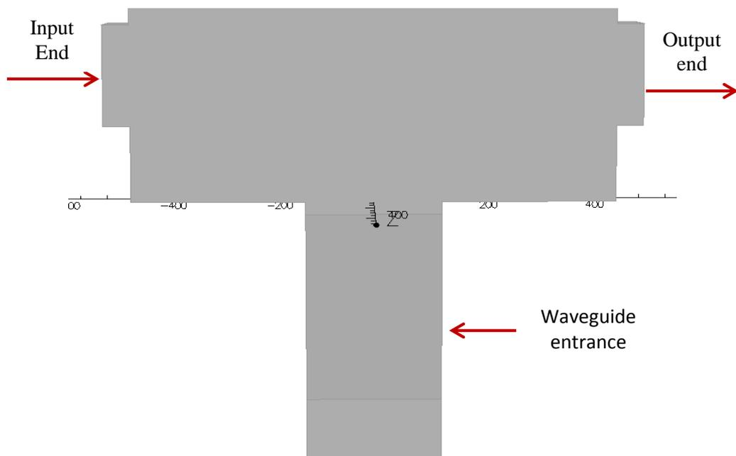
**Figure 5-19: Schematic of the internal structure of the cavity showing the input end, the output end and the connector end to the waveguide.**
