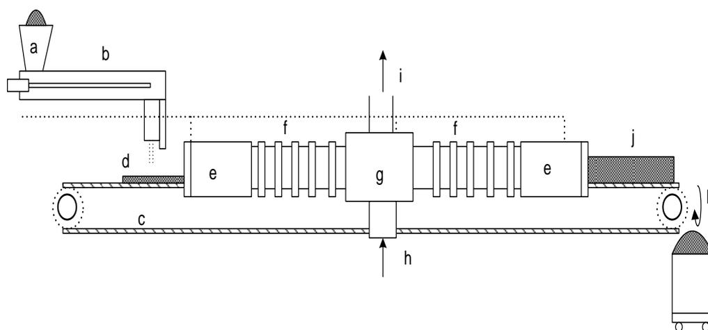
**Figure 5-6 : Industrial Microwave Vermiculite Exfoliation rig (2.45 GHz)**
