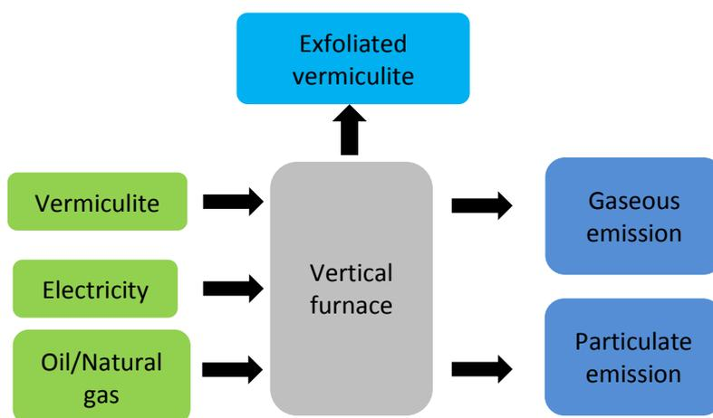
*Figure 6-4: Conventional exfoliation process diagram showing the material and energy input and the associated particulate and gaseous emissions*
