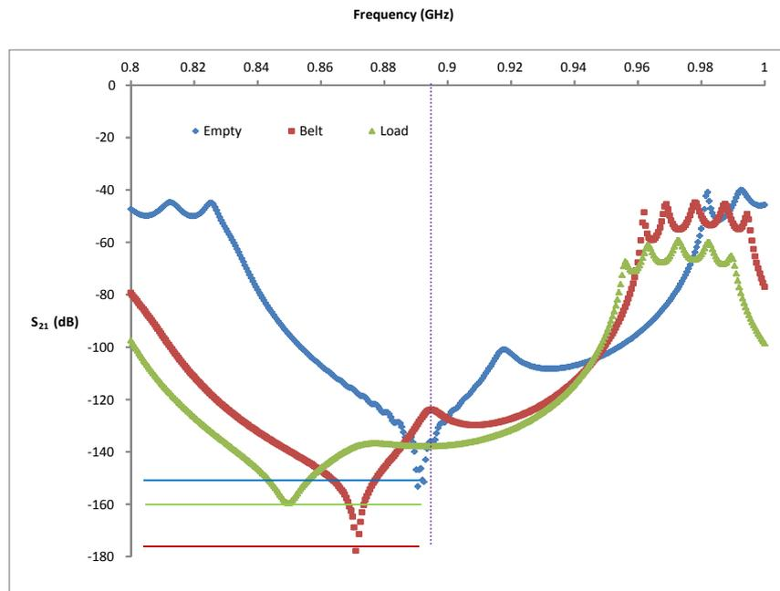
**Figure B-2:**  $S_{21}$  scattering parameters of the choke versus frequency for the three different types of possible operation, totally empty, with belt but unloaded and loaded with a 5mm deep bed of vermiculite.
