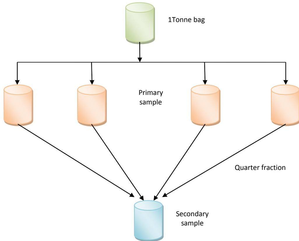
**Figure 4-4: Representative sample preparation using rotary sample divider**
