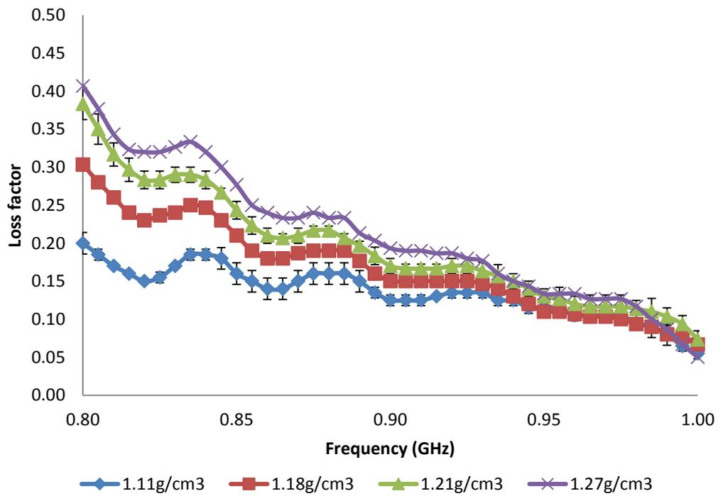
*Dielectric Properties of Australian Sample (superfine) as measured by waveguide technique*
