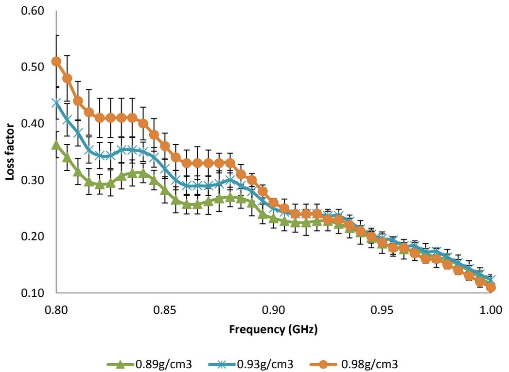
*Dielectric Properties of Chinese Sample (Medium) as measured by waveguide technique*
