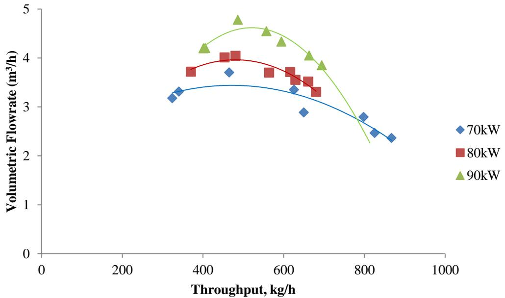
*Figure 5-26: Volumetric flowrate vs mass throughput for superfine grade of South African vermiculite using a continuous treatment system operating at 896 MHz*
