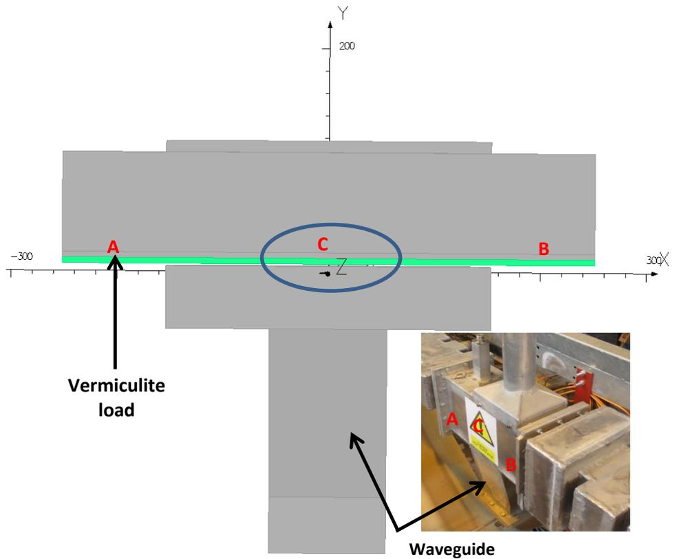
**Figure 5-5:** Microwave applicator with vermiculite load. An area marked 'A' and 'B' signifies the input and exit ends of the applicator respectively and they experience low power density. The area marked 'C' is at the centre of the applicator and this is the region of high power density.
