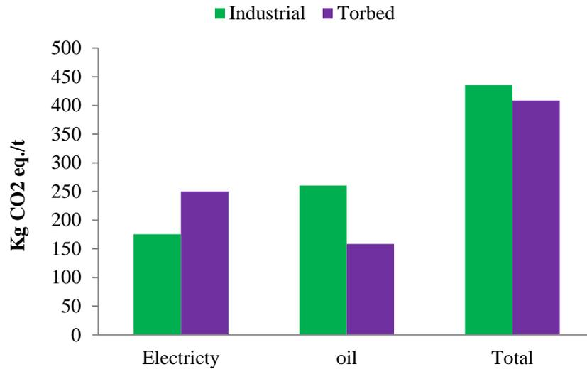
*Figure 6-10: Life cycle CO<sub>2</sub> emission contributed by electricity and oil in conventional thermal exfoliation*
