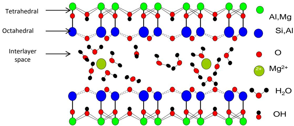
Figure 2-2: The vermiculite structural diagram. Adapted from (Reeves et al., 2006)
