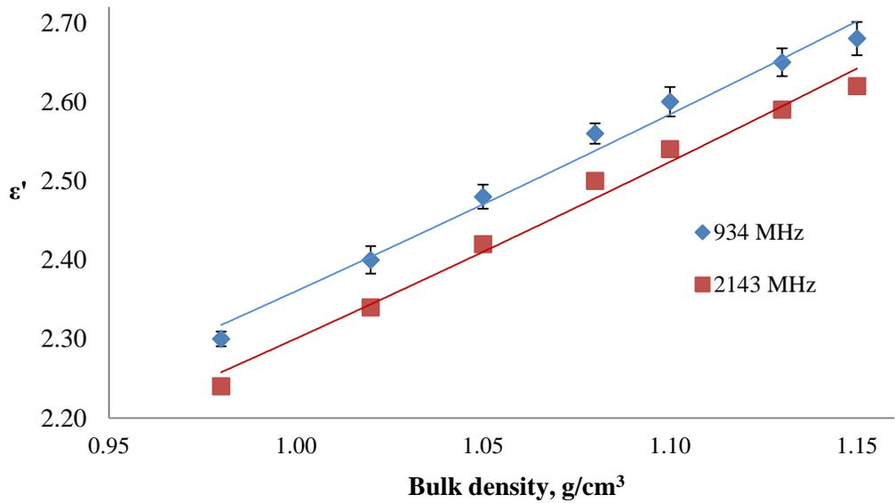
**Figure A:3-3:** Second order polynomial regression curve of dielectric constant (934 and 2143 MHz) of Australian sample against bulk density.
