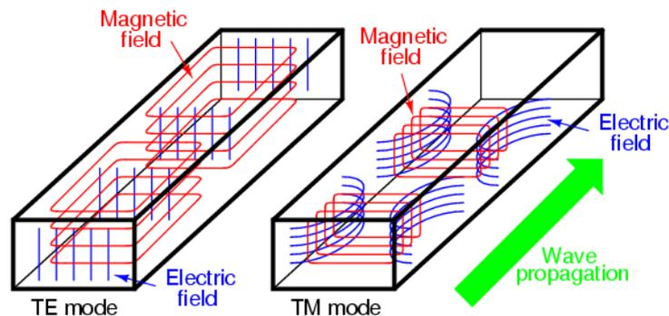
*Figure 3-15: Transverse electric (TE) and transverse magnetic (TM) waveguide*
