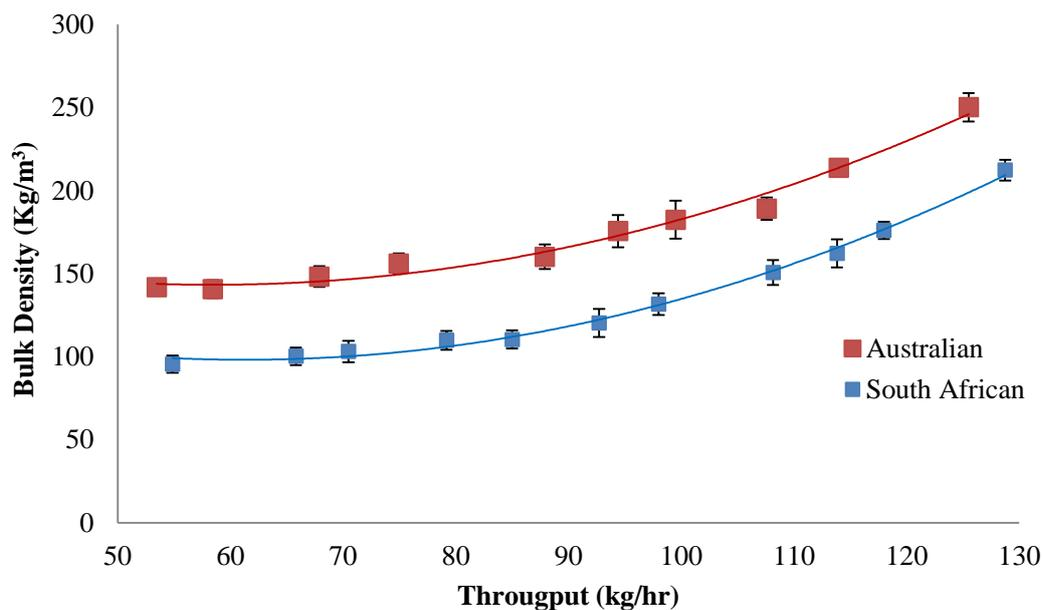
*Figure 5-7: Mean Performance (bulk density) vs throughput of pilot scale of vermiculite exfoliation system operating at 2.45 GH and 15 kW.*
