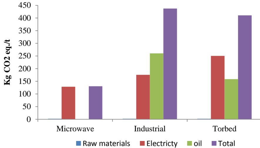
**Figure 6-8: Life cycle CO<sub>2</sub> emission for microwave and conventional thermal exfoliation using oil for furnace heating**
