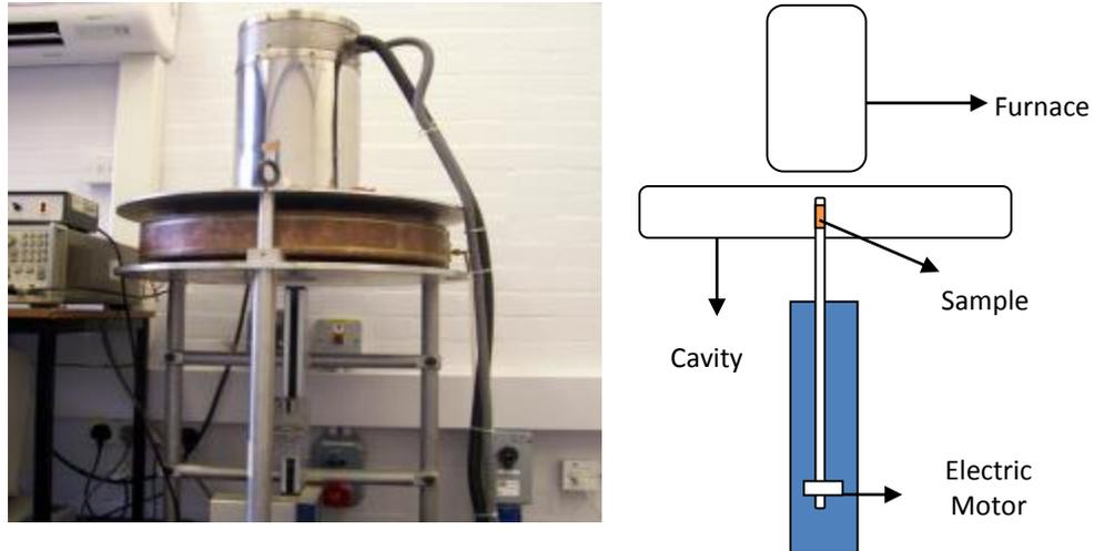
**Figure 4-18: Experimental set-up for cavity perturbation**
