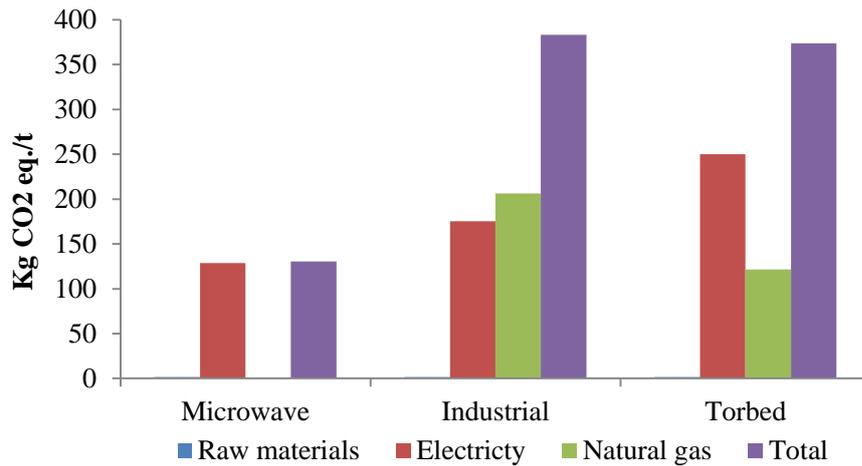
*Figure 6-7: Life cycle CO<sub>2</sub> emission for microwave and conventional thermal exfoliation using natural gas for furnace heating*
