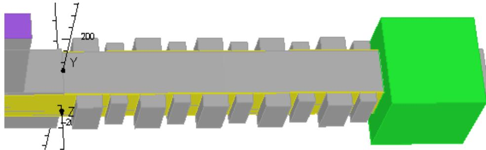
**Figure A-1: Detail of the choke used in the current study. The corrugated reflective choke is connected nearest to the applicator followed by the resistive choke (green colour). Note the author of this thesis did not design this**
