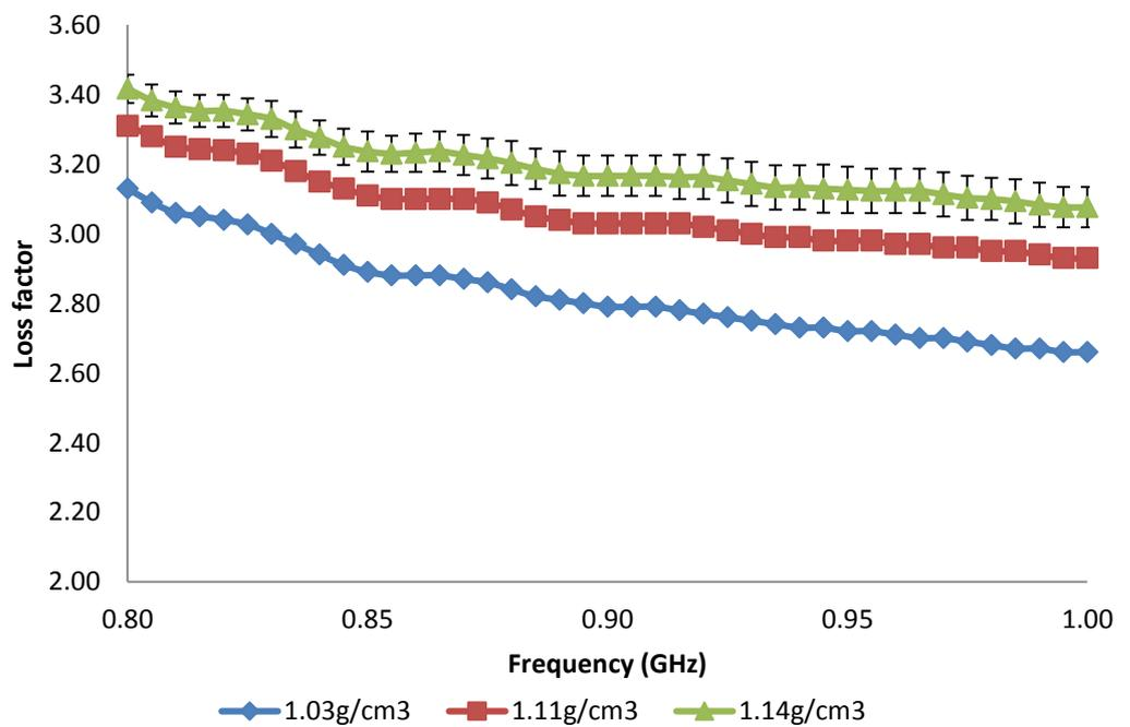
*Dielectric Properties of Brazilian Sample (Medium) as measured by waveguide technique*
