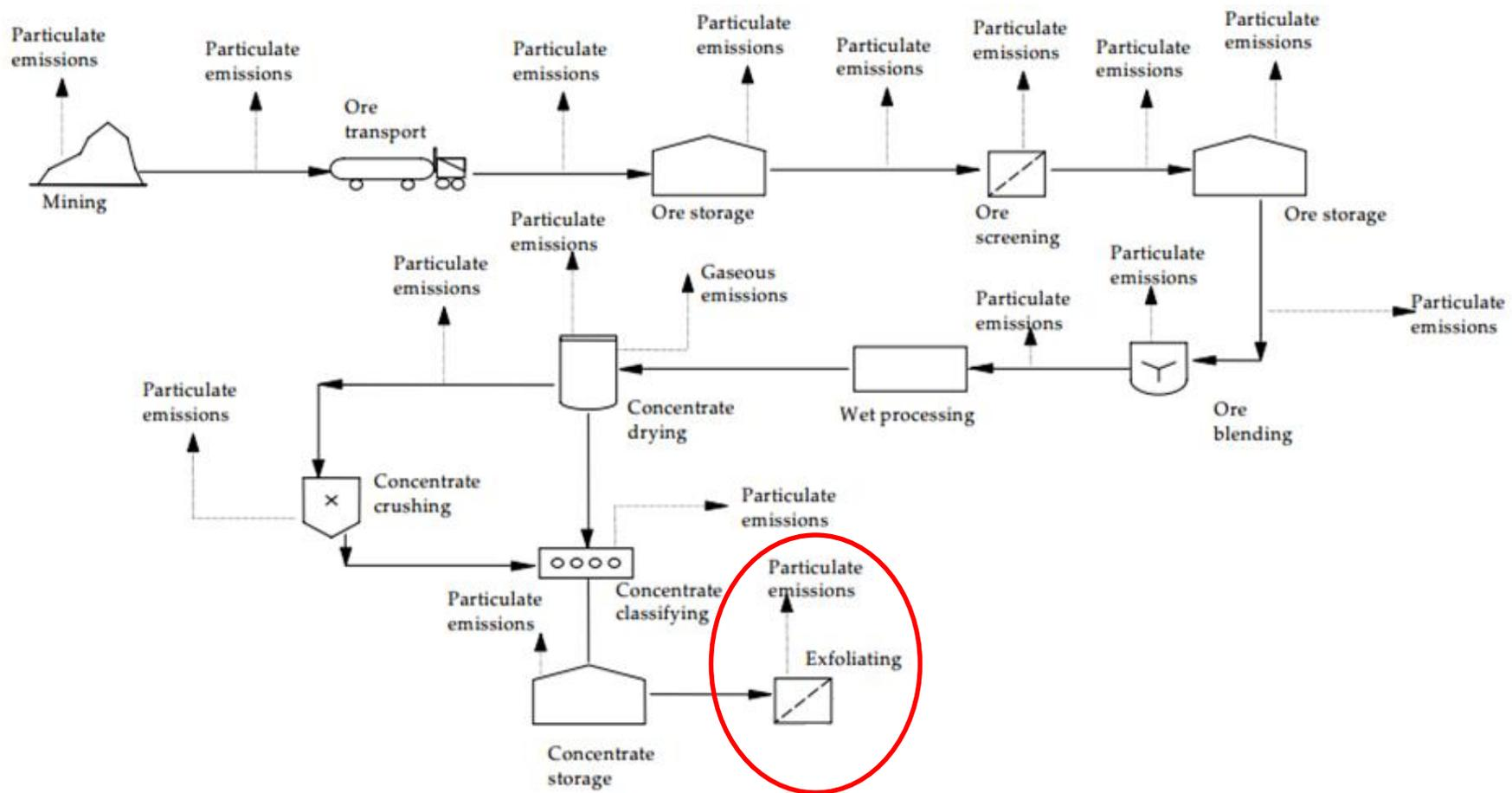
Figure 6-1: Process flowsheet for vermiculite processing from mining stage for storage of exfoliated product (NPI, 1999)
