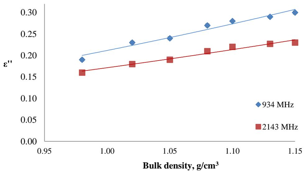
**Figure A:3-4:** Second order polynomial regression curve of loss factor (934 and 2143 MHz) of pulverised Australian sample against density
