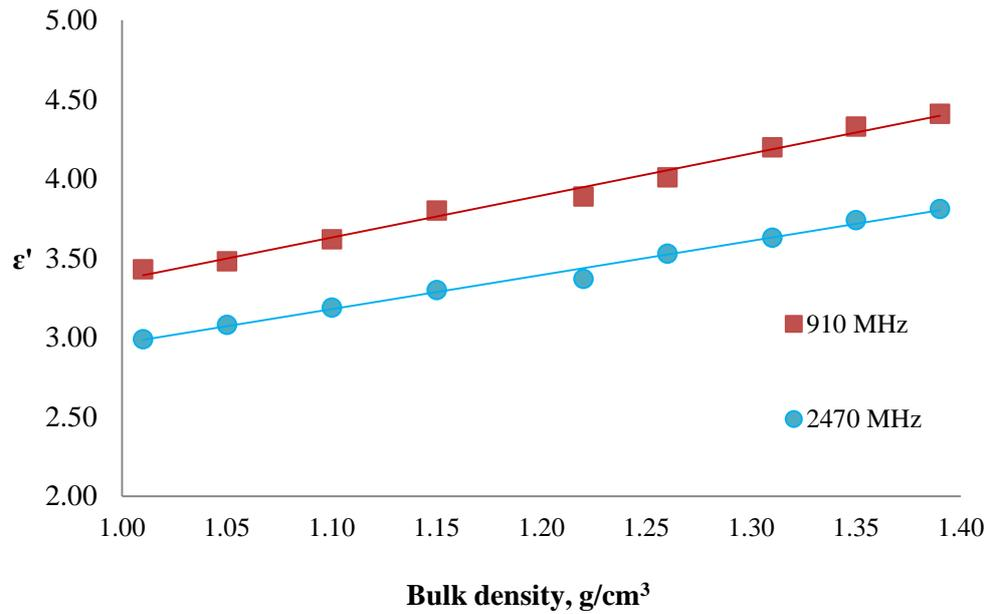
**Figure A:3-7: Second order polynomial regression curve of dielectric constant (910 and 2470 MHz) of pulverised Chinese sample against bulk density**
