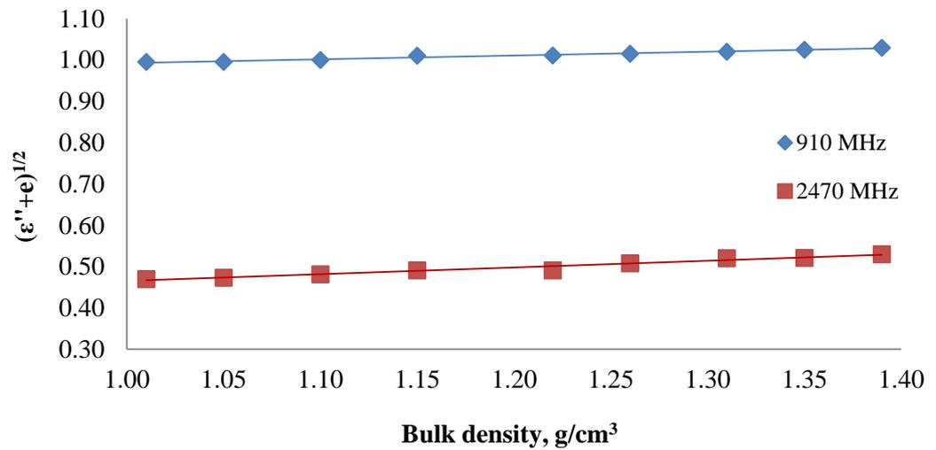
Figure A:3-24: Linear relationship between  $(\epsilon''+e)^{1/2}$  and density for Chinese sample
