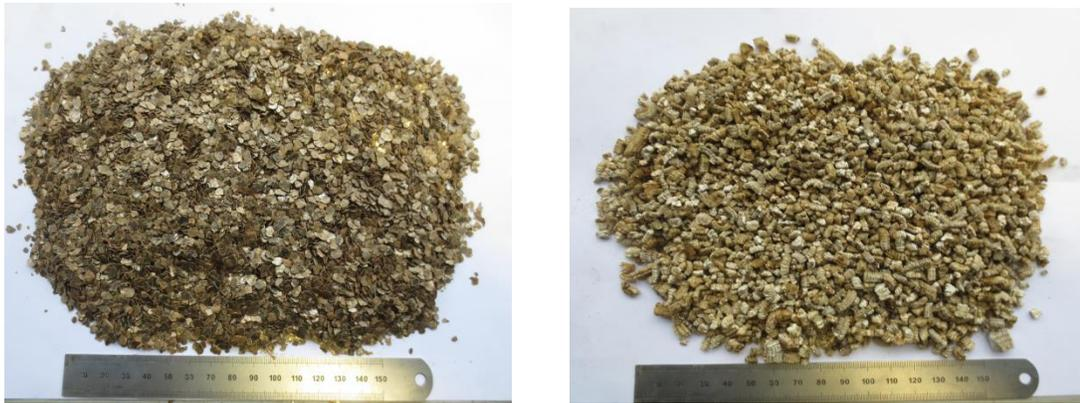
*Figure 2-1: The raw and exfoliated form of medium grade of Brazilian vermiculite*
