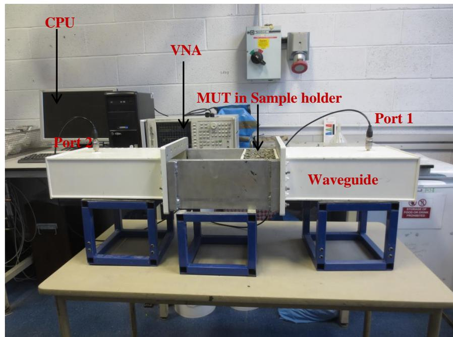
*Figure 4-33: Rectangular waveguide loaded with vermiculite bulk sample*
