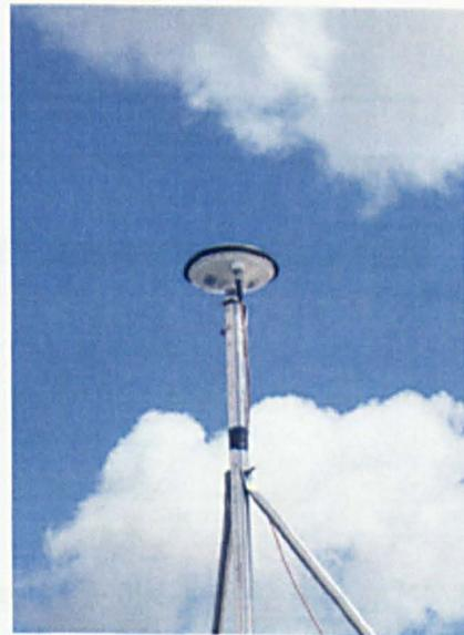
Figure 8.4: Placement of Novatel Pinwheel antenna for OEM4 receiver and POSRS system
