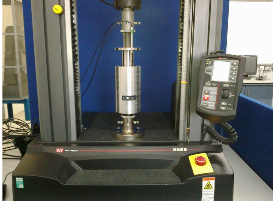
Fig. 3.1: Compaction testing rig.
