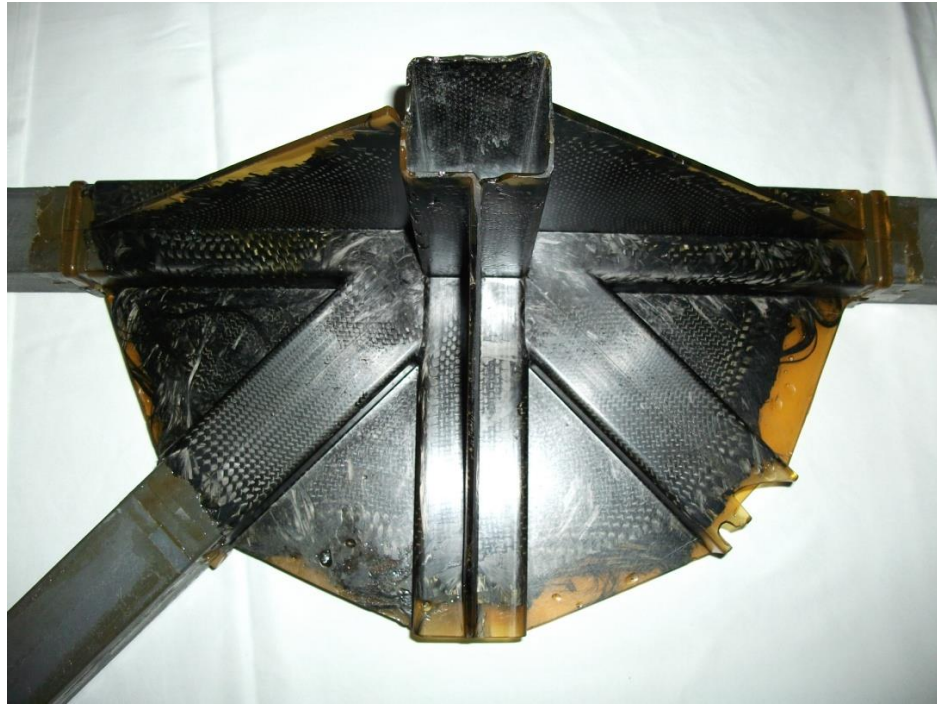
Fig. 9.3 (a): Prototype manufactured node top surface view.
