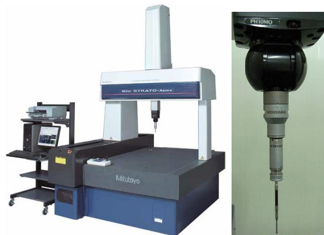
Fig. 3.11: Mitutoyo coordinate measuring machine, with scanning probe, (right).
