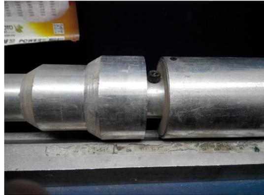
Figure 5.4: Photograph of (a) moling head connected to the body cover and (b) that of the bolted plate cover of the moling head connector.
