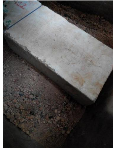
Figure 5.9: (a) The soil box that contains soil with a circular opening for entry of motion and (b) the concrete slab which acts as surcharge on the soil for the first 0.55 m after entry.
