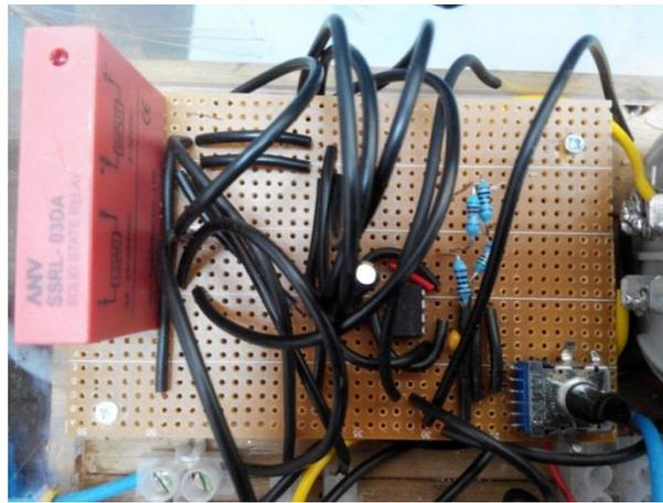
Figure 5.2: The circuit board LM555 the timer and potentiometer that manipulates the operating frequency of AC power supply.
