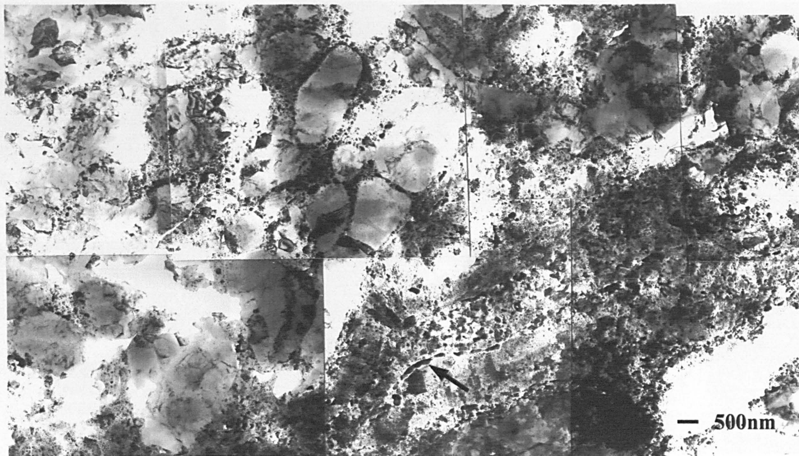
Figure 7.8 TEM montage of the as-sprayed Al 2 O 3 Sn 3 Si coating
