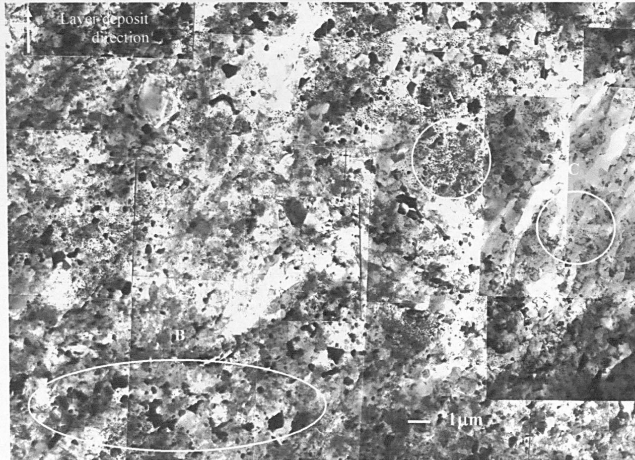
Figure 4.21 TEM montage of HVOLF as-sprayed coating
