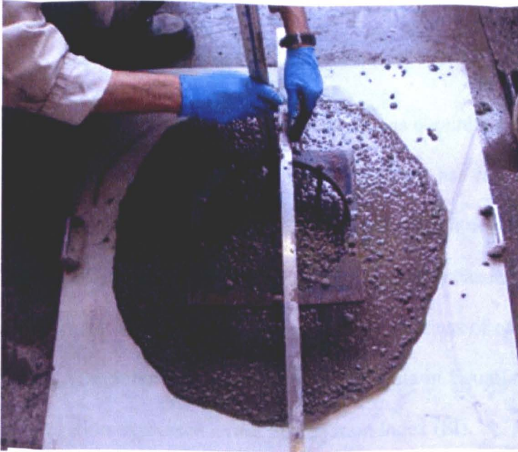
Figure 4.11 The measurement of J-Ring flow and blocking step of SCC
