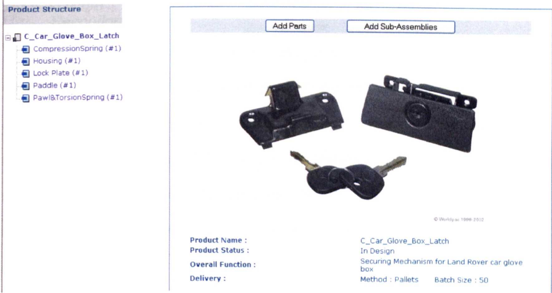
FIGURE 7-26: C CAR LATCH WITH INHERITED PRODUCT STRUCTURE
