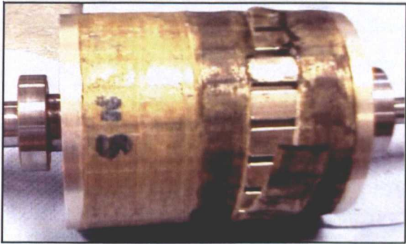
Figure 5-9: The PMSM's rotor and the damaged sleeve
