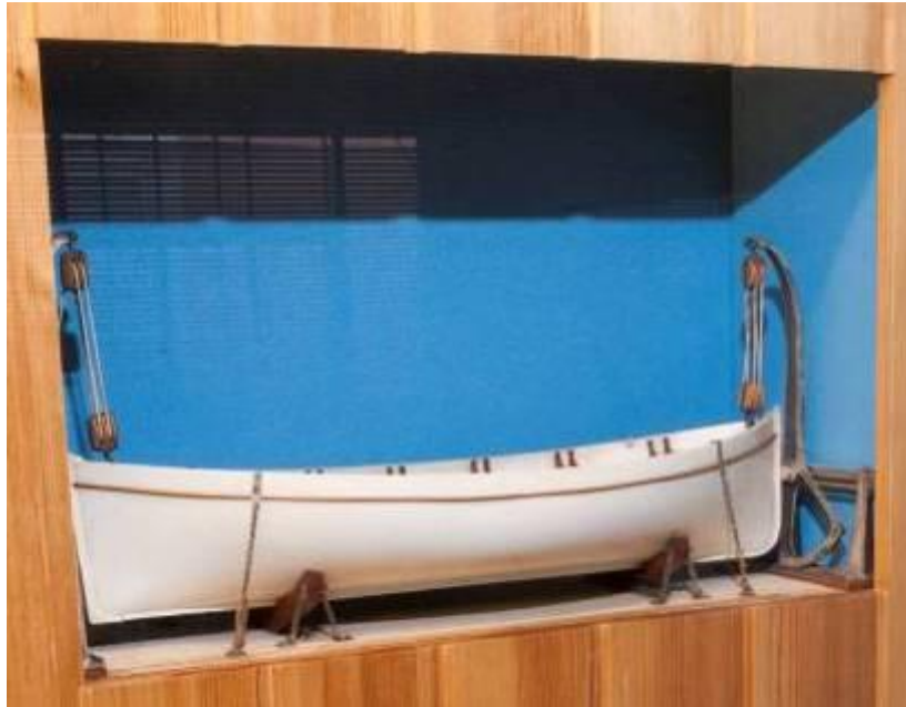
Figure 40 A photograph of the Ship's Lifeboat model showing the 'quadrant' type davits patented by the Swedish inventor Axel Welin. The model was presented to the museum by Welin in 1905. (Inventory No.: 1905-107). Scale 1:16. (© Science Museum / SSPL).
