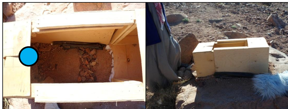
Figure 20: Apparatus used for recording rampart sounds shown from the top (left) and the side. Circle indicates the position of the microphone during recording.
