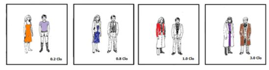
Figure 3.2: Insulation values of different kind of clothing (1 Clo =0.155 m<sup>2</sup>K/W) \_ reproduced after Fanger P. O., 1985 as a source.
