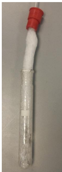
Figure 5-19: Polymer foam formed when carrying out 30 cm 3 non-CCT controlled MMA polymerisation within CEM Discover at 100 °C
