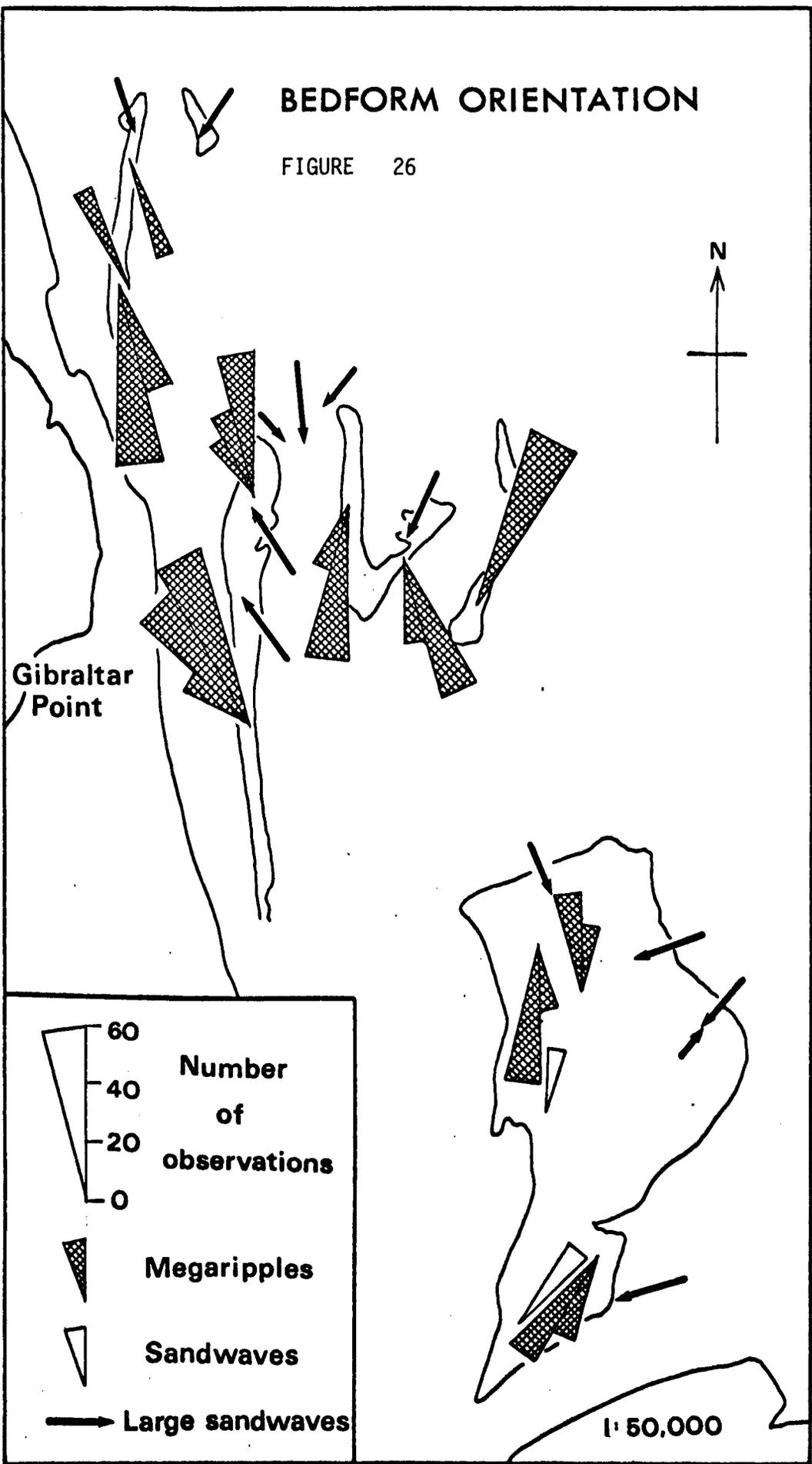
cones are at the location of the grid systems deployed for orientation measurement. Large sandwaves were measured individually and their orientations are shown by arrows on the map.
