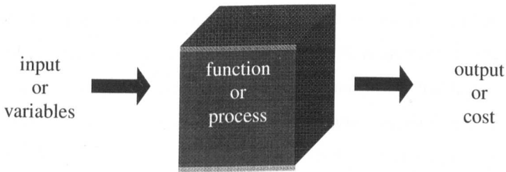
Figure 3.1: Diagram of a function or process that is to be optimised. Optimisation varies the input to achieve a desired output.
