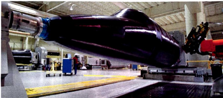
**Fig 1-13** Typical automated tape winding process [41]
