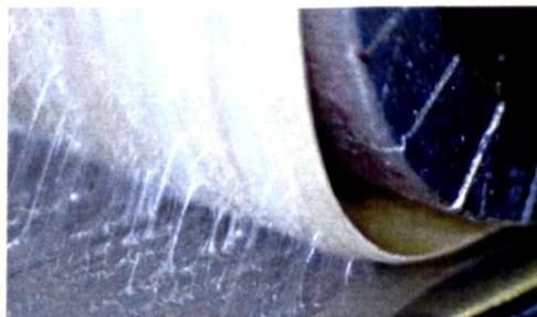
**Fig 3-14** Deviation in bending radius from the roller radius during high tack peel
