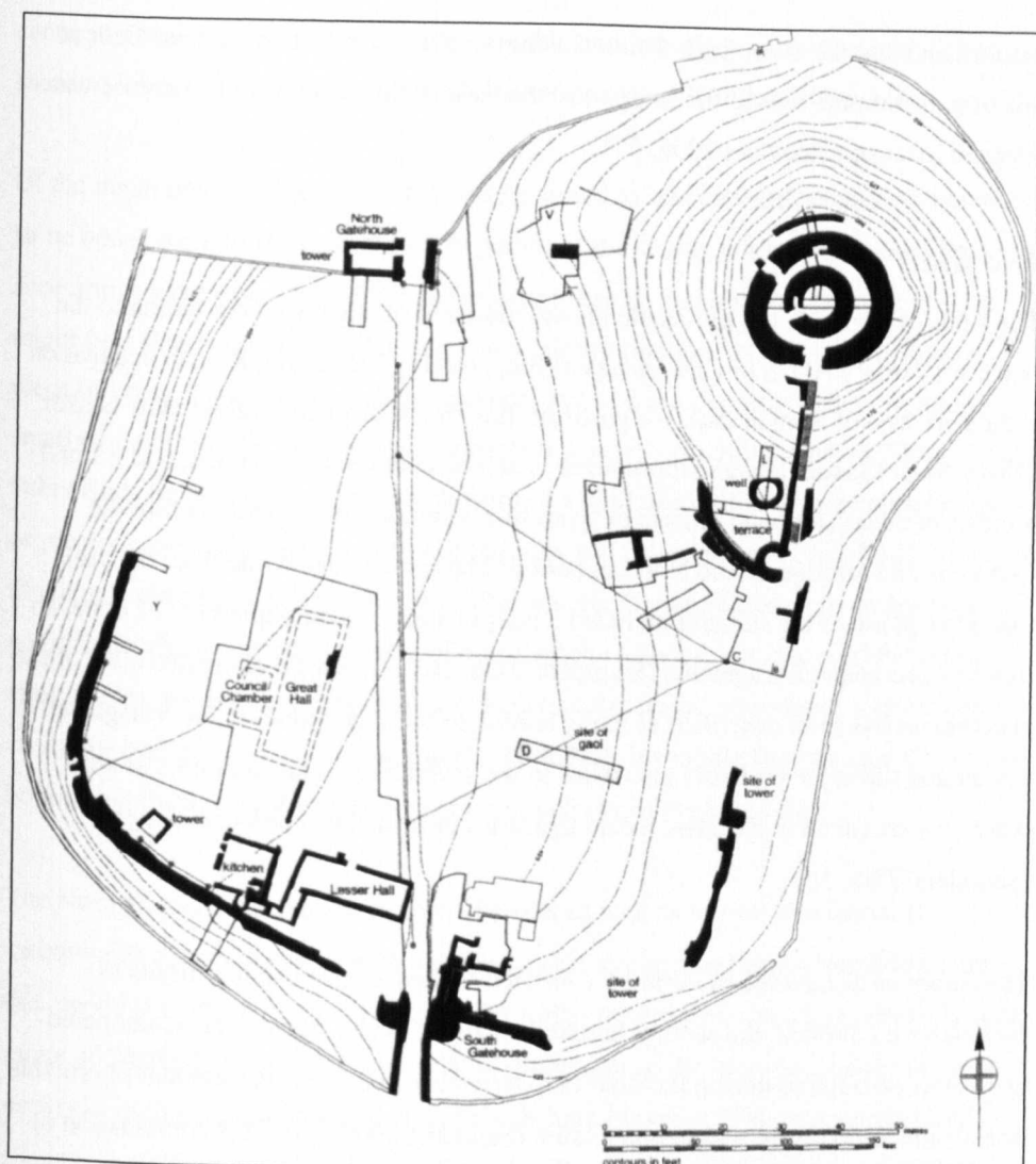
Figure 207 - Contour plan of Launceston Castle, showing the standing remains and excavated areas, including survey lines (Saunders 2006, Figure 4.2, 53)
