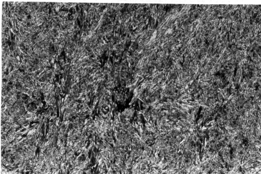
Plate 88 Teruggite crystals appearing very small and needle-shaped in the thin section. Crossed nicols, x10.
