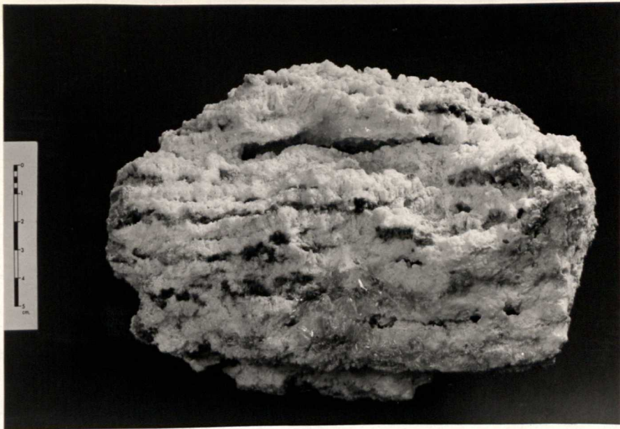
Plate 64 Calcite, alteration product of colemanite, and colemanite crystals in the middle showing the relationships between colemanite and its alteration product, Espey mine.
