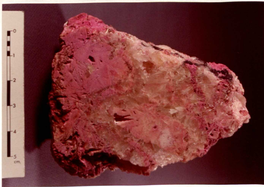
Plate 65 Polished, etched and stained colemanite showing alteration to calcite, which has a pink colour after the staining.
