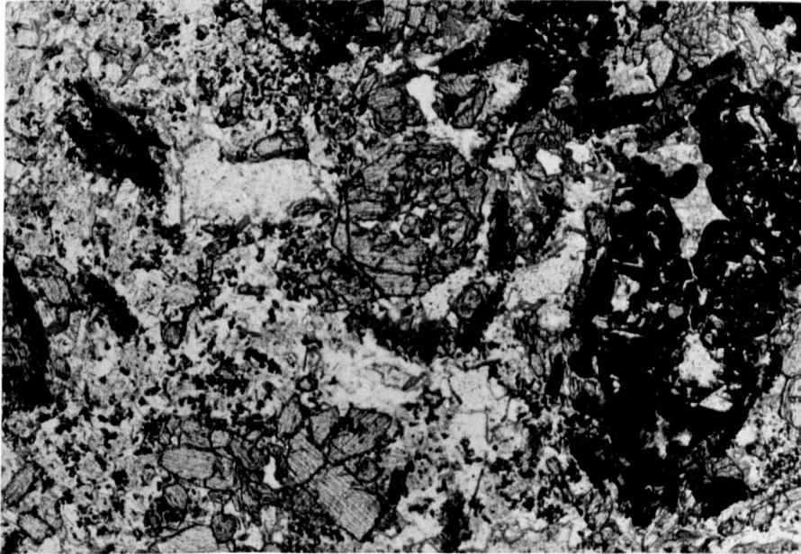
Plate 9. Olivine-augite basalt or andesitic basalt showing phenocrysts of olivine, augite, biotite and porphyritic groundmass. Plane polarized light, x10.
