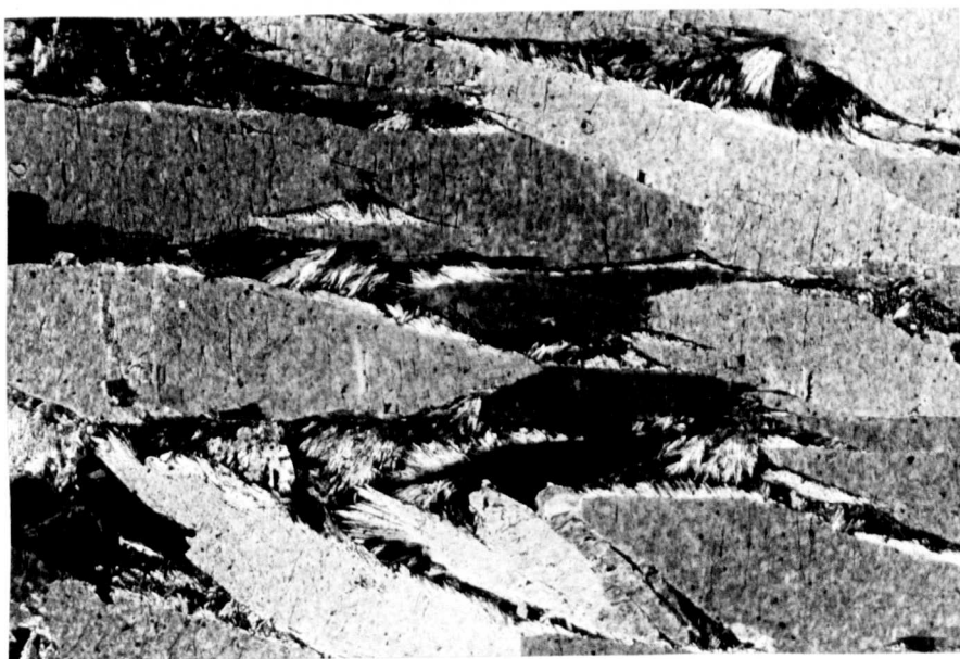
Plate 57 Prismatic colemanite crystals and fibrous crystals growing at their edges. Crossed nicols, x10.
