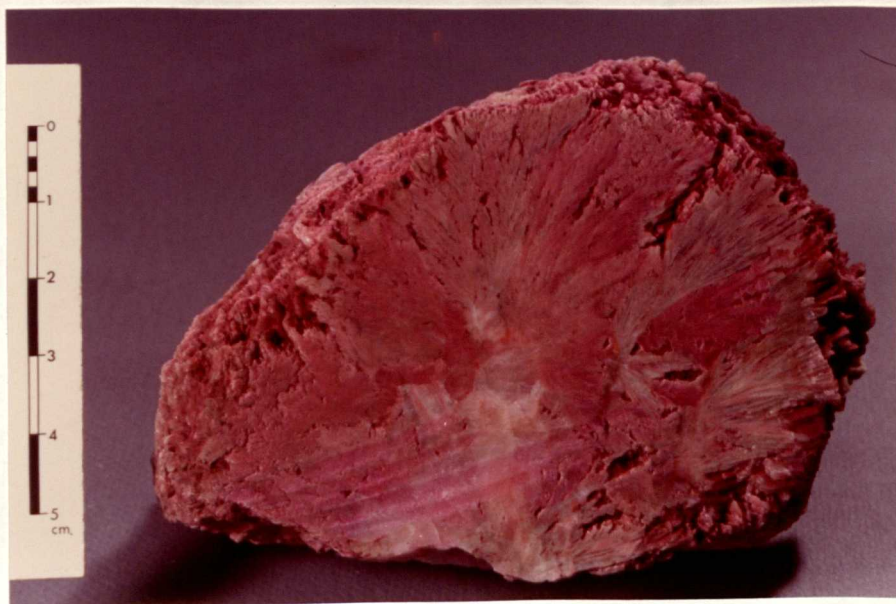
Plate 66 Polished, etched and stained colemanite nodule showing alteration to calcite mainly along the radiating structure.
