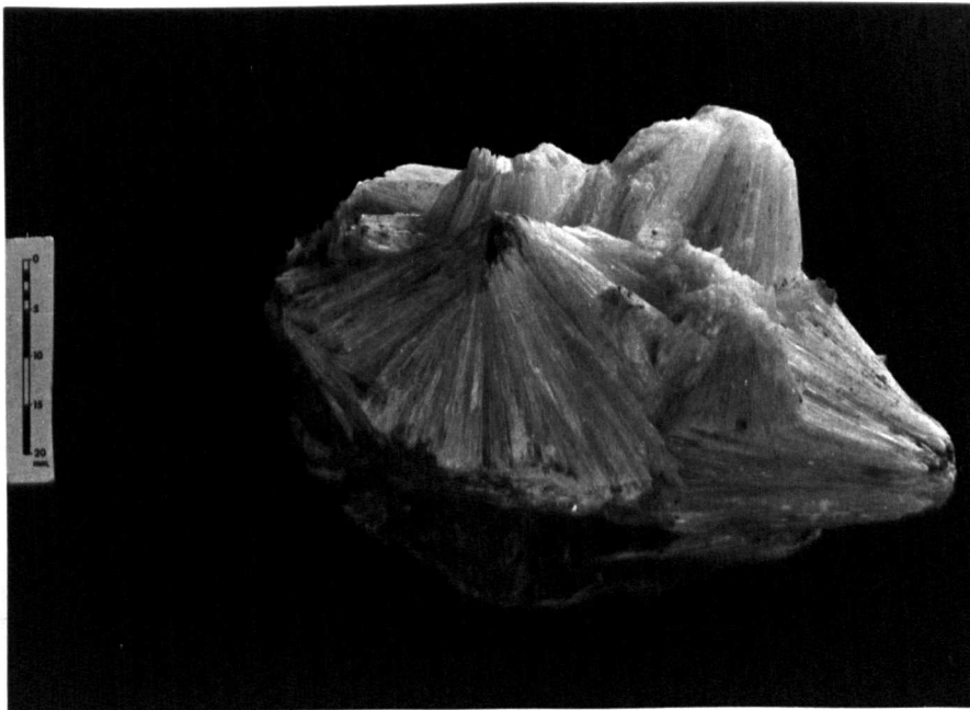
Plate 81 Radiating crystals of hydroboracite intersecting with each other and groups of them showing a conical appearance, Killik locality.
