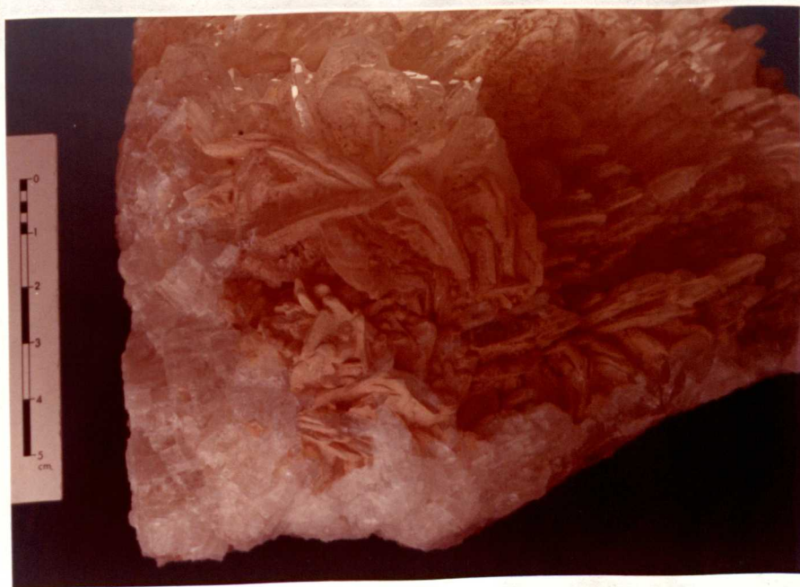
Plate 61 Plate showing cahnite coating on euhedral colemanite crystals, Espey mine.
