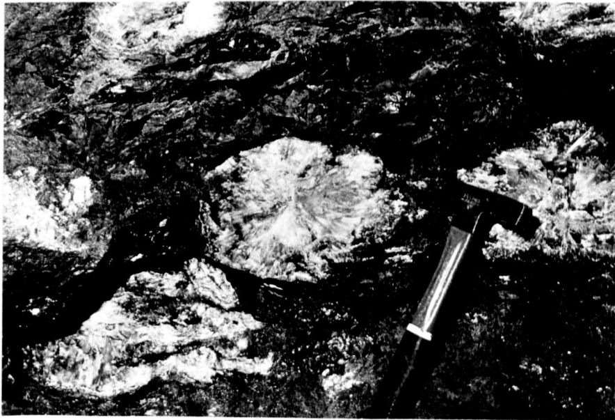
Plate 31 Colemanite nodules in the borate zone showing a radiating structure, surrounded by clays, Killik underground mine.
