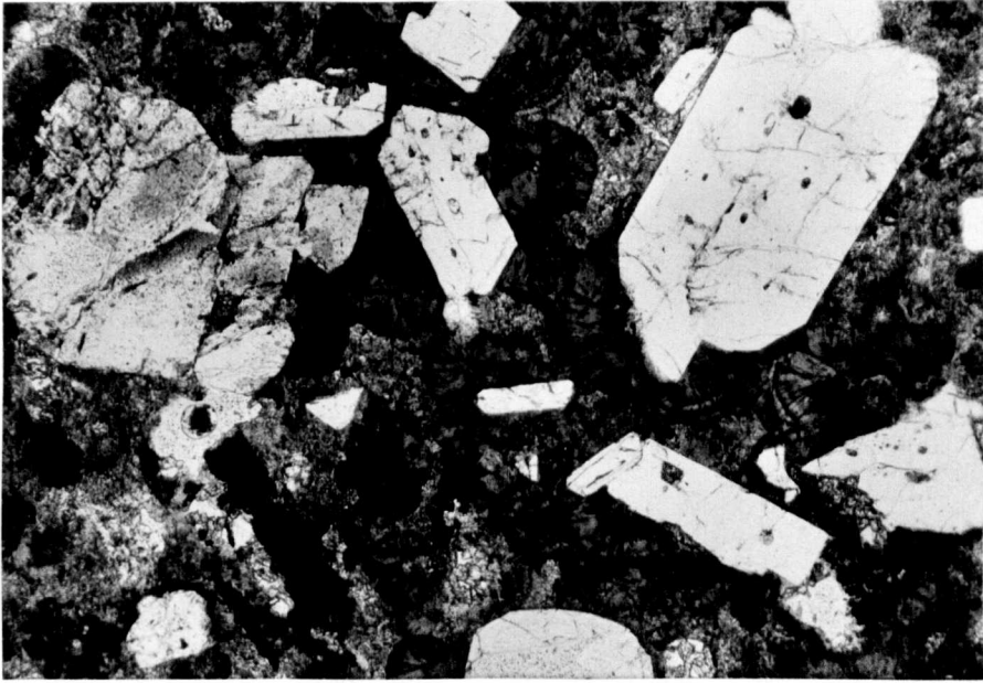
Plate 5. Plate showing spherulitic rhyolite containing phenocrysts of quartz, feldspar, biotite and a microfelsitic and spherulitic groundmass. Plane polarized light, x10.
