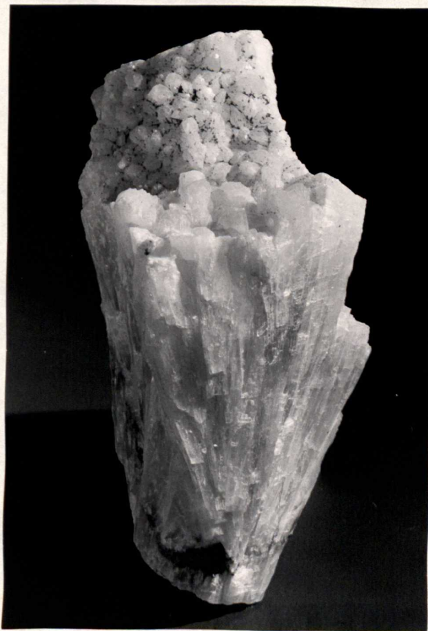
Plate 33 Massive granular colemanite with radial structure. Subeuhedral to euhedral crystals at the upper end. Sample used as standard, Sarikaya opencast mine.
