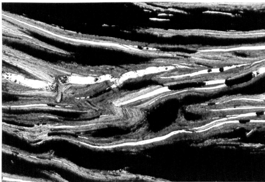
Plate 73 Ulexite and clay mixture showing very thin veins, occasionally filled by calcite crystals. Plane polarized light, x10.
