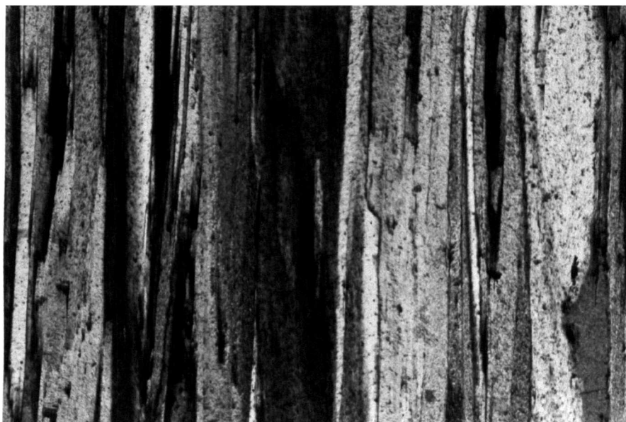
Plate 102 Fibrous gypsum with basal pinacoidal cleavage. Crossed nicols, x10.
