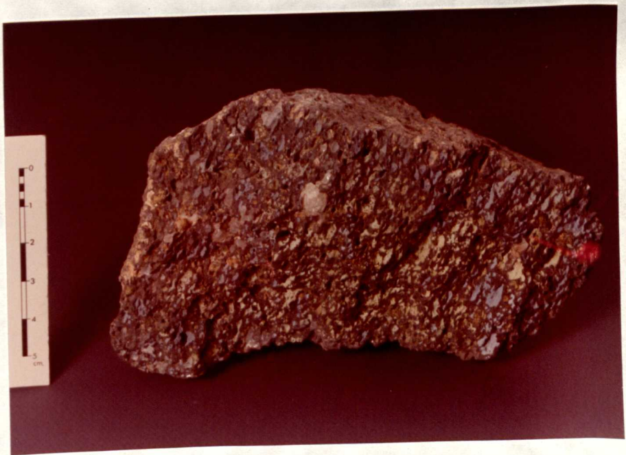
Plate 7. Hand specimen of pyroxene andesite showing calcite as amygdule-fillings, phenocrysts of feldspar and biotite, pyrite. Due to alteration it shows a greyish yellow and blue colouring.
