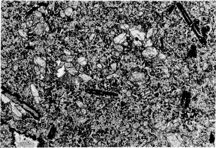
Plate 8. Plate showing pyroxene andesite containing phenocrysts of pyroxene, plagioclase, biotite, and porphyritic groundmass. Plane polarized light, x10.
