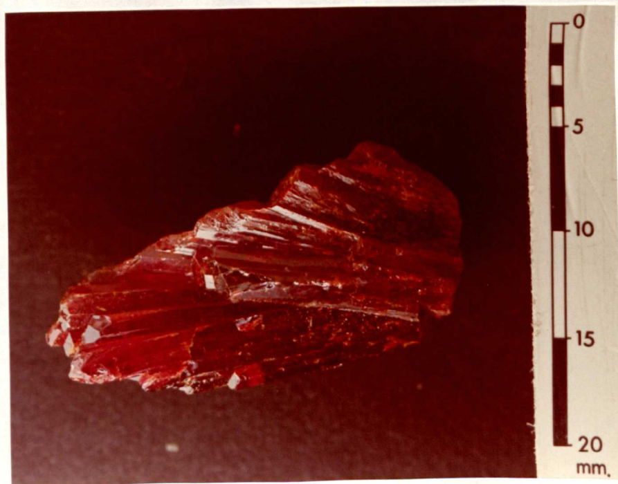
Plate 93 Plate showing realgar crystals exceeding 2cm in length, Sarikaya locality.
