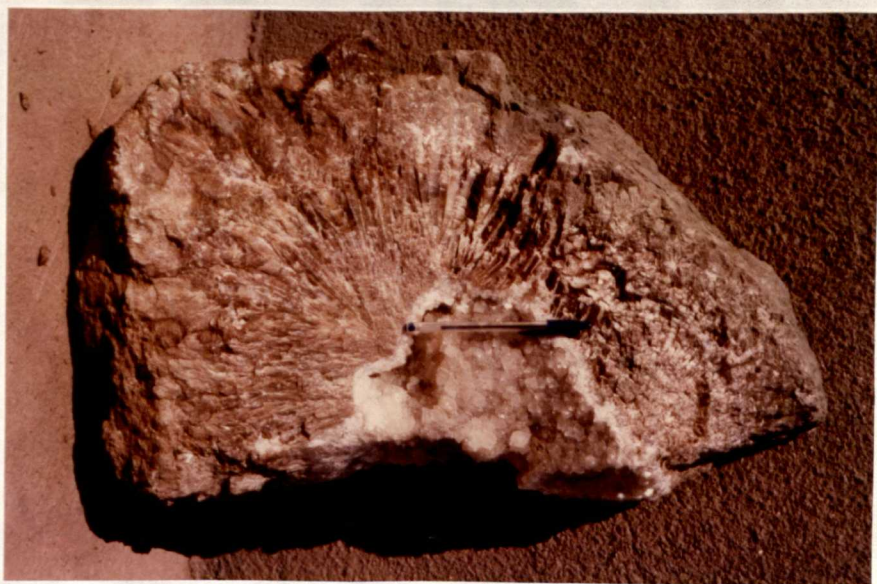
Plate 32 Section of colemanite nodule showing radiating structure with clay injection in between colemanite crystals, vugh in the centre filled with euhedral colemanite crystals and clay covering the outer edge of the nodule, Killik underground mine.
