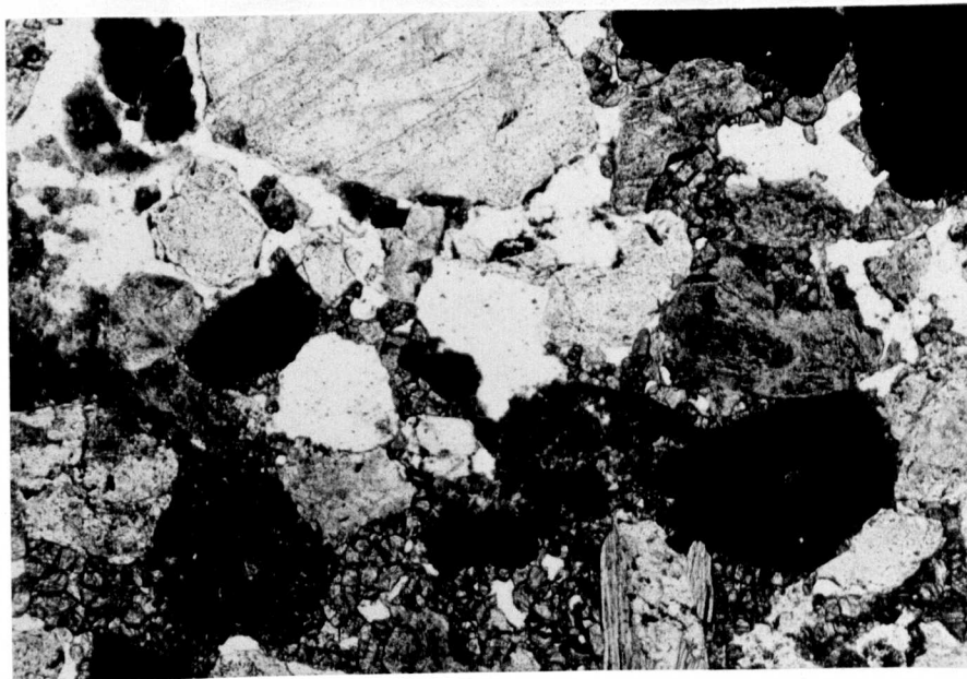
Plate 14. Conglomerate containing grains of quartz, plagioclase, mica and metamorphic rock fragments, with calcite cement. Plane polarized light, x10.
