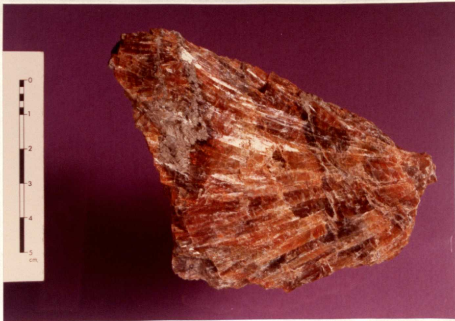
Plate 94 Colemanite showing a bright orange to red colour, which includes realgar and orpiment, Killik locality.
