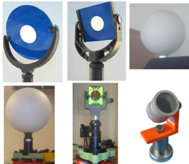
Figure 5-2: The HDS and sphere targets used in the field trial. Top left: 6" circular blue and white middle. Top middle: 3"x3" square blue and white. Top right: small sphere 145 mm dia., lower left: large sphere 200 mm dia., lower middle and right: mini prism for large and small sphere respectively.
