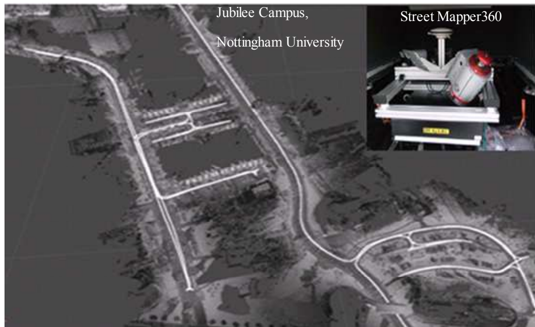
Figure 3-20: StreetMapper360, data collected in test area (Jubilee campus) overlain vehicle trajectory. Point shade represents the strength of the returned laser pulse. Right corner: MLS contains (Riegl VQ-250, IMU and GPS antenna).
