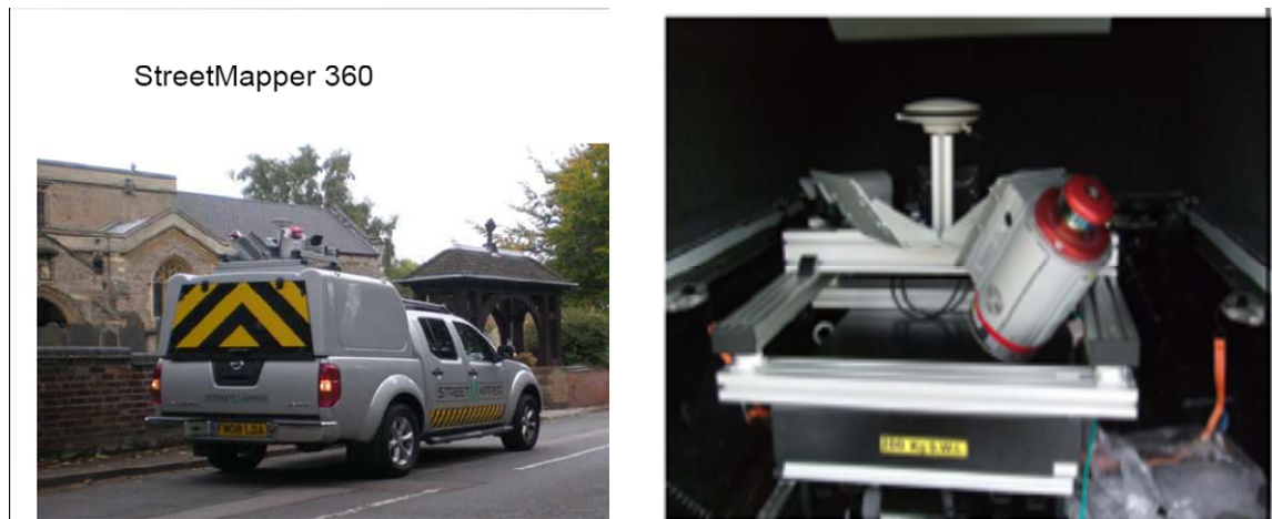
Figure 2-3: StreetMapper360 with Riegl VQ-250 (left) and the system inside the vehicle with fixed frame (right) (source (Streetmapper360, 2009).
