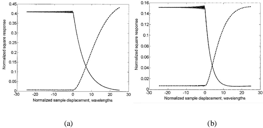
Fig. 2-25 Surface wave response across an interface on and off resonance (a) 'weak' coupling; (b) strong coupling
