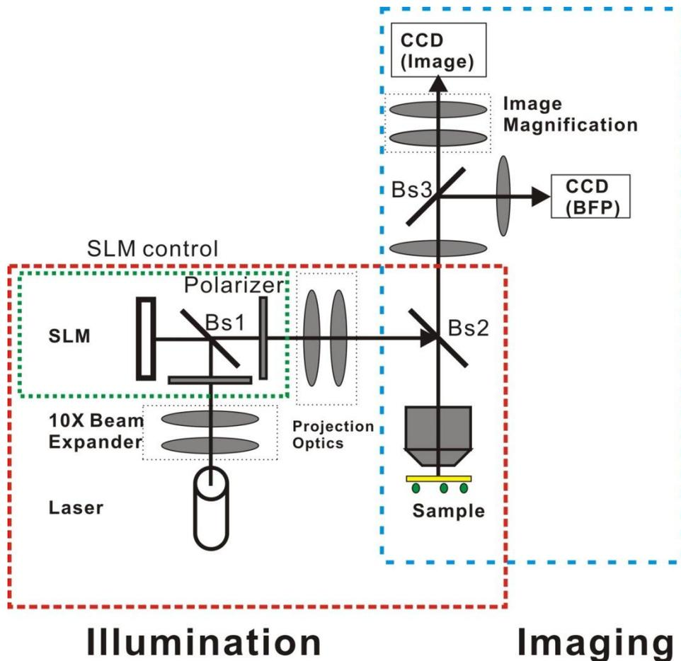
Fig. 3-2 Schematic diagram of the experiment setup
