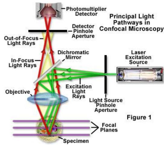
Fig. 2-30 the mechanics of confocal microscopy from Nikon Microscopy
