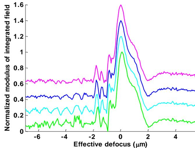
Fig. 5-16 The effect of SLM misalignment on the quality of the  $V(\alpha)$  curves. The SLM was misaligned by -0.01, 0, 0.01, 0.02 units of the back focal plane aperture from the lower green line to the upper magenta line. The curves are displaced along the y-axis by 0.2 units for clarity.
