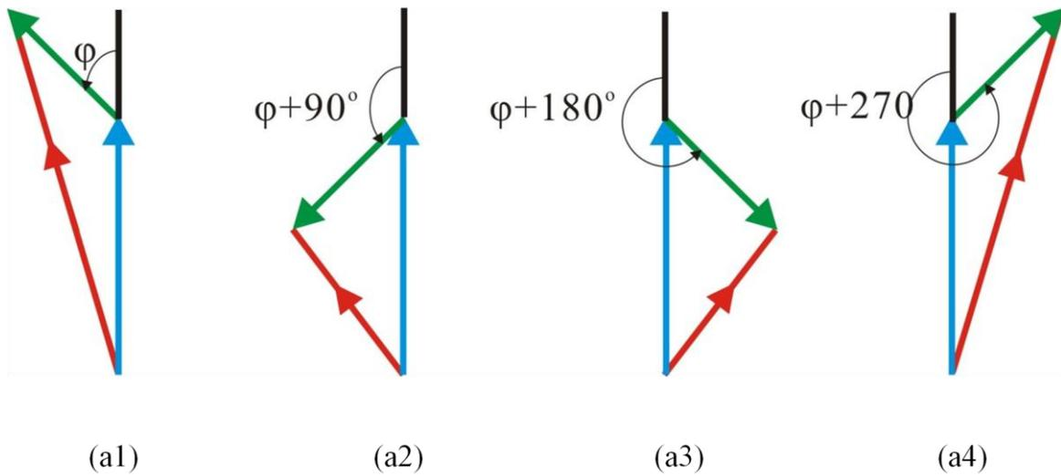
Fig. 6-3 Effect of phase stepping on relative phase of reference and plasmon beams, green line is the reference signal R, blue line is the SP, red line is the resultant signal V. a1, a2, a3, a4 shows the four steps vectors;
