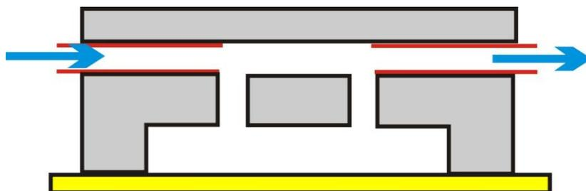
Fig. 7-2 Schematic diagram of the designed flow cell
