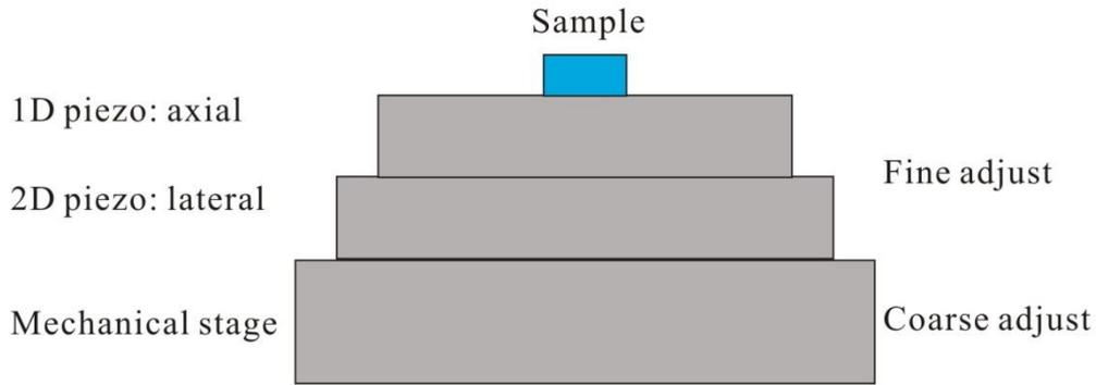
Fig. 3-10 Schematic diagram of the sample scanning system
