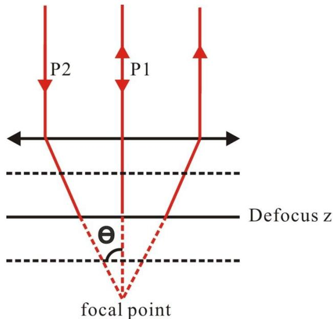
Fig. 5-2 basic idea of defocus  $z$  scanning
