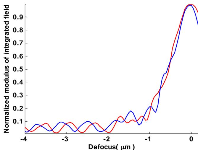
Fig. 5-15  $V(\alpha)$  curves obtained with two different phase shifts of the reference, red curve refers to the non-phase shifting case and the blue line refers to the case with shifting  $90^\circ$  on the reference beam;
