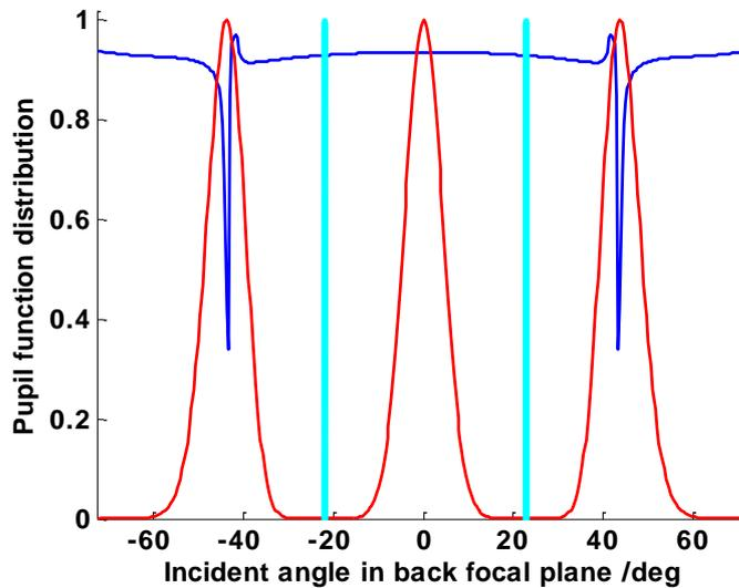
Fig. 6-2 Pupil function distribution (red curve) and calculated reflection coefficient for p-incident polarization on an uncoated sample (blue curve); the vertical cyan lines represent the range of angles over which the phase stepping of the reference beam was imposed.
