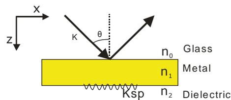
Fig. 2-7 three layer sandwiched sample structure
