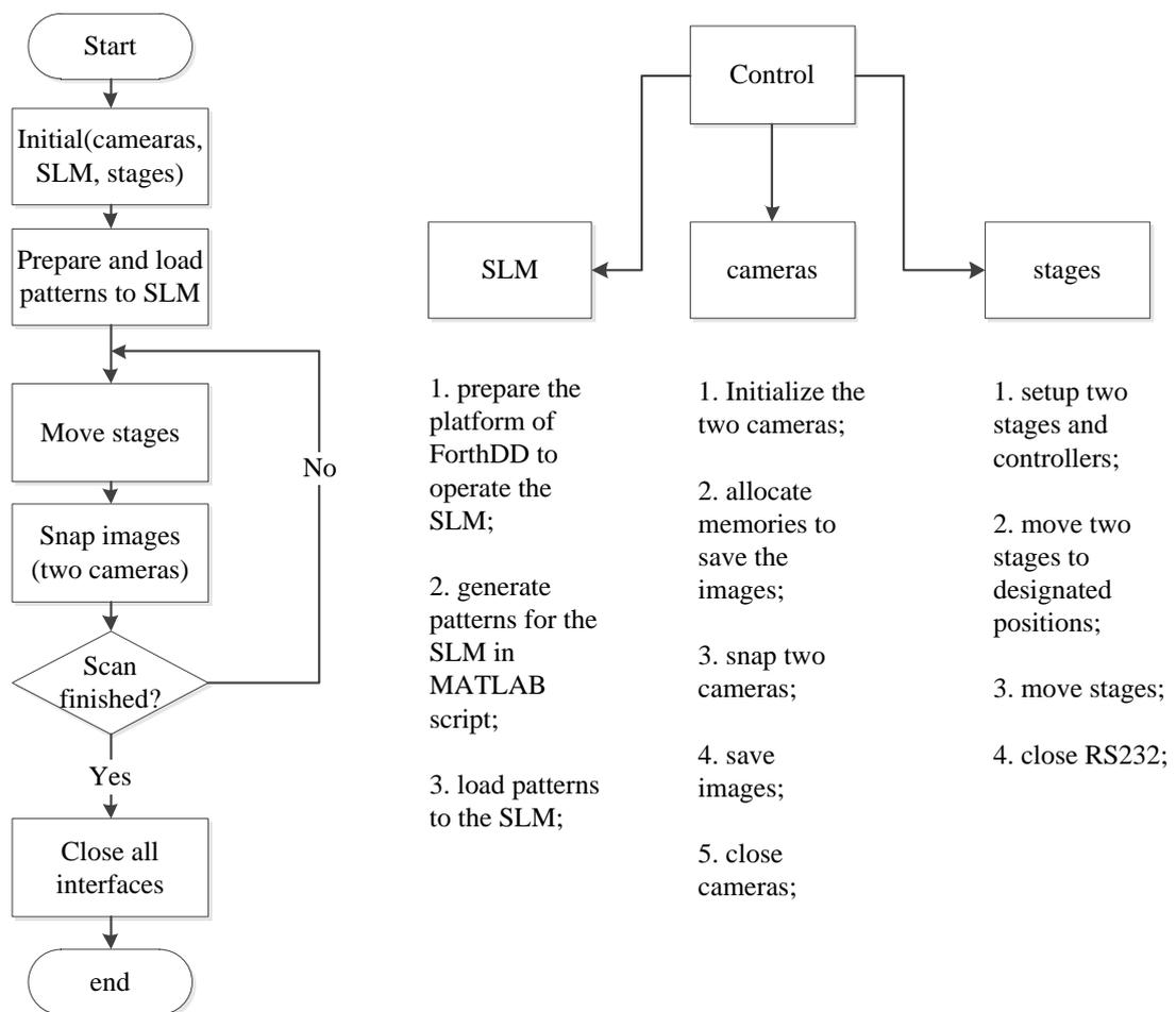
Fig. 3-14 Flowchart of the controlling software
