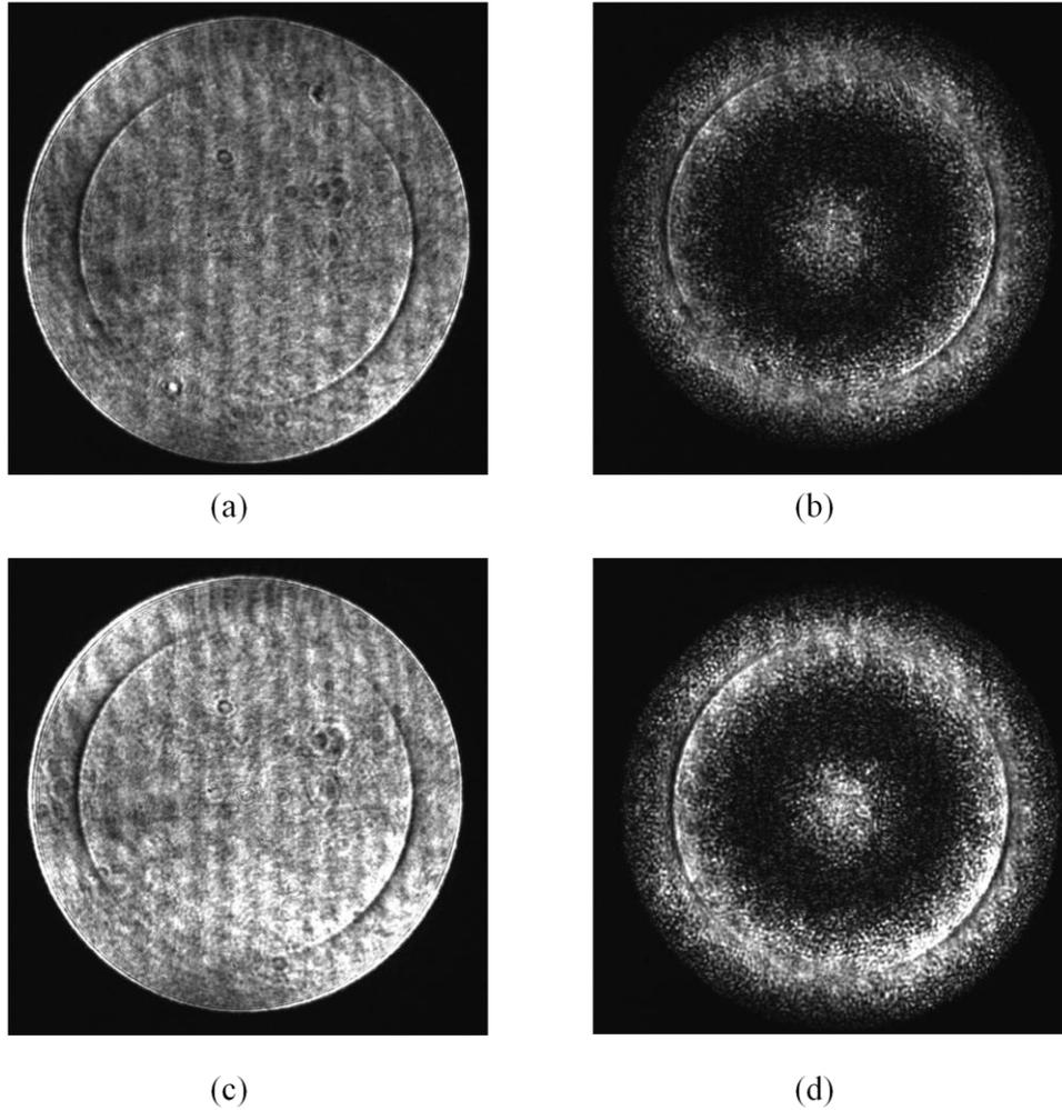
Fig. 5-10 Back focal plane (BFP) images using a phase SLM to effectively modulate the amplitude; (a) is the un-modulated BFP image when using uncoated gold; (b) is the modulated BFP image when using uncoated gold; (c) is the un-modulated BFP image when using 10nm ITO coated gold; (d) is the modulated BFP image when using 10nm ITO coated gold.
