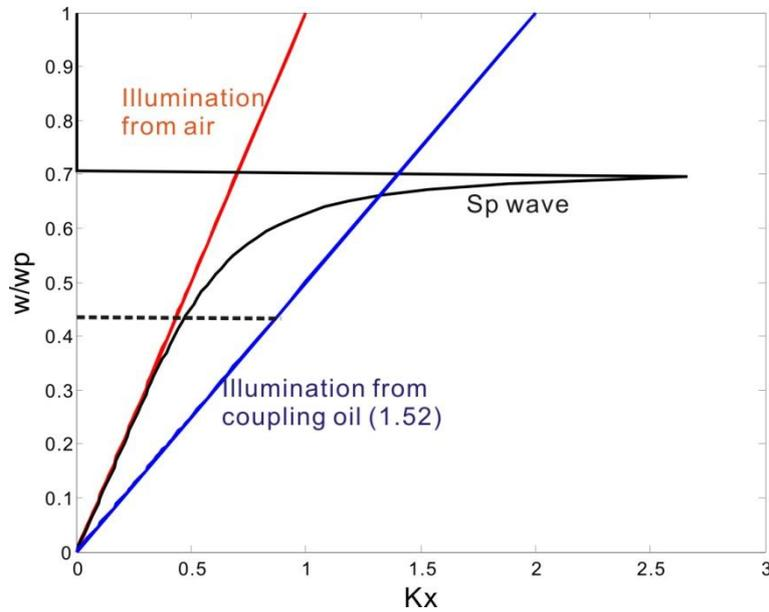
Fig. 2-3 Dispersion relations of electromagnetic waves; the red line, blue line and black curve describe the light dispersion in air, glass and the SPR non-linear dispersion relation when using metal/air.
