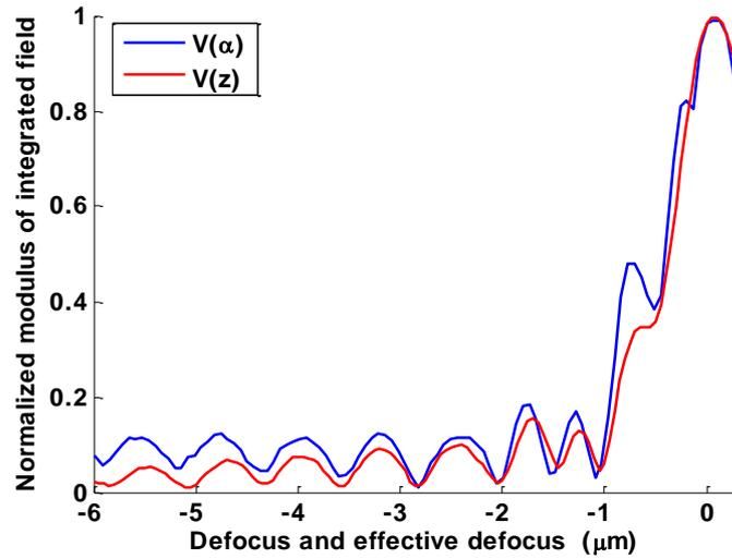
Fig. 5-12 Comparison between  $V(z)$  and  $V(z_{eff})$ , the red line refers to the real  $V(z)$  curve and blue line refers to the effective  $V(z)$  calculated from  $V(\alpha)$
