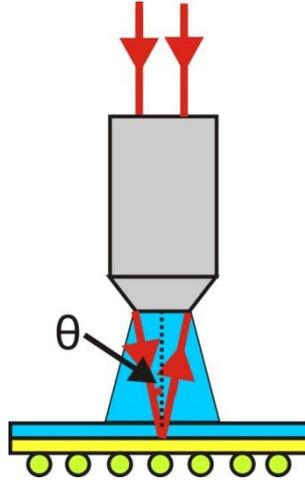
Fig. 3-5 Excitation of SPR by using a high NA oil-immersion objective
