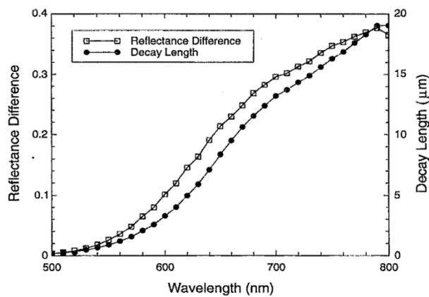
Fig. 2-24 Reflectance difference for bare gold and gold coated with 2.5nm  $SiO_2$  (circles) and surface plasmon decay lengths (squares) [40]
