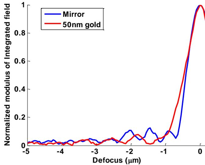
Fig. 4-18  $V(z)$  curve of mirror and 50nm gold without pupil function modulation;
