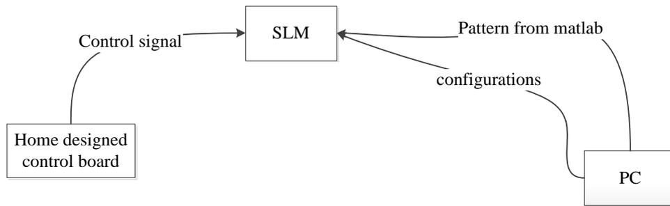
Fig. 3-18 hardware connection of the SLM
