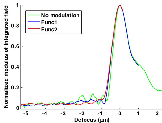
Fig. 4-19  $V(z)$  curves comparison with no pupil function modulation, modulated pupil function 1, and optimized modulated pupil function 2
