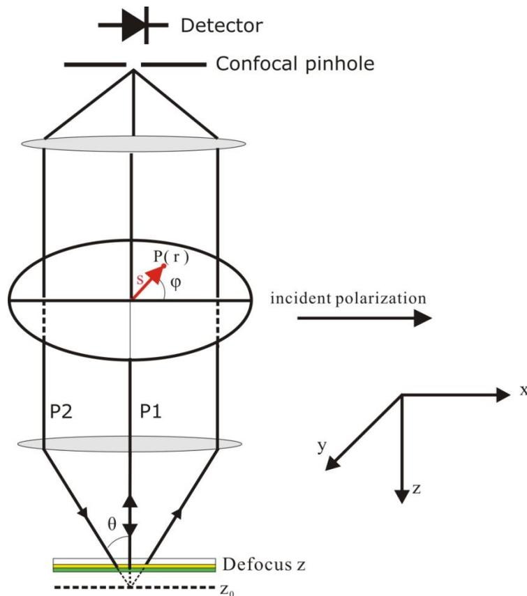
Fig. 4-1 systematic diagram of defocus and back focal plane
