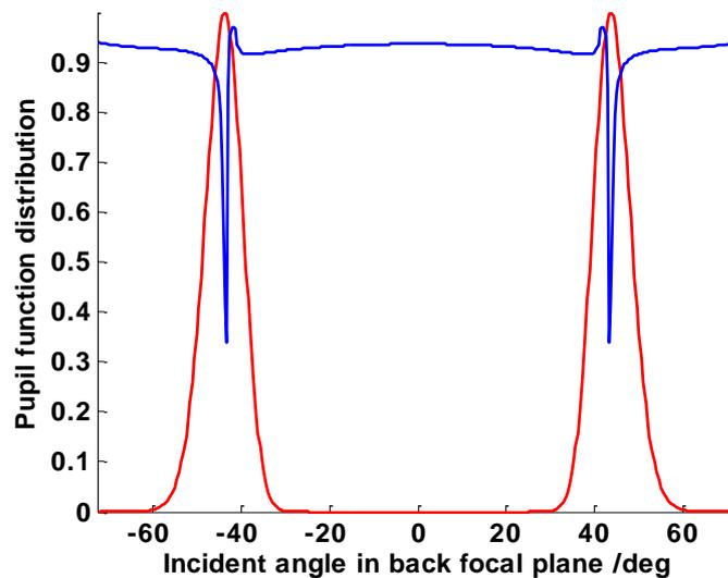
Fig. 6-8 Pupil function distribution (red curve) for the direct measurement of the propagation length and calculated reflection coefficient for p-incident polarization on an uncoated sample (blue curve);
