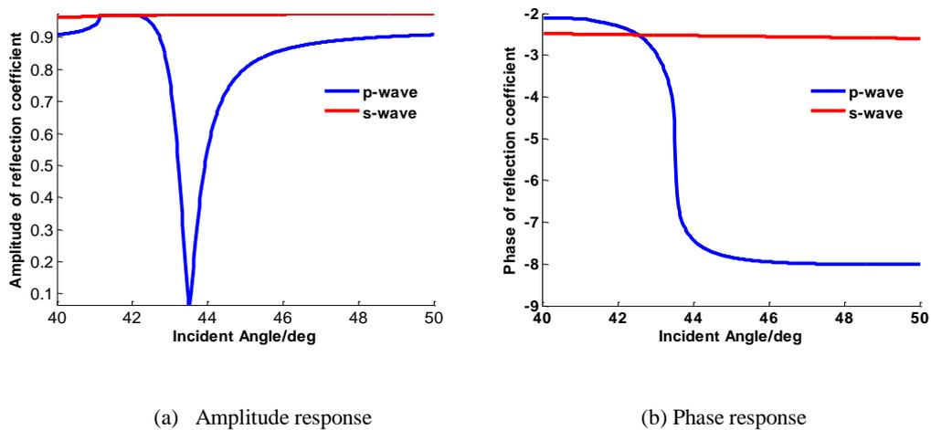
Fig. 2-9 Comparison of SPR excitation by using p and s polarized illumination
