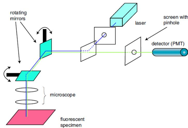
Fig. 2-31 Basic setup of a beam scanning microscope[84]
