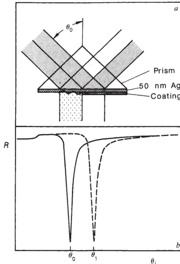
Fig. 2-19 Imaging contrast mechanism of the SPRM [12]
