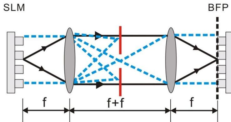
Fig. 3-7 4-f projection structure of the SLM
