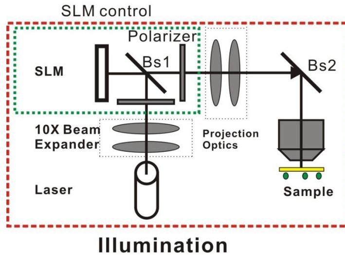
Fig. 3-3 Schematic diagram of the illumination part
