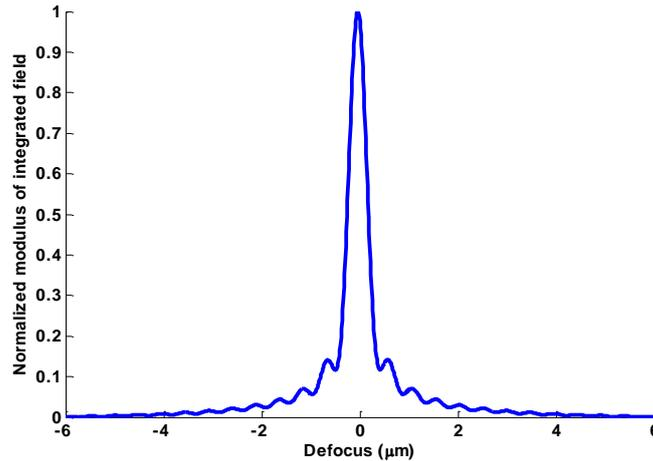
Fig. 4-5  $V(z)$  of non-plasmonic sample. The ripples are caused by the sharp edge effect.
