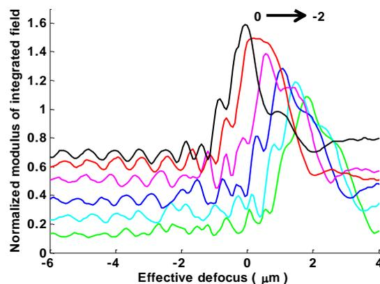
Fig. 5-14  $V(\alpha)$  curves obtained with different amounts of physical defocus . The black line to the bottom green line, represent fixed physical defocusses of 0, -0.4, -0.8, -1.2, -1.6, -2 respectively. The curves are displaced along the y-axis by 0.2 units for clarity. Line order black (solid), red(dashed), magenta (dotted), blue (solid), cyan (dash), green (dotted).
