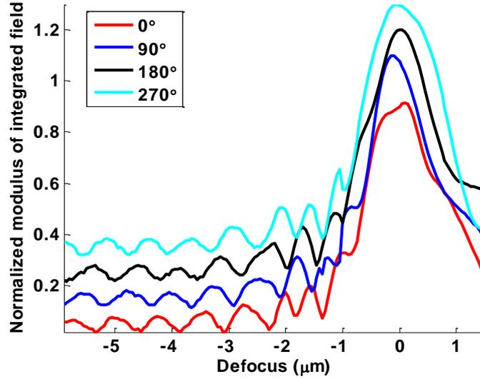
Fig. 6-4  $V(z)$  curves variations of bare gold obtained by shifting the phase of the reference in increments of 90 degrees. From lower to upper figures I have: zero phase shift (red), 90 degree phase shift (blue), 180 degree phase shift (black) and 270 degree phase shift (cyan). Successive curves are shifted by 0.1 units for clarity.
