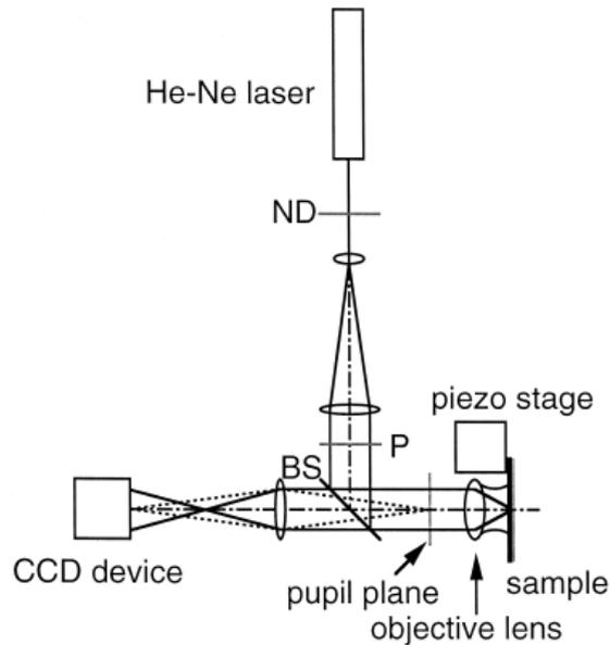
Fig. 2-22 system setup of back focal plane scanning SPRM by Kano [75]
