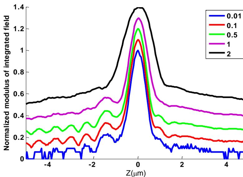
Fig. 4-17 Experimental  $V(z)$  curves on 50nm gold sample for different pinhole radii
