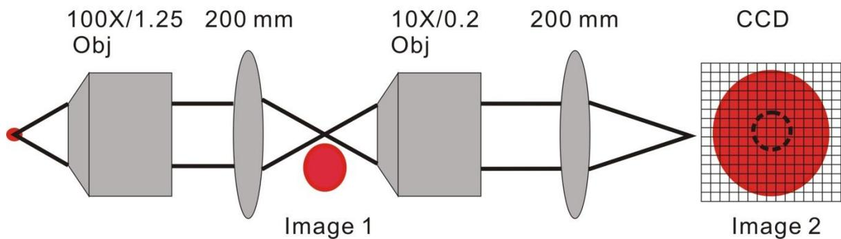
Fig. 3-9 Schematic diagram of the focal point magnification system
