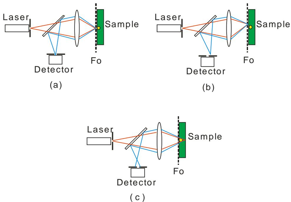
Fig. 2-32 Schematic of confocal laser scanning microscope, (a) focal plane; (b) off-axis; (c) defocus
