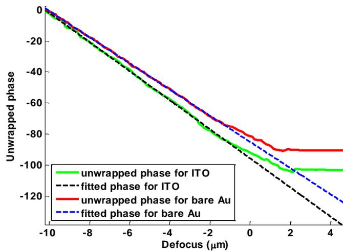
Fig. 6-5 Calculated  $\varphi(z)$  from four  $V(z)$  curves by using phase-stepping technique. The red curve refers to the unwrapped  $\varphi(z)$  of bare gold and the blue line is the fitted data, while the green curve refers to the ITO coated sample case and the black line is the linear fitted data.
