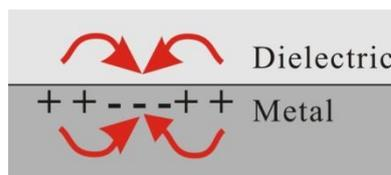
Fig. 2-1 Collective oscillation along a metal - dielectric interface
