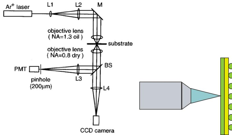
Fig. 2-21 Optical setup of Sample scanning SPRM by Kano [36]
