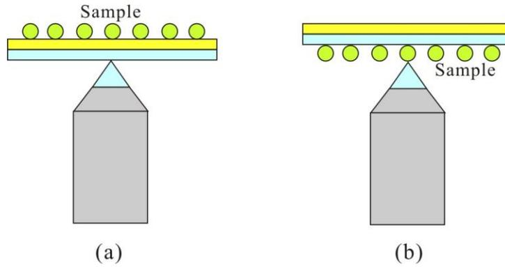
Fig. 1-1 Comparison of sample location from the point view of direction of observation. (a) shows the SPR technique; (b) shows the other techniques.
