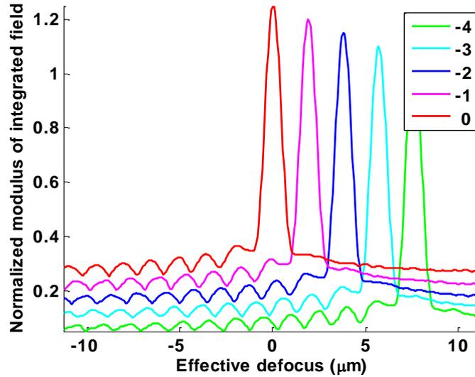
Fig. 5-6 Simulation  $V(\alpha)$  results comparison on the effect of defocus. From the top red curve to the bottom green curve represent fixed physical defoci of -4, -3, -2, -1 and 0 respectively. The curves are displaced along the y-axis by 0.1 units for clarity.
