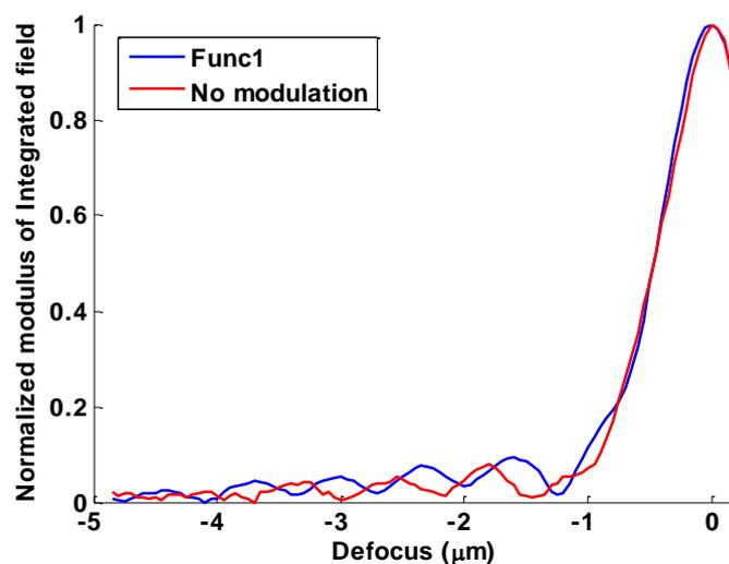
Fig. 4-20  $V(z)$  curves of 50nm gold without modulation and by using Func1 pupil function
