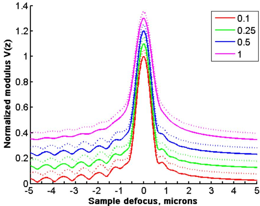
Fig. 4-4 Simulated  $V(z)$  curves for different pinhole diameter. Solid curve 50nm bare gold, dashed curves gold with 10nm overlayer with refractive index 1.5. Each pinhole diameter displaced by 0.1 in y-axis and overlayers displaced by 0.05 in y-axis to distinguish the curves. Pinhole radii defined in terms of radius of Airy disc  $(0.61\lambda/NA)$  are shown in the legend.
