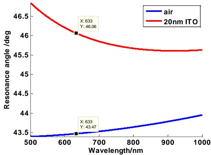
Fig. 3-4 Plasmonic resonance angle v.s. wavelength of illumination source
