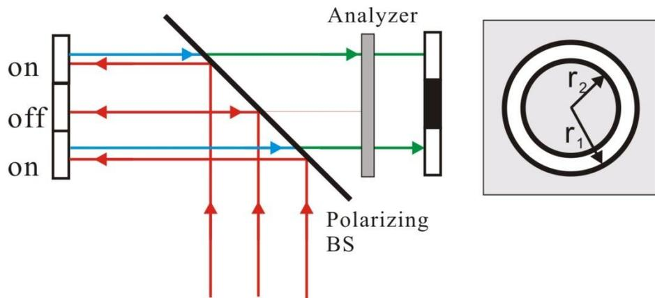
Fig. 3-12 Optical alignment schematic diagram of the amplitude SLM
