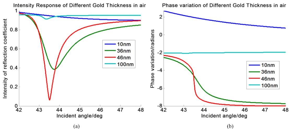
Fig. 2-11 Comparison of SPR excitation by using different gold thickness samples (glass/gold/air)
