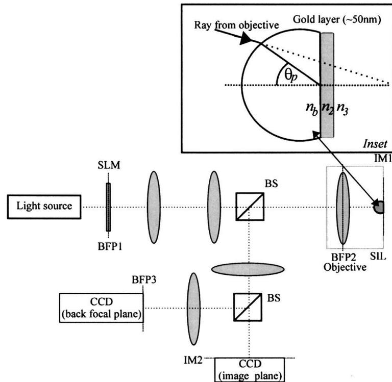
Fig. 2-23 Optical setup of the SIL wide-field objective [76]
