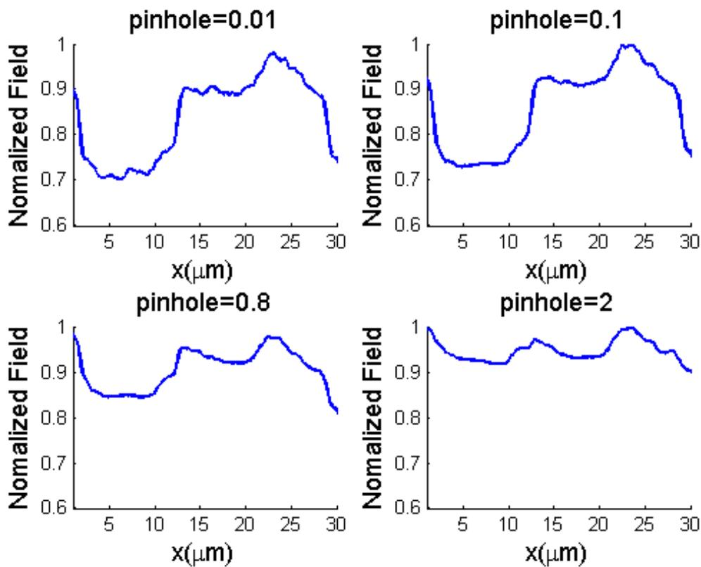
Fig. 4-23 One dimensional grating images at  $-1.25\mu\text{m}$  defocus using different pinhole radii
