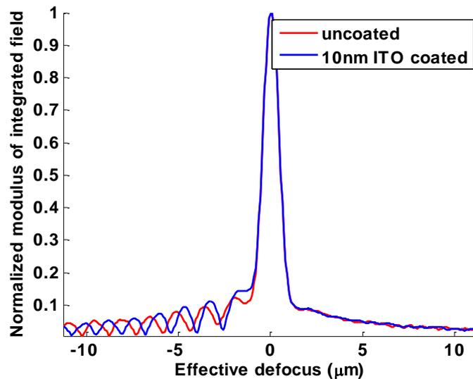
Fig. 5-5 Simulated  $V(\alpha)$  curve movement when using the bare gold (red curve) and 10nm ITO coated sample (blue curve)
