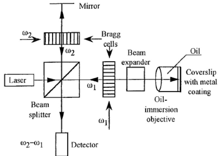
Fig. 2-26 schematic diagram of the scanning heterodyne interferometer [4, 5]
