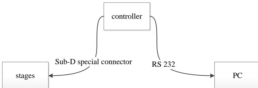
Fig. 3-15 hardware connections of the stages
