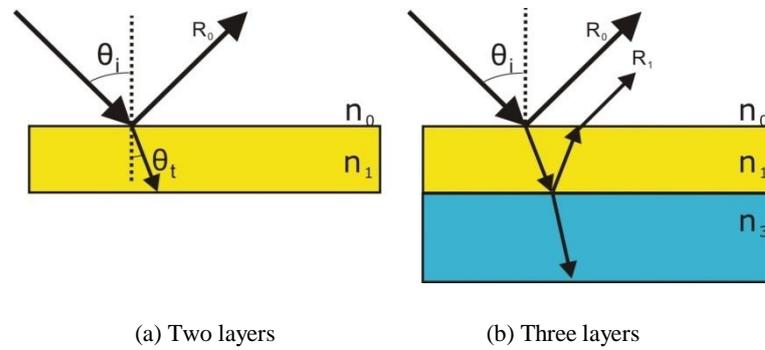
Fig. 2-8 Sample structure for Fresnel equations
