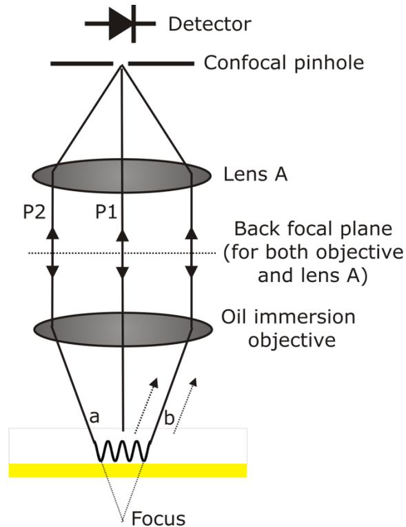
Fig. 1-2 Diagram of the confocal surface plasmon microscopy figure
