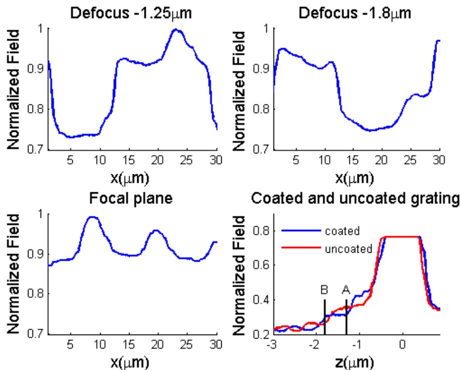
Fig. 4-22 One dimensional grating images with different defoci. Bottom right shows  $V(z)$  curves on coated and uncoated regions explaining contrast reversal
