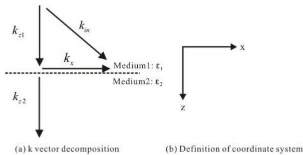
Fig. 2-2 The definition of coordinate system and the k vector decomposition in both dielectric and metal
