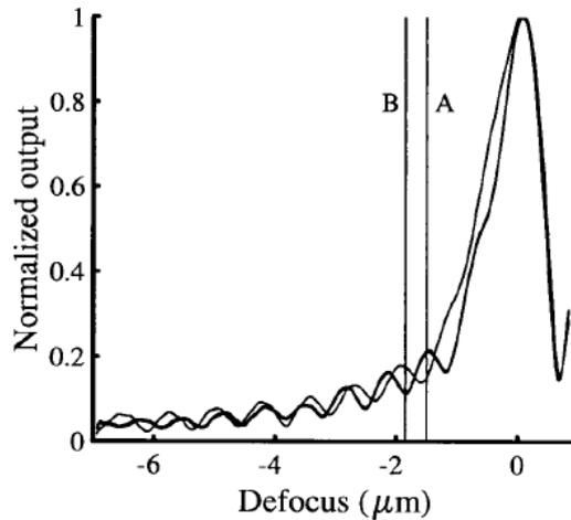
Fig. 2-28  $V(z)$  curves by scanning the coated sample and uncoated sample, thin and thick line refers to the on and off part of the grating sample, thin line refers to the coated section and thick line is that of the uncoated section [4, 5]. Here the minus defocus means the distance between the sample and the objective lens is shorter than the focal length of the lens.
