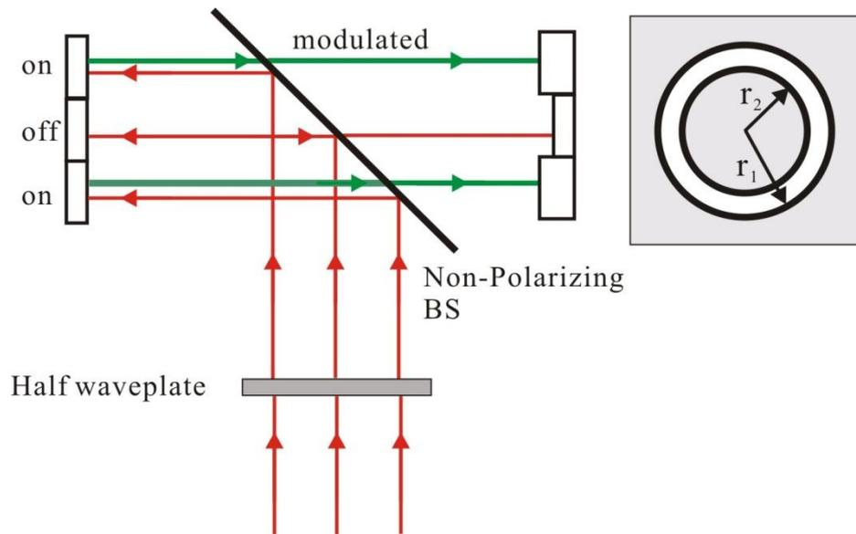
Fig. 3-22 optics alignment of the phase SLM
