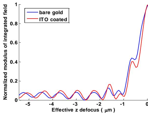
Fig. 5-13  $V(\alpha)$  comparison between uncoated and ITO coated sample, the red line is the ITO coated case and blue line is the uncoated case;
