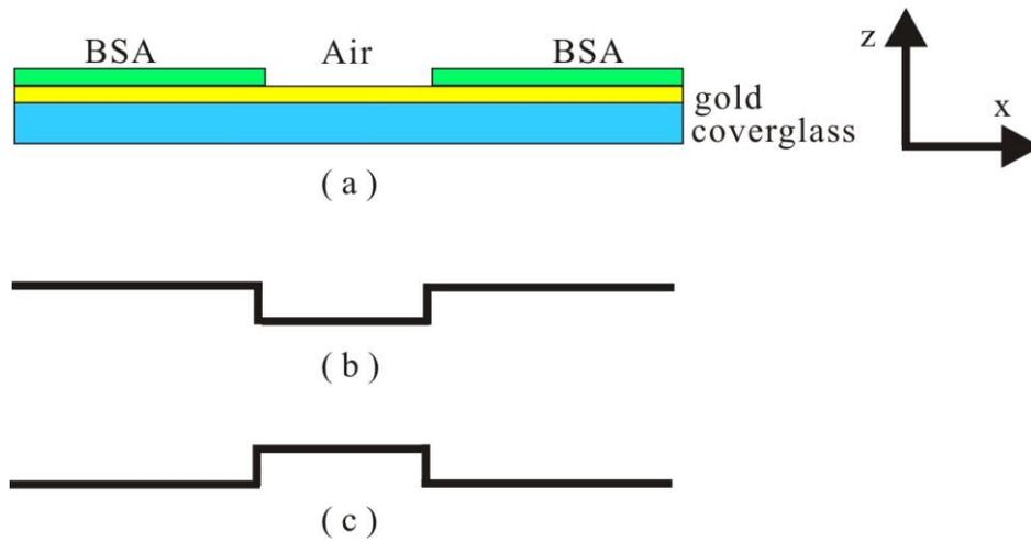
Fig. 4-14 (a) BSA grating structure; (b) theoretically grating image when using near defocus; (c) inverted theoretically grating image when using farther defocus;
