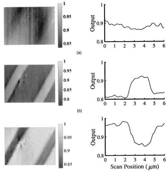
Fig. 2-29 Scanning images from the scanning heterodyne interferometric SPRM with different defocus. (a)  $z=0$ ;(b)  $z=-1.5\mu\text{m}$ ;(c)  $z=-1.8\mu\text{m}$  [4, 5]
