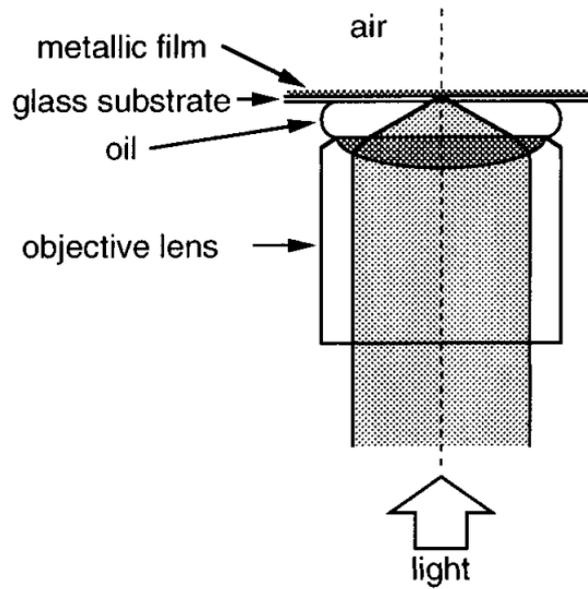
Fig. 2-20 SPR excitation by using an oil-immersion objective lens invented by Kano[36]
