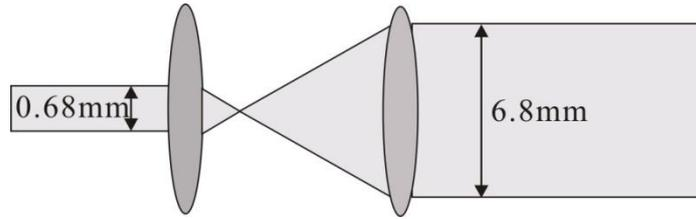
Fig. 3-6 Schematic diagram of the 10X beam expander
