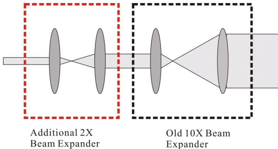
Fig. 3-21 Modified beam expander
