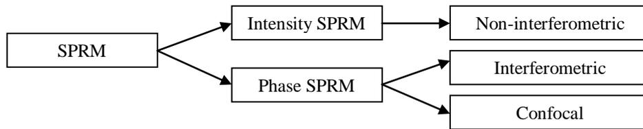
Fig. 2-18 Classification diagram of different type of SPRM in this thesis
