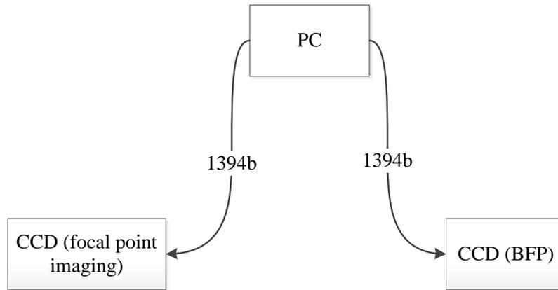
Fig. 3-16 CCD cameras connection
