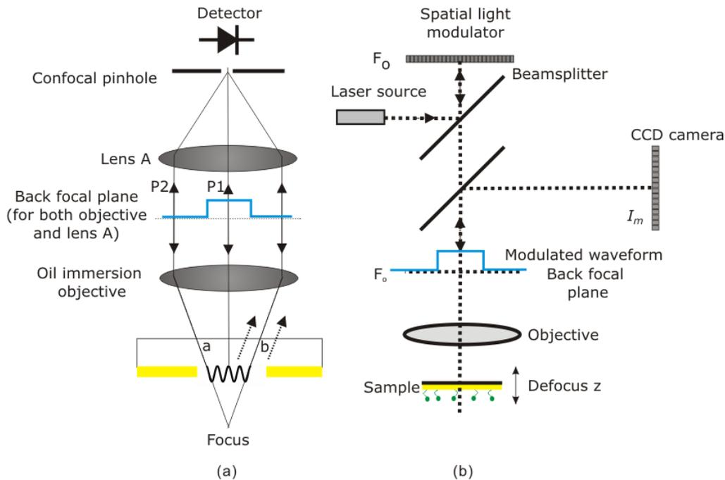
Fig. 6-1 (a) Simplified schematic showing operation of confocal microscope with SP excitation; (b) Schematic of optical system showing relationship between different planes in the system. The blue waveform indicates phase modulation in the back focal plane.
