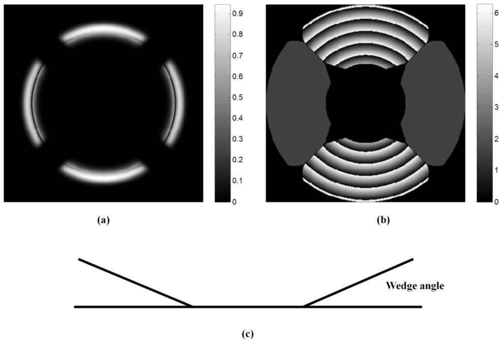
Fig. 7-3 (a) Amplitude pupil function used for the artificial plasmon; (b) Phase pupil S wedge angle = -0.1111 degrees; (c) unwrapped phase pattern; Pixel size=15 microns and one-sided wedge=100 pixels and back focal plane size=357 pixels
