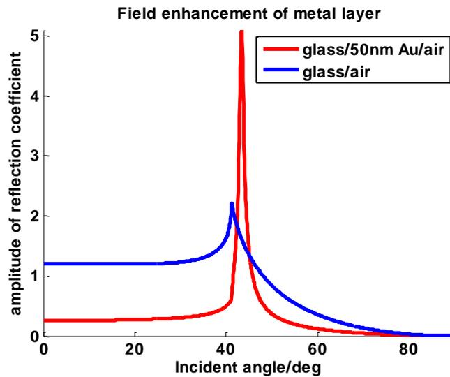
Fig. 2-10 Comparison of the excited electric field enhancement when using a sample structure with gold layer (red curve) and without gold layer (blue curve)
