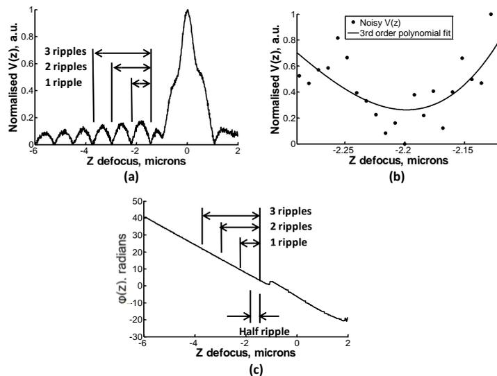
Fig. 6-6 (a) shows the method of measuring the ripple period measurement (b) shows 3<sup>rd</sup> order polynomial fit (black) to locate a minimum position for ripple period measurement; (c) shows regions on  $\phi(z)$  and corresponding ripple positions.
