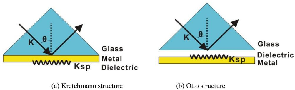
Fig. 2-6 prism based SPR excitation structure
