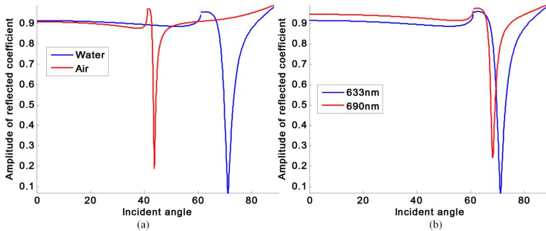
Fig. 7-1 (a) Simulated SPR excitation comparison in water and in air; (b) Simulated SPR excitation in water using 633nm and 690nm illumination respectively.
