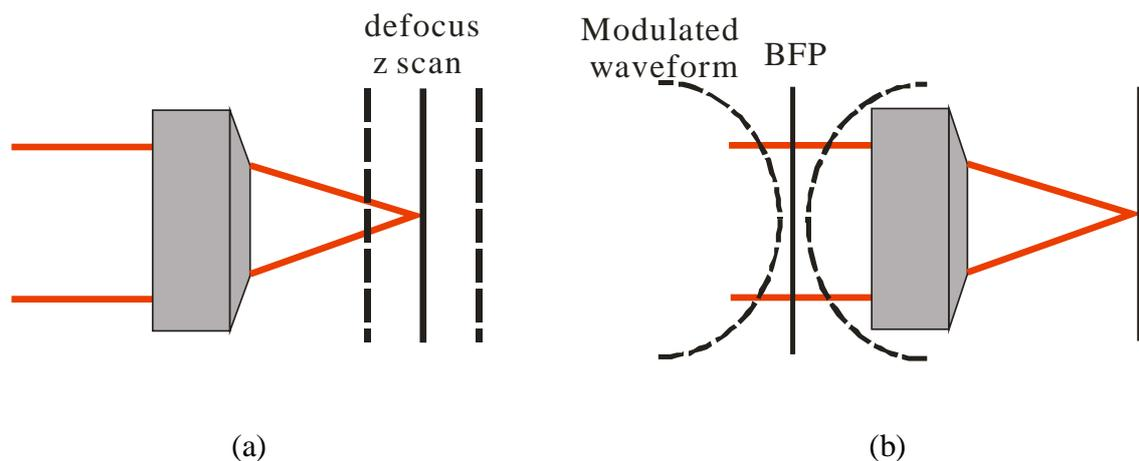
Fig. 5-3 from  $V(z)$  to  $V(\alpha)$ ; (a) the principle of  $V(z)$  by mechanically scanning the defocus along axial direction; (b) the principle of  $V(\alpha)$  by generating the phase pattern on the back focal plane
