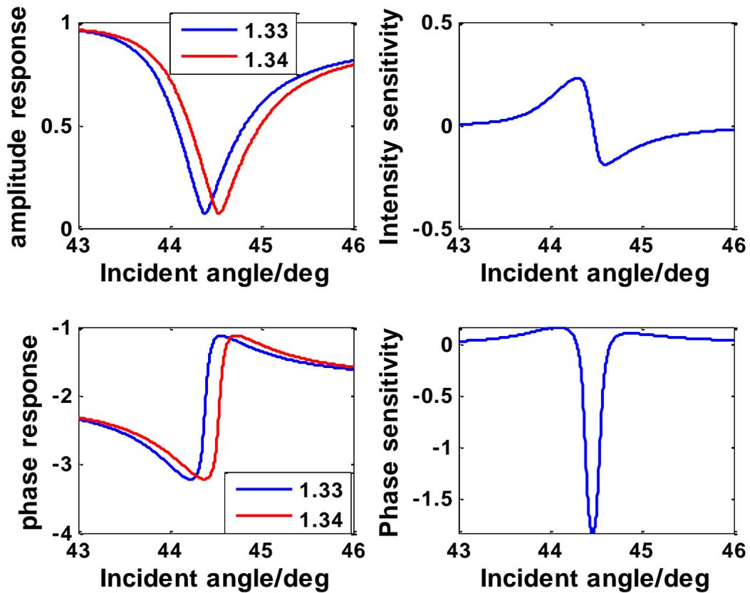
Fig. 2-17 Sensitivity comparison between intensity and phase when  $n_{dielectric}$  varies from 1.33 to 1.34
