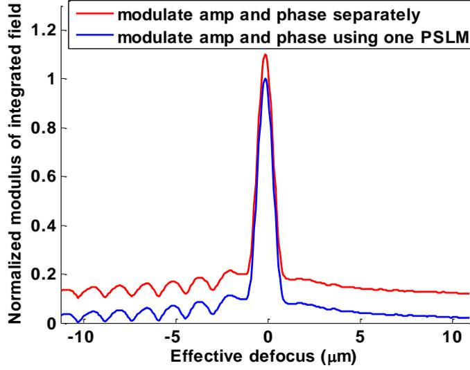
Fig. 5-7 Simulated results to show if amplitude modulation and the phase modulation independent; red curve is the result modulating the amplitude and phase separately and blue curve shows the result modulating both the amplitude and phase with one pure phase SLM. The red curve is displaced along the y-axis by 0.1 units for clarity.
