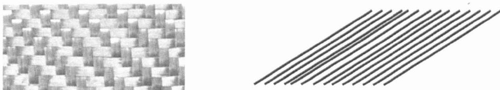
Figure 1.3 Structure of woven (left) and unidirectional fibre plies (right).
