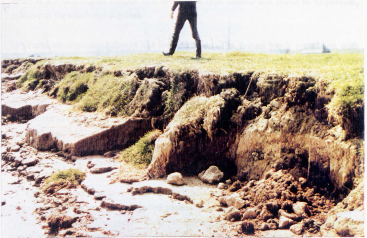
Plate 3.4 Disaggregated Blocks of Cohesive Bank Materials Following Mass Failure of IJssel River Banks, The Netherlands
