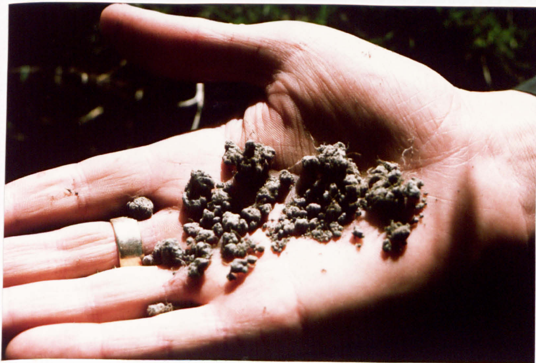
Plate 3.7 Non-Cohesive Aggregates of Cohesive Bank Materials
