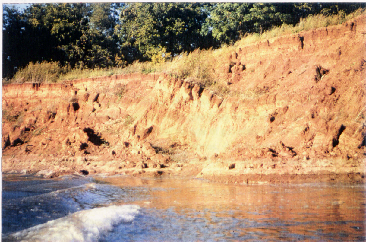
Plate 3.1 Geometry of Rotational Slip Failure on the Red River, Louisiana
