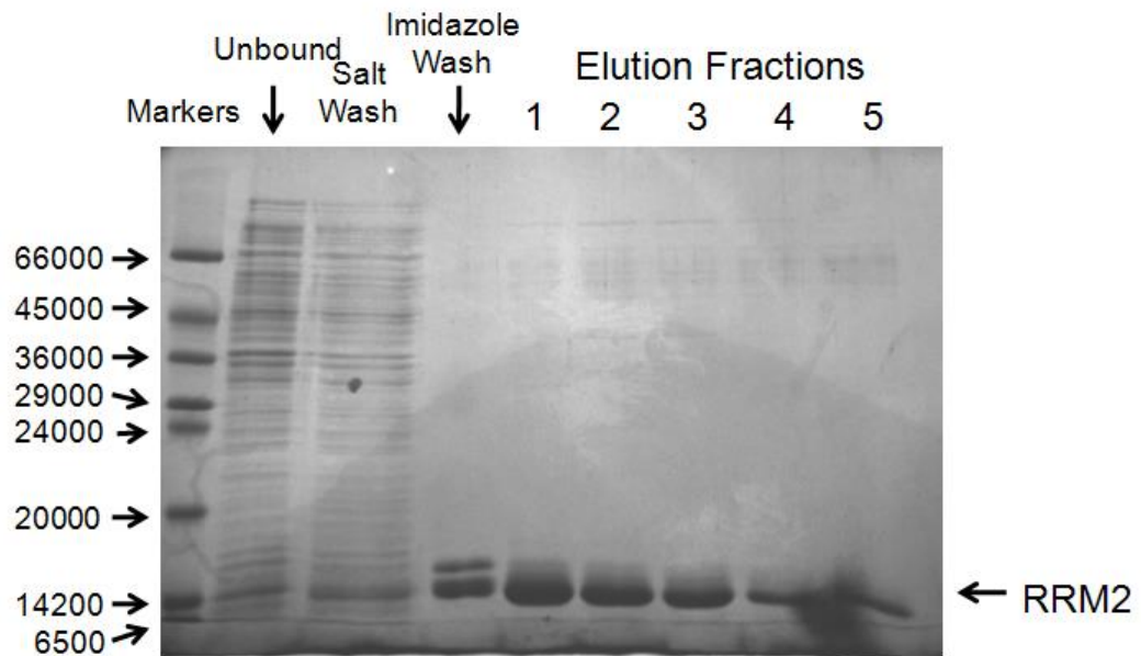
Figure 4.5: SDS-PAGE of washes and elution fractions from the IMAC column stage of the RRM2 purification. Significant quantities of protein were eluted by the 10 mM imidazole wash, which was reduced to 1 mM for the later purifications. The expected mass of the protein, allowing for the 6-His tag, was 9.6 kDa. The presence of multiple faint bands above the main RRM2 band suggests impurities bound to the protein.
