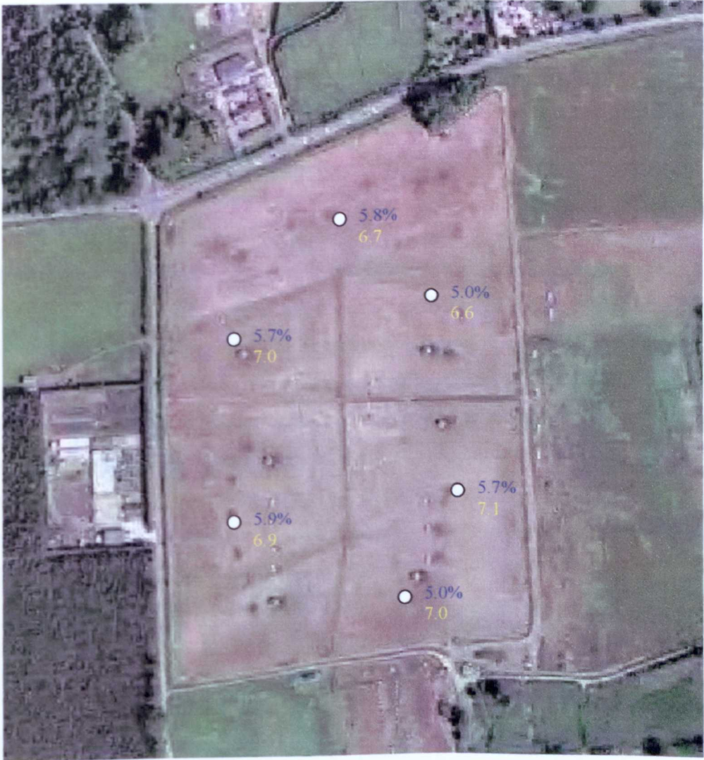
Figure 5.18: Soil sampling positions, Run 3. Soil moisture content: dark blue; pH: yellow.
