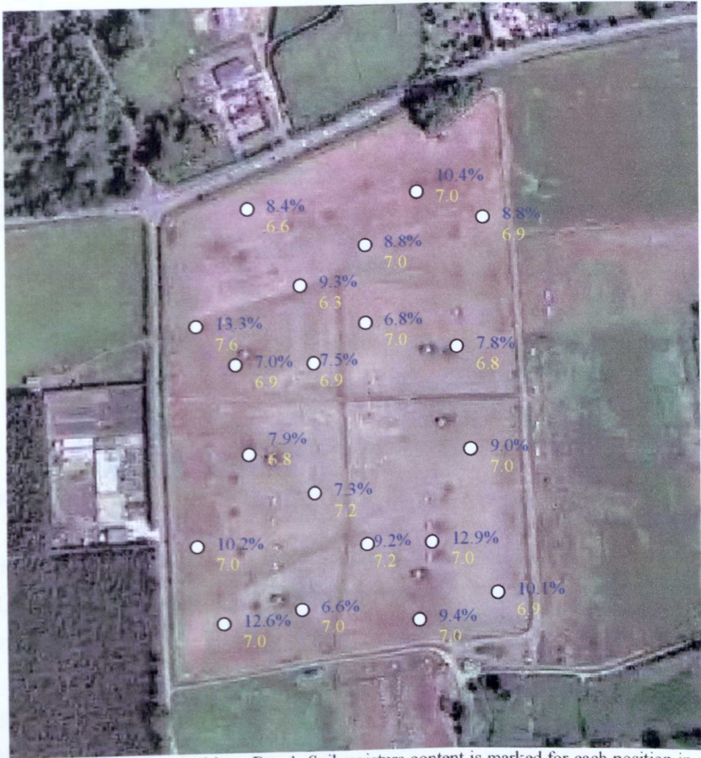
Figure 5.15: Soil sampling positions, Run 1. Soil moisture content is marked for each position in dark blue, whilst pH is yellow.
