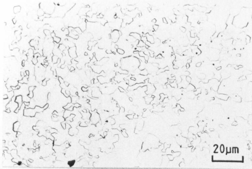
Fig. 3-1d Microstructure of the pure Zn used
