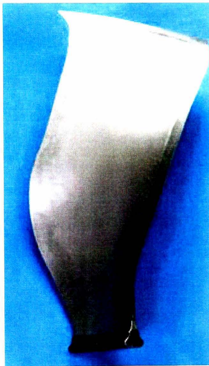
Figure 1.3 Wide-chord fan blade of an aero engine (Image Rolls Royce Plc) [5]
