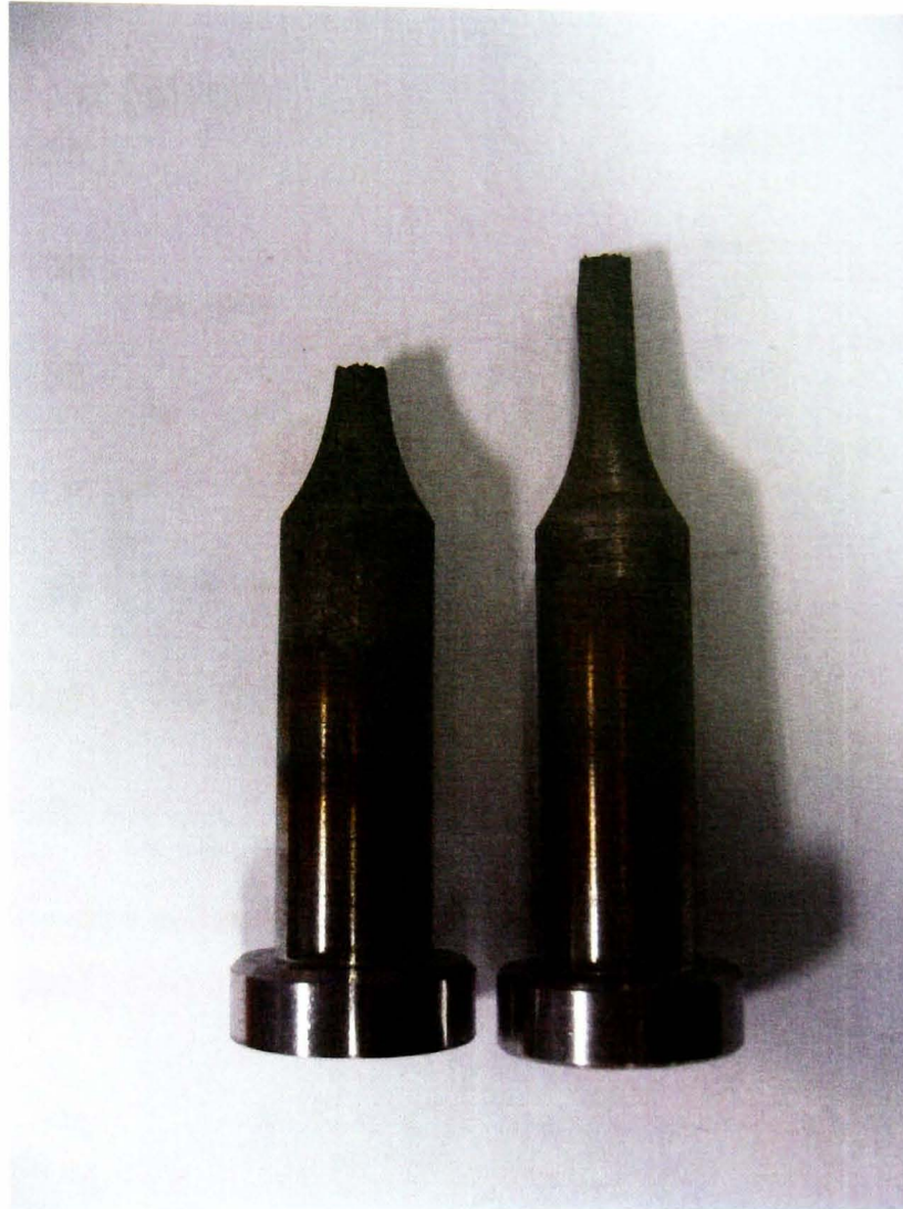
Fig. 3.28 Fractured specimen of the representative strain controlled TMF test.
