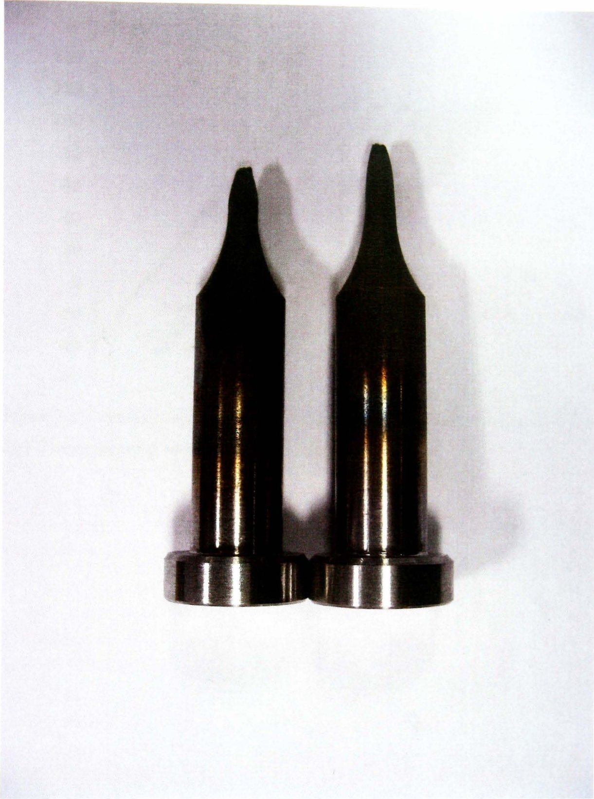
Figure 3.41 A fractured specimen from a stress controlled isothermal test at 900°C.
