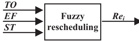
Figure 3.16: Fuzzy rescheduling with the inputs TO , EF , ST , and the output Re_i
