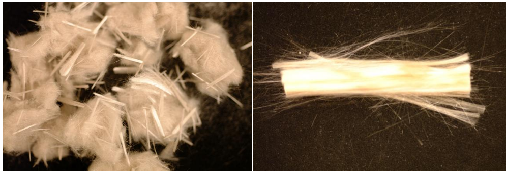
Figure 6-4: PGF showing severe corrosion with EA exposure for 15 minutes (left) and 5 minutes (right).
