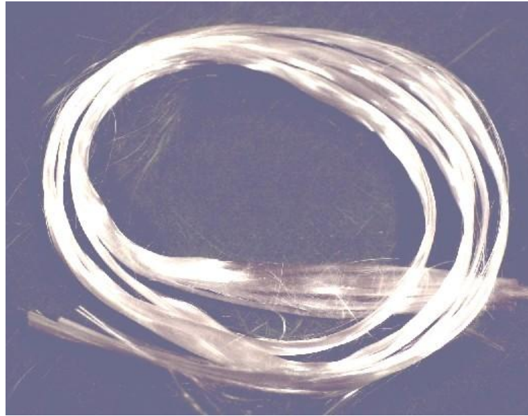
Figure 3-10: Melt drawn P45Fe4 glass fibre bundle, shows ease of fibre drawing with higher phosphate content
