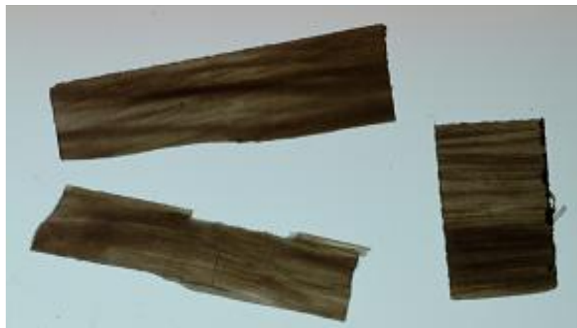
Figure 6-5: EA modified PGF reinforced composite shows severe corrosion and inferior mechanical properties
