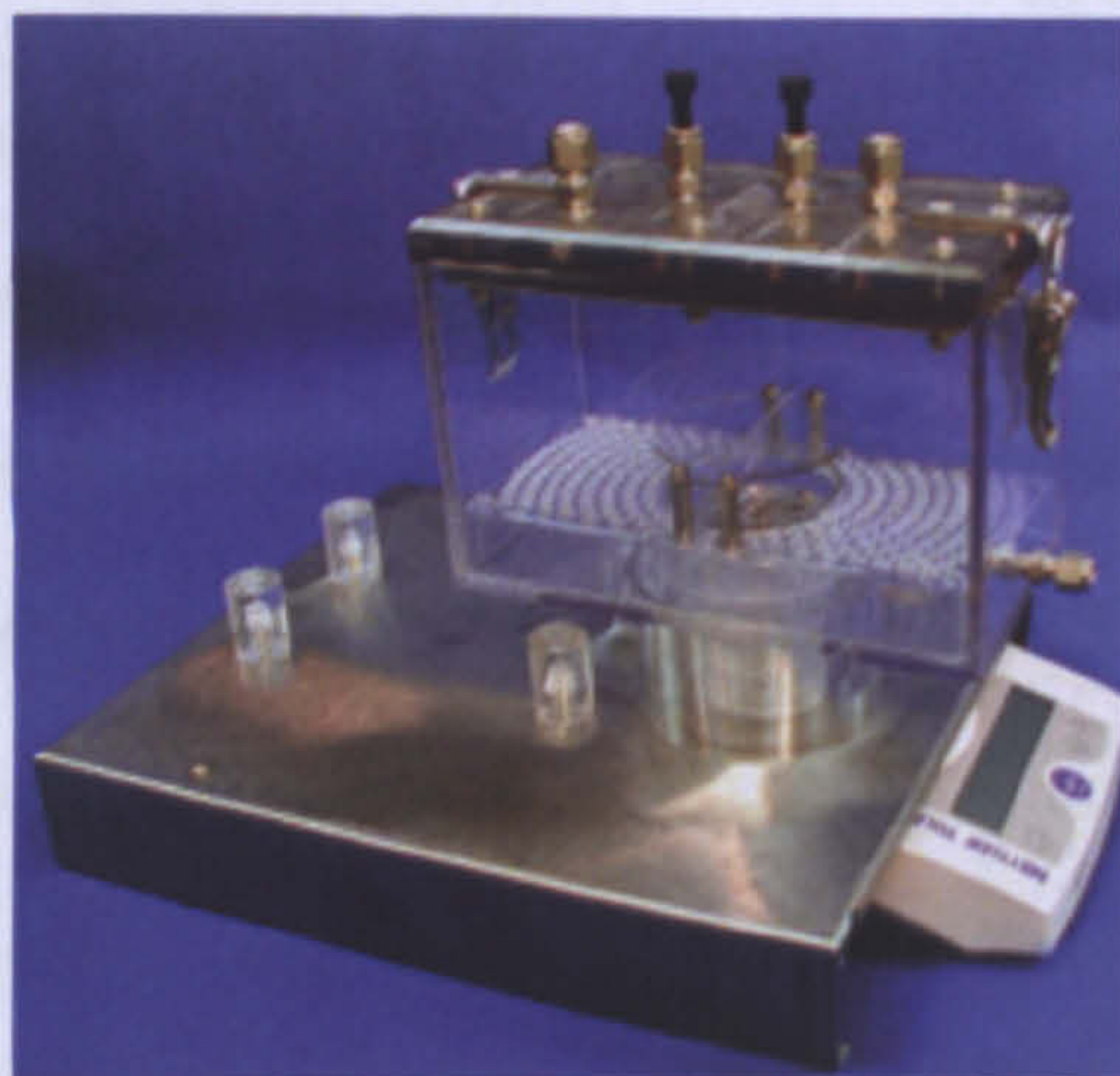
Picture 2: The above picture shows the food hopper which is independently filled and put in place on the base containing a digital scale, measuring the food hopper contents, with the
