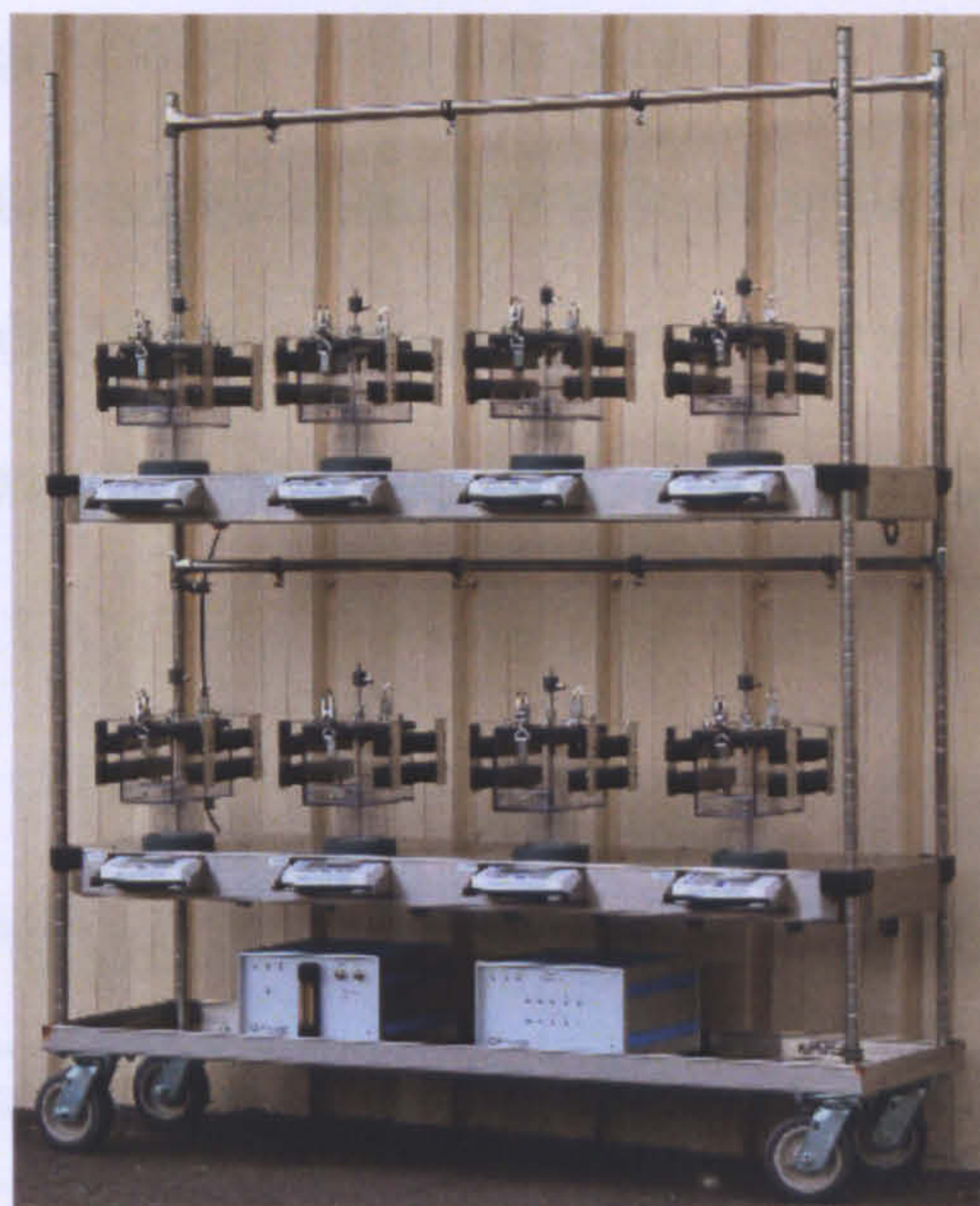
Picture 1: This picture displays the CLAMS setup as used in the following experiments described in this chapter. There are eight Perspex boxes all in a closed metabolic measurement system. Each animal setup is completely sealed so all metabolic gases, waste and food intake are accurately measured through computerised calibration systems. Data on those parameters as well as all movement and activity are electronically transferred and available for analysis.
