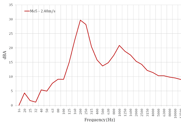
Figure 2.3.17: Measurement taken inside the building with a reference wind speed of 2.48m/s
