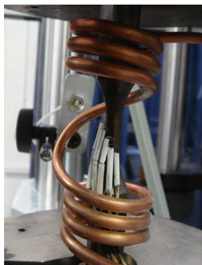
Figure 3.5: The positions of the 5 thermocouples along the gauge section during temperature calibration stage
