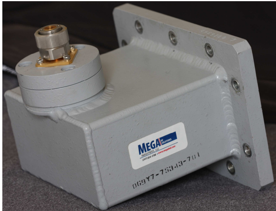
Figure 7.2. A waveguide-to-coaxial transition. Two identical transitions of this kind were used to insert the panel in between for this experiment.
