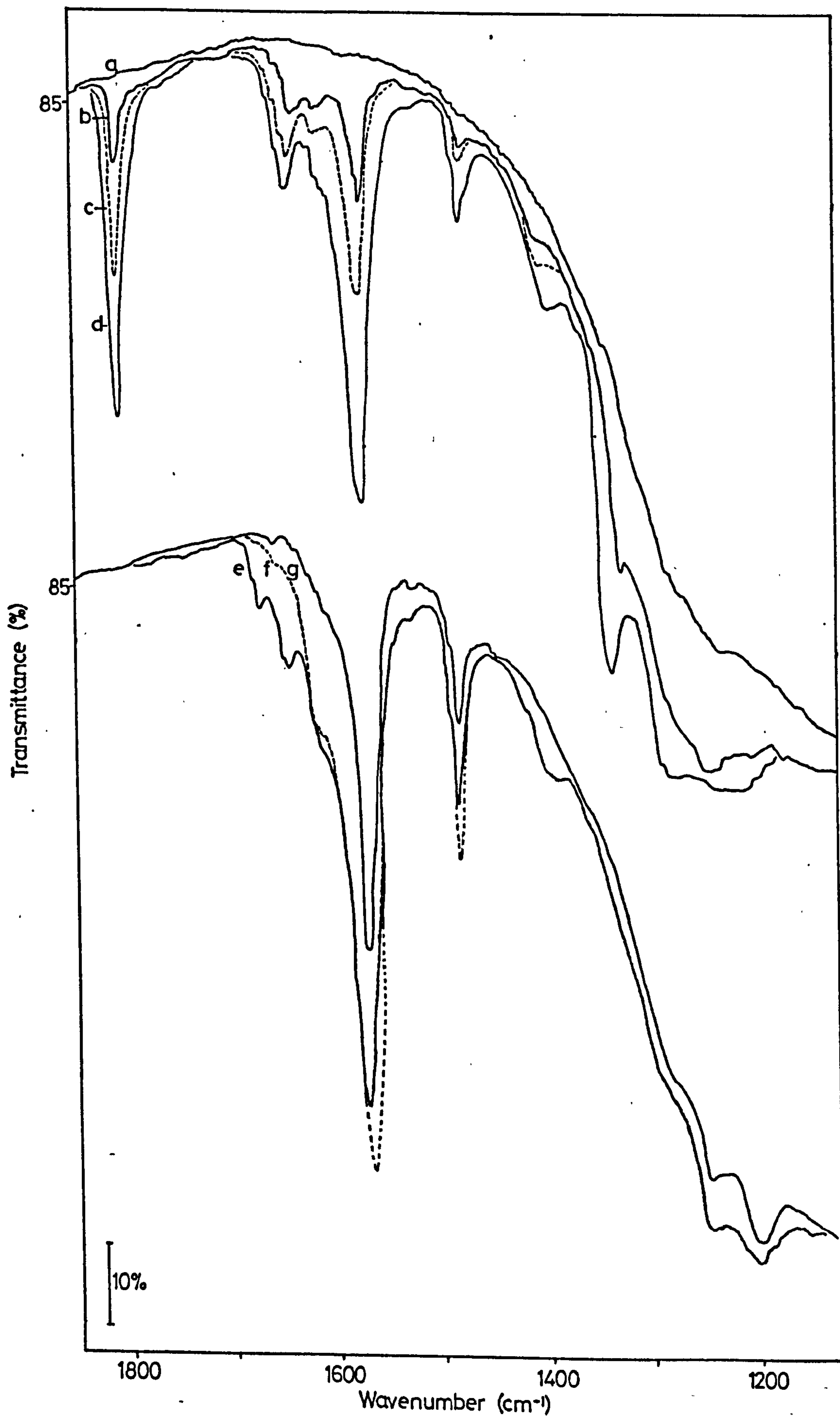
Spec 6.1 Adsorption of Hexafluoroacetone onto a 673 K Oxidized Surface
