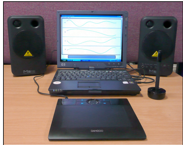
Figure 6-2: Experimental setup showing laptop with curve shape images and Wacom tablet for interacting with images to produce curve shape or curvature sonifications.
