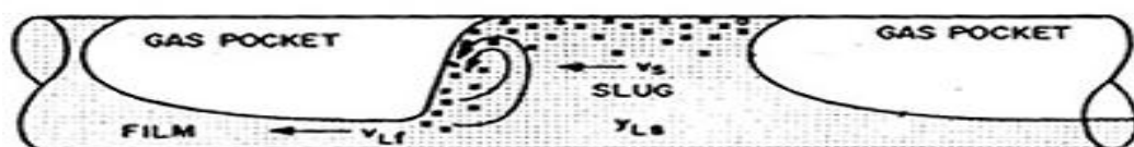
Figure 2.3: Horizontal slug flow
