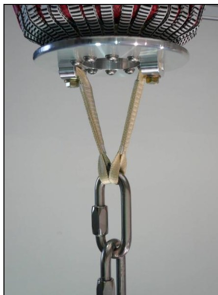
Fig. 8.5 Anchor rigging at the base of the bag
