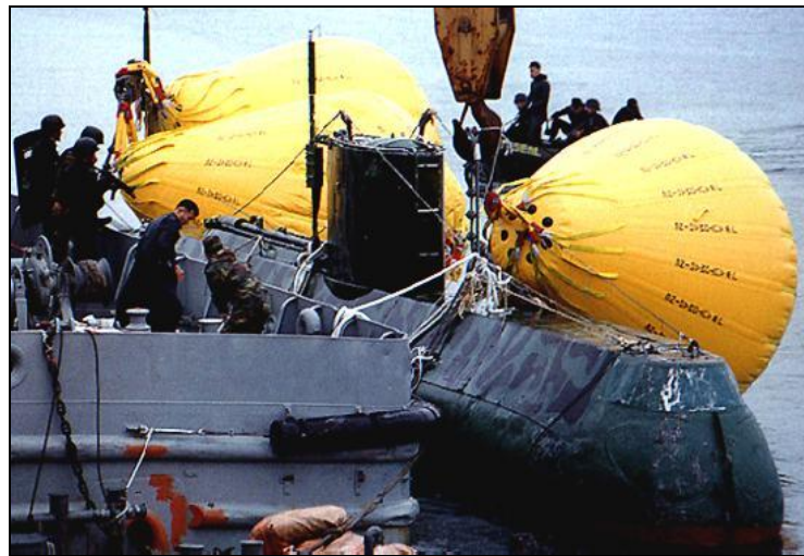
Fig. 2.12 35t closed bottom lifting bags used to raise a North Korean submarine [72]
