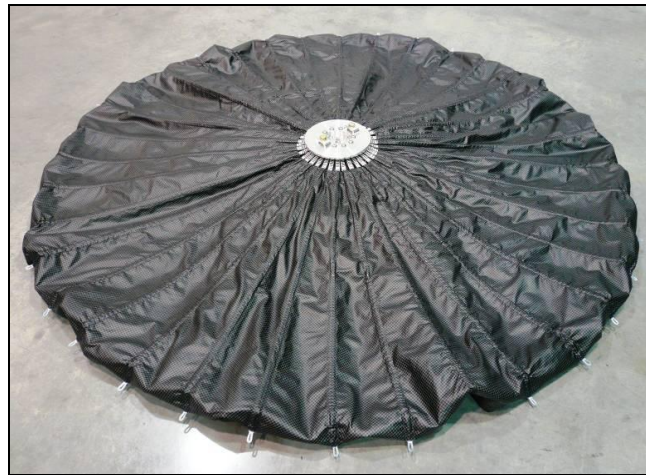
Fig. 5.3 A prototype Energy Bag with the UHPV architecture laid out on the ground. Wrinkling due to tendon shortening is visible
