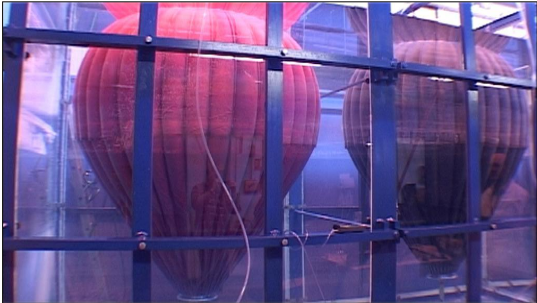
Fig. 8.6 The two 1/10 th scale prototype Energy Bags partially inflated underwater, with p_0 \approx 0
