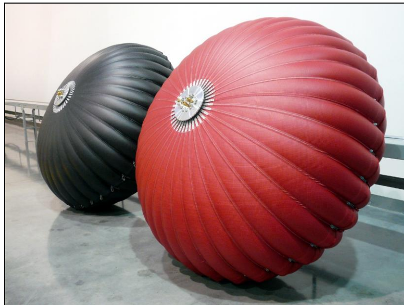
Fig. 8.1 The two 1/10 th scale prototypes undergoing a test inflation before installation in the tank
