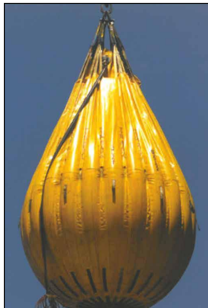
Fig. 2.17 A large water load test weight [80]
