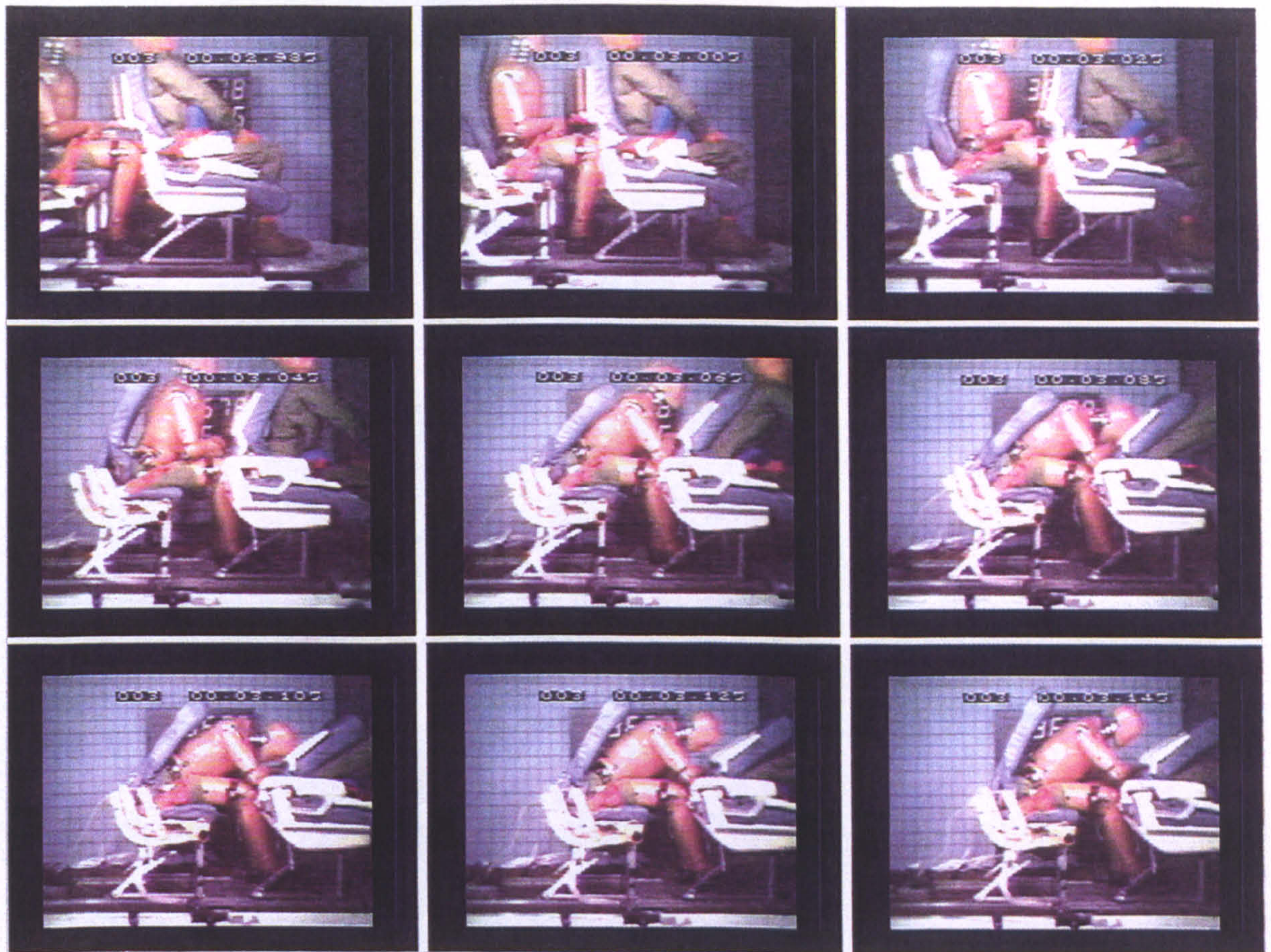
Fig. 16 Run No. 3678 - Unbraced/Legs Back, 28" Seat Pitch
