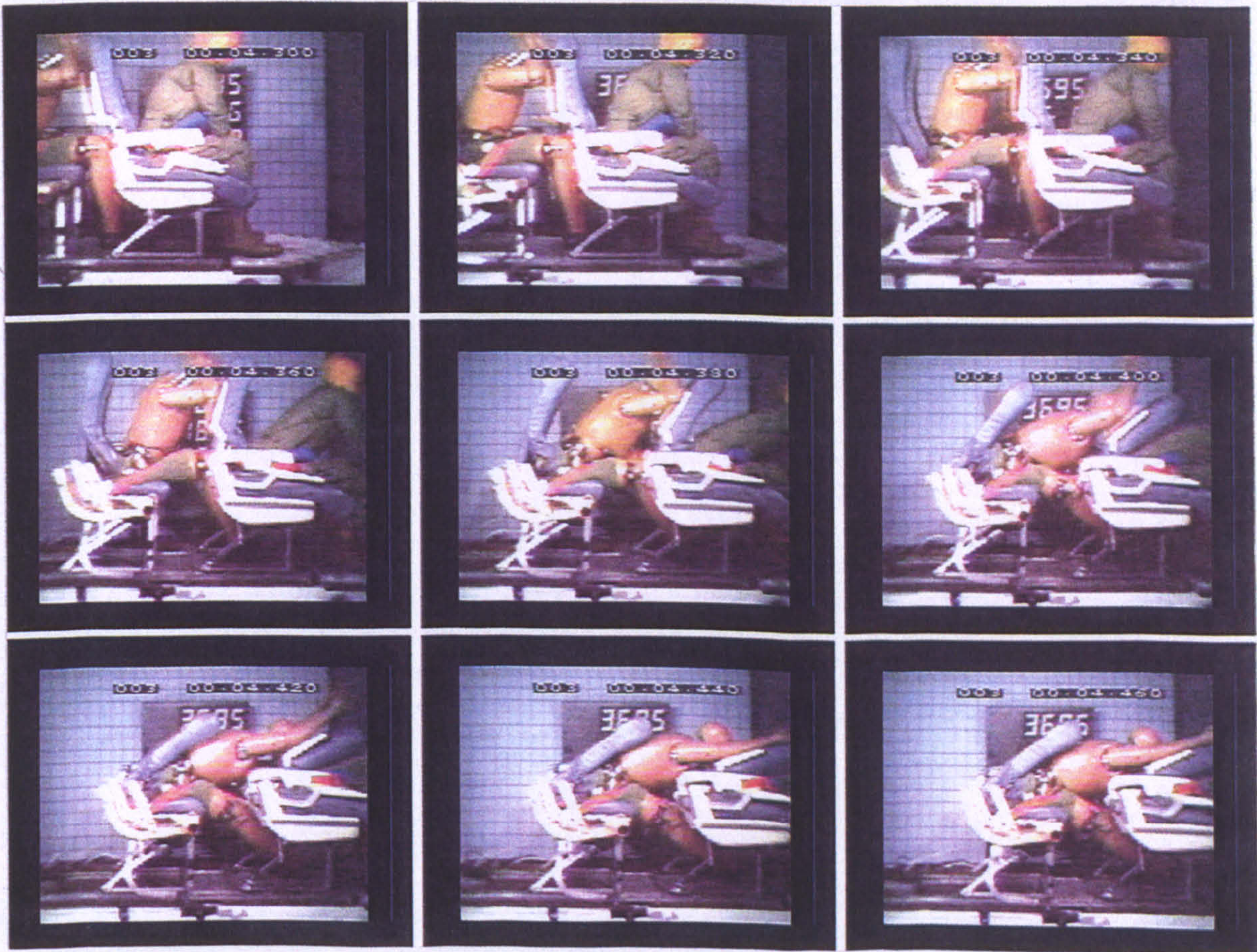
Fig. 15 Run No. 3695 - Braced/Legs Forward, 28" Seat Pitch
