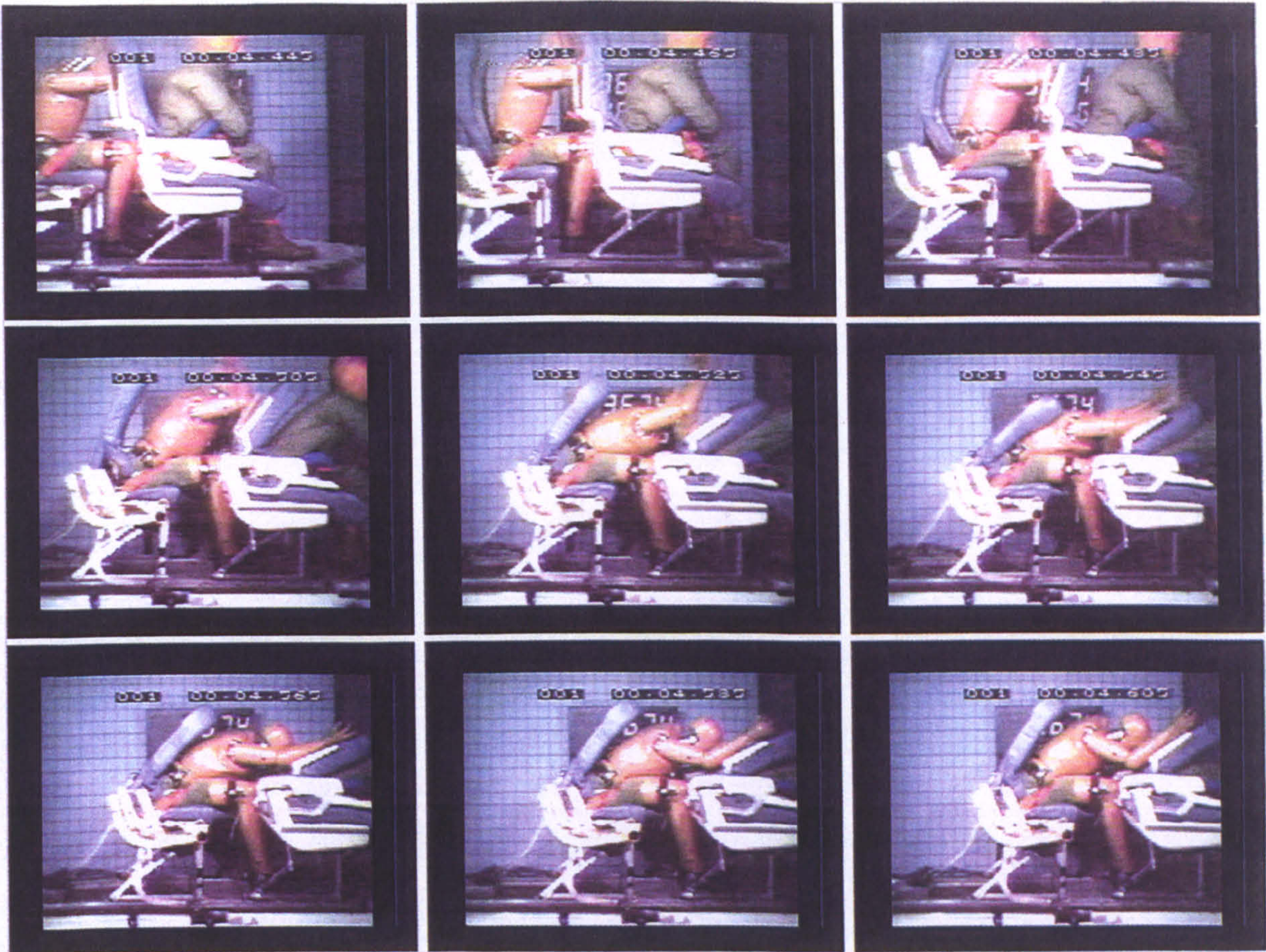
Fig. 14 Run No. 3674 - Braced/Legs Back, 28" Seat Pitch
