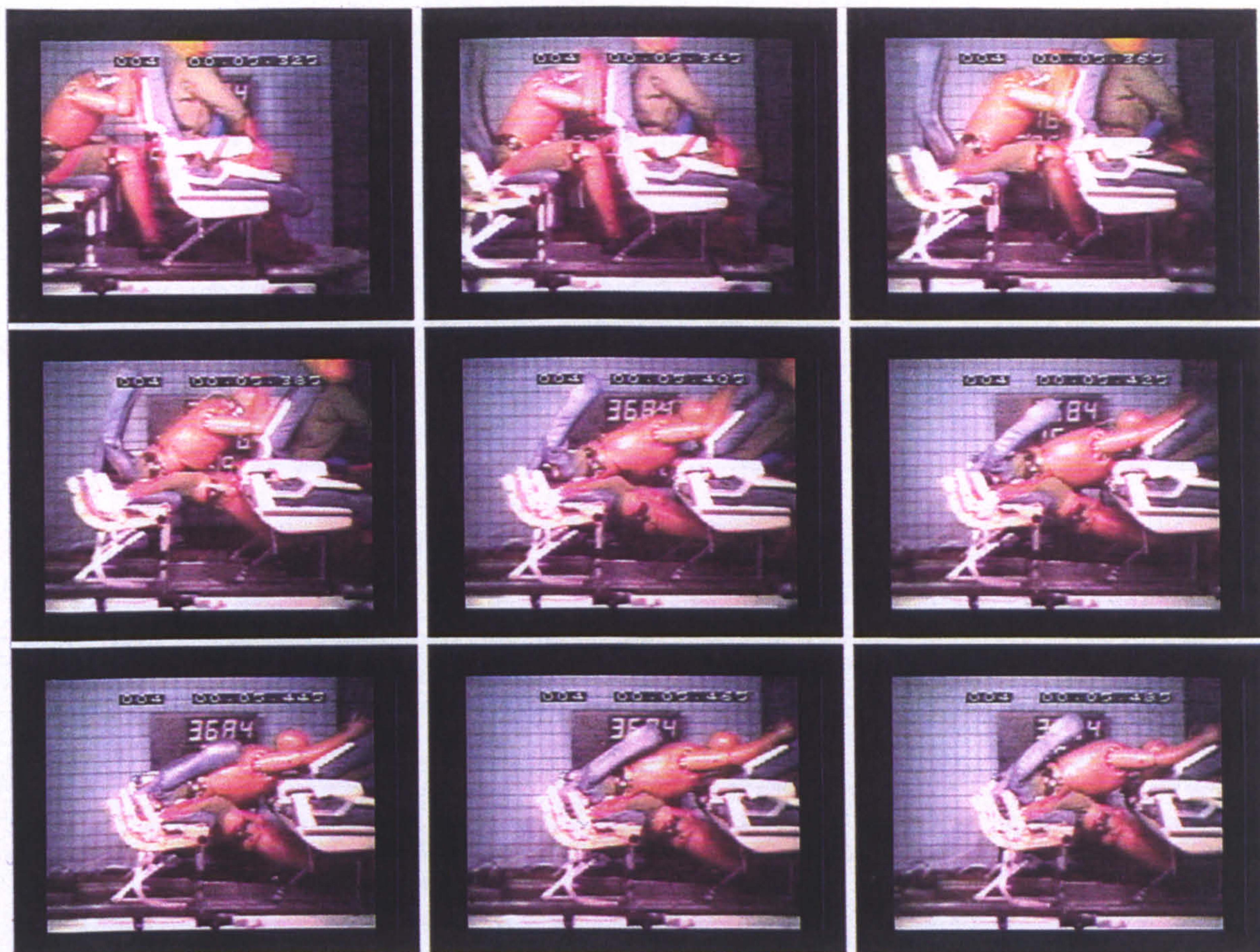
Fig. 11 Run No. 3684 - Braced/Legs Forward, 32" Seat Pitch
