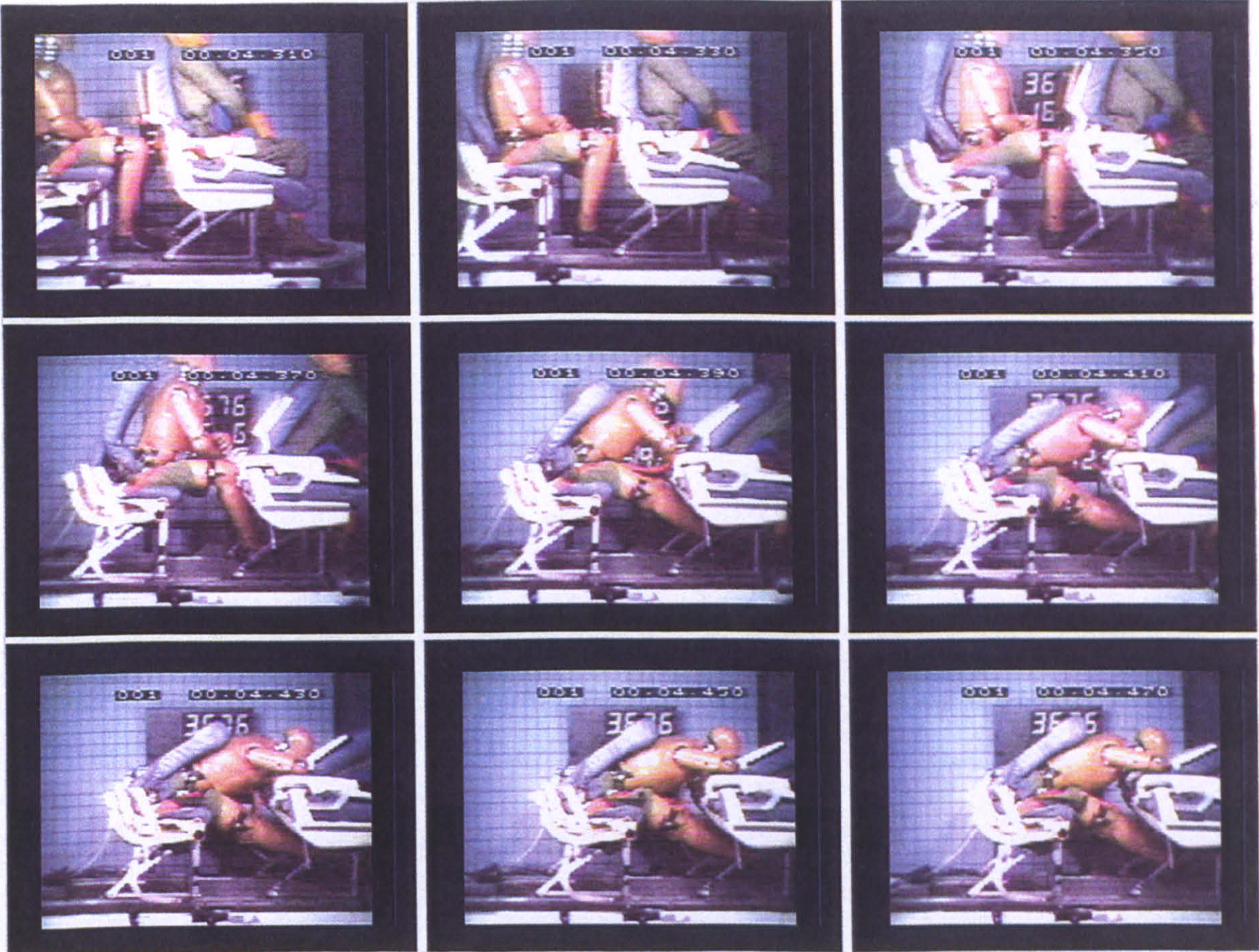
Fig. 12 Run No. 3676 - Unbraced/Legs Back, 32" Seat Pitch
