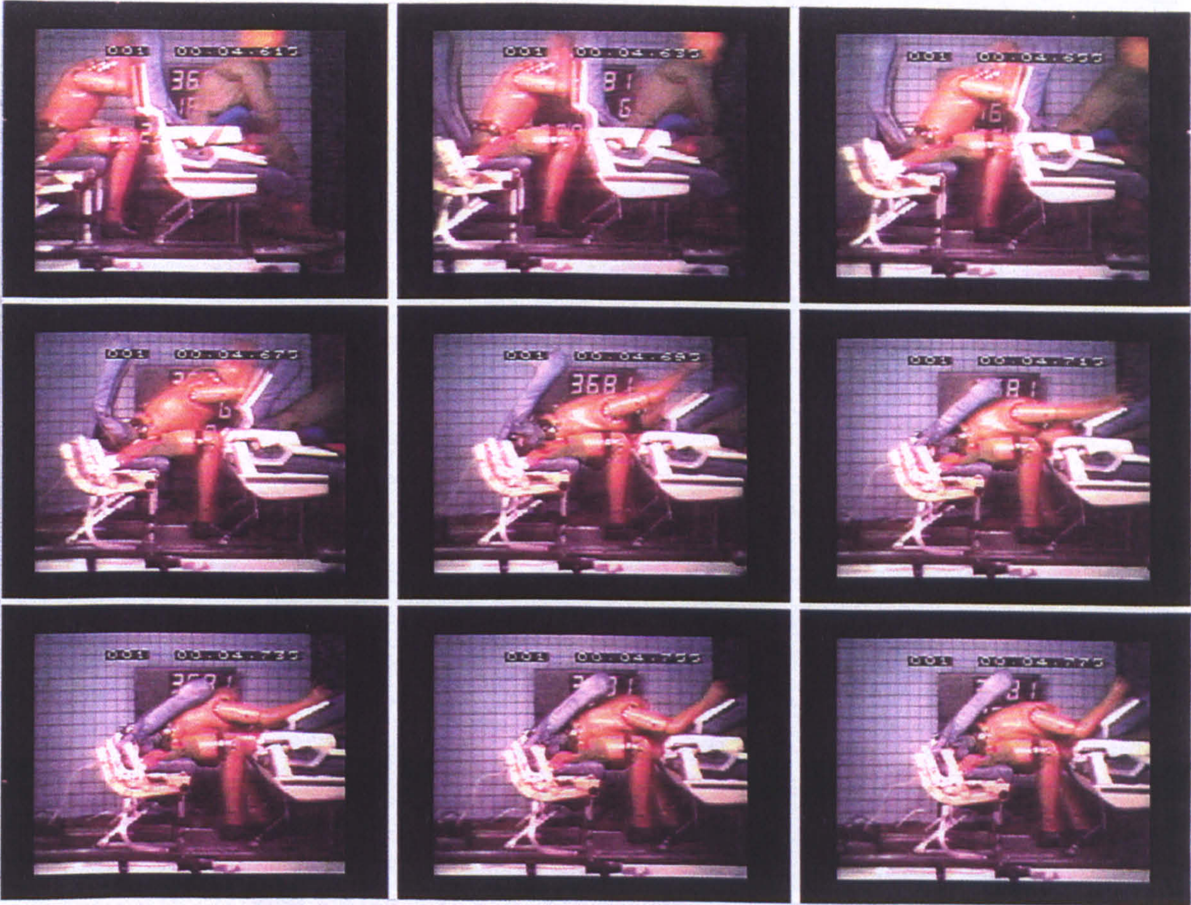
Fig. 10 Run No. 3681 - Braced/Legs Back, 32" Seat Pitch
