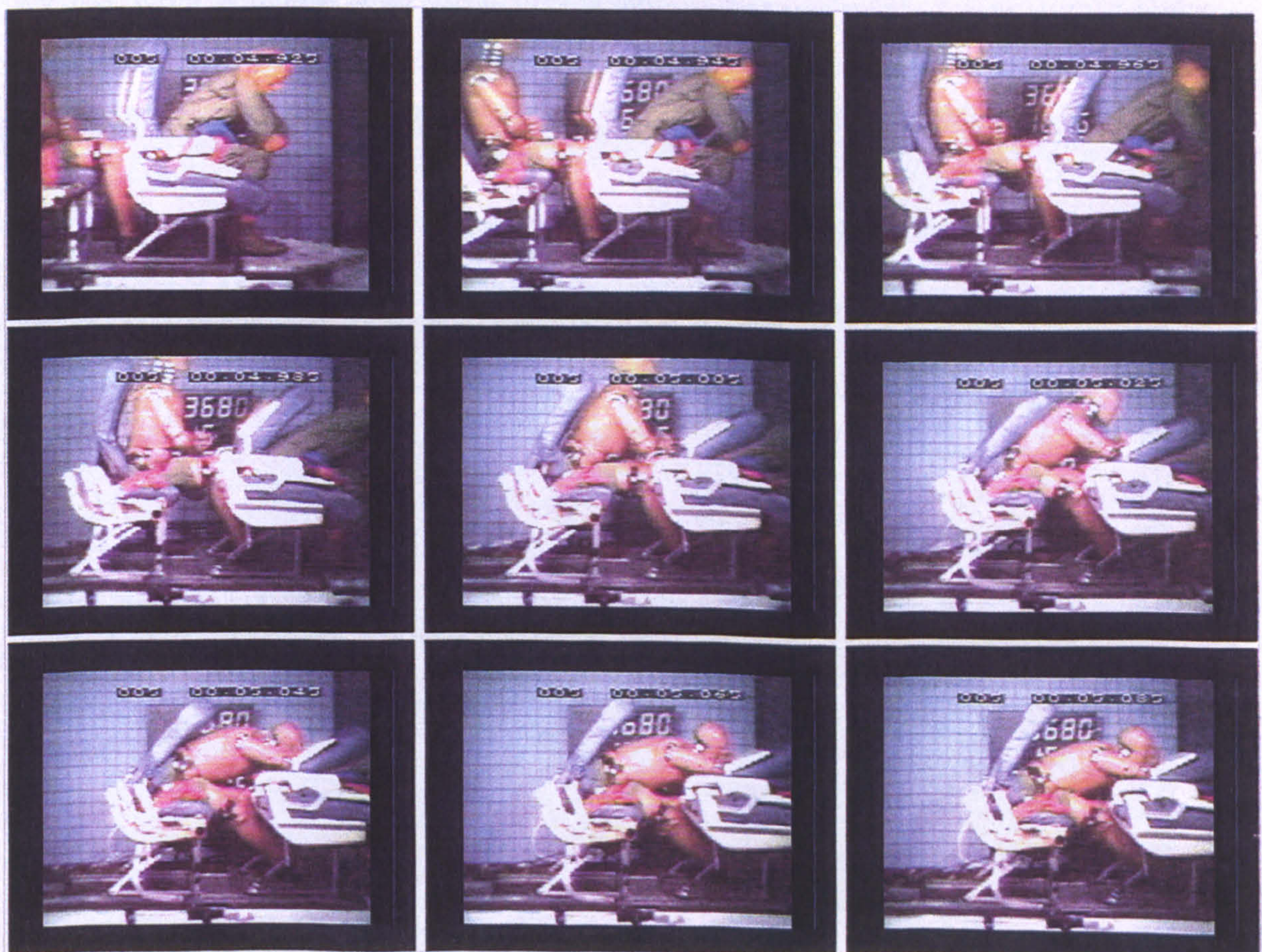
Fig. 17 Run No. 3680 - Unbraced/Legs Forward, 28" Seat Pitch
