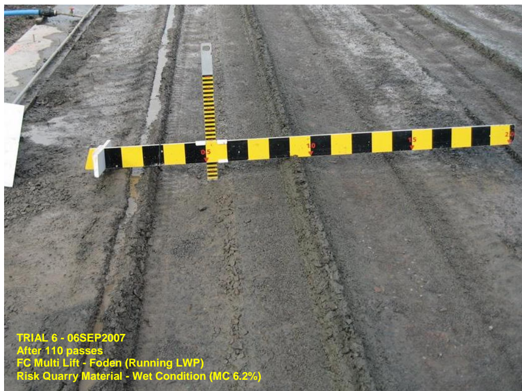
Figure 5.22 – Example of pictures taken in the wheel paths at the end of each round of passes
