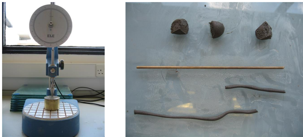
Figure 5.16 – (a) Penetrometer for Liquid Limit determination & (b) Plastic Limit Test
