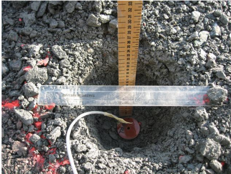
Figure 4.26 – Installation of a coil in Trial 10
