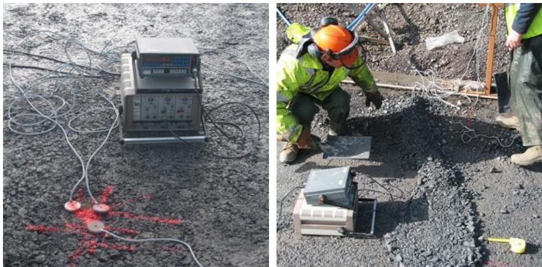
Figure 4.29 – Installation of the coils in the test section
