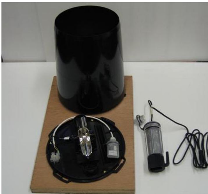
Figure 4.4 – Simplified weather station and shuttle reader for data-logger download
