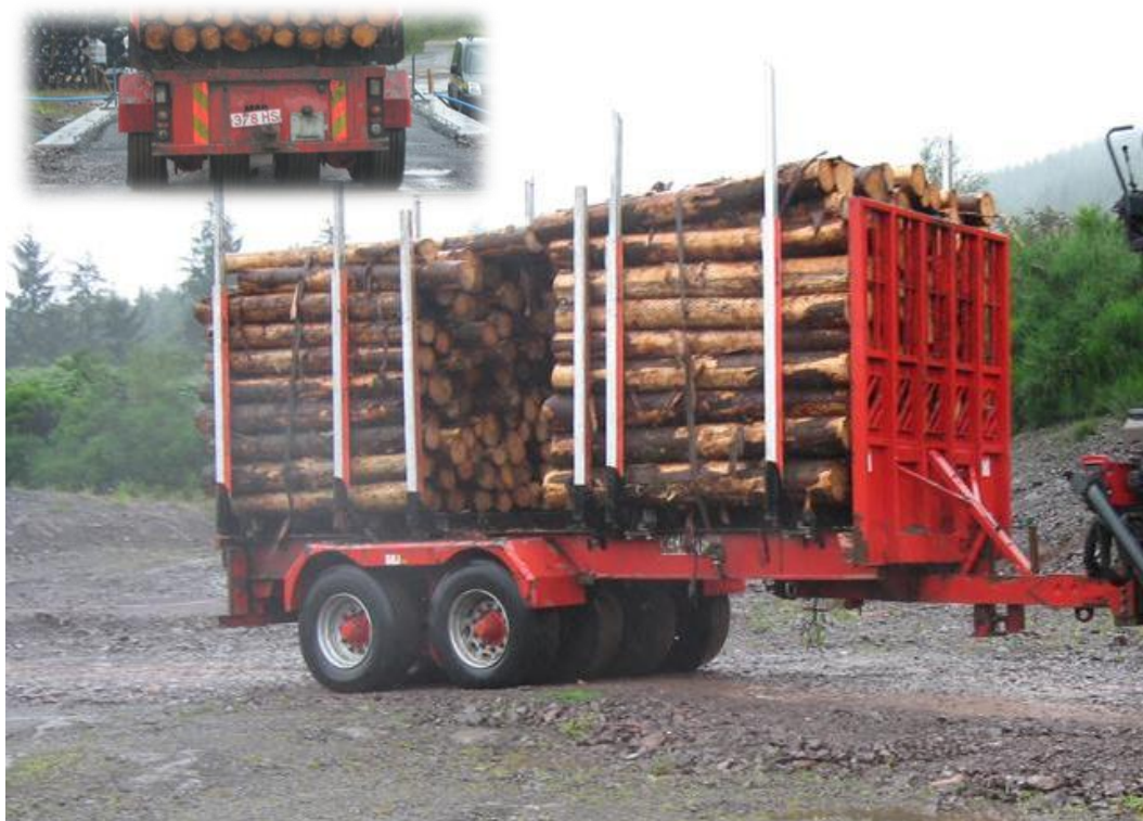
Figure 4.24 – “Low ground pressure” vehicle trailer with tyres equally spaced across pavement on stub-axes
