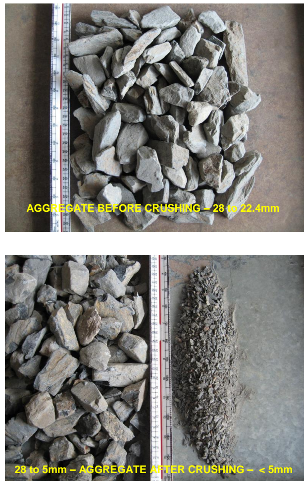
Figure 5.13 – Example of aggregate before and after TFB Test for Kilburn Hill material
