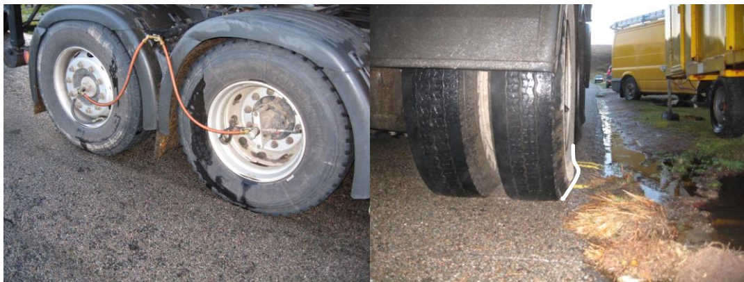
Figure 3.5 – TPCS Installed on a timber lorry in Scotland
