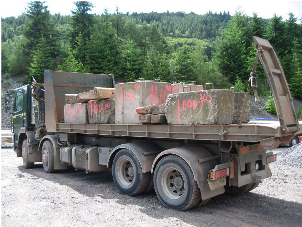
Figure 4.23 – FC Foden “Multi-Lift” truck trafficking a Ringour trial
