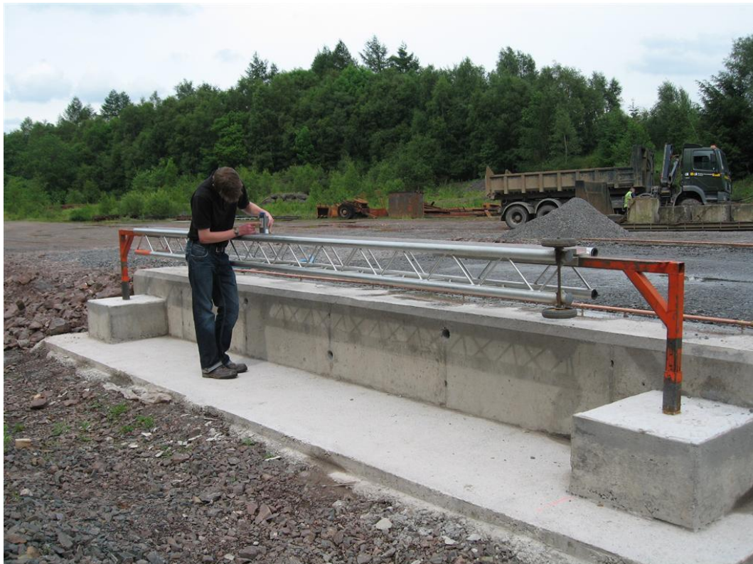
Figure 4.10 – Portable aluminium beam for rut profiling - at the calibration base.
