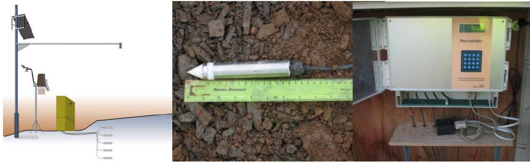
Figure 4.35 – (a) Schematic diagram of a Percostation Installation [Saarenketo 2006] (b) Percostation Probe (c) Percostation System
