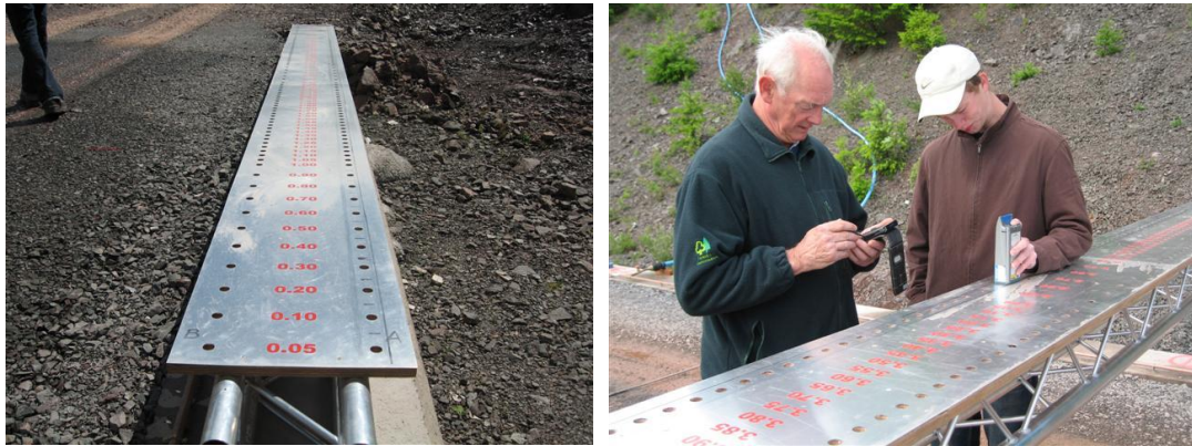
Figure 4.11 - Detail of the two sided beam with 0.1m spaced readings & recording procedure
