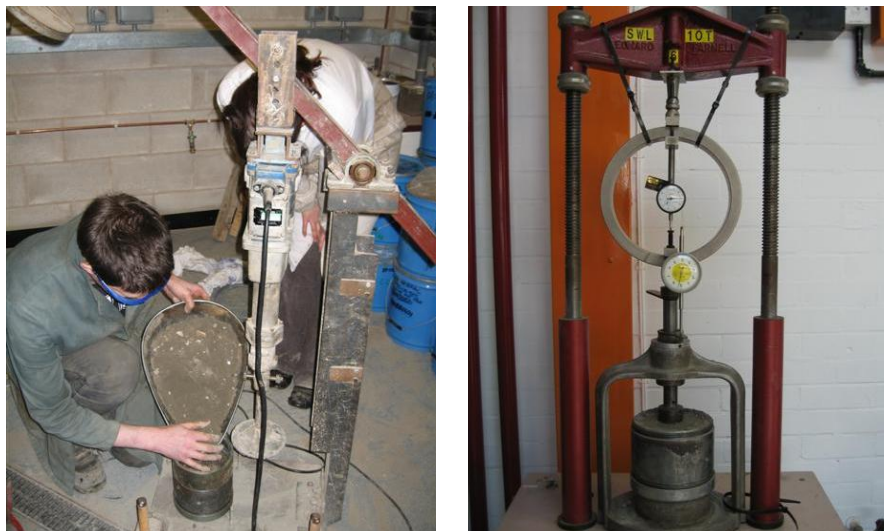
Figure 5.14 – Preparation and compaction of CBR samples & CBR Loading Apparatus
