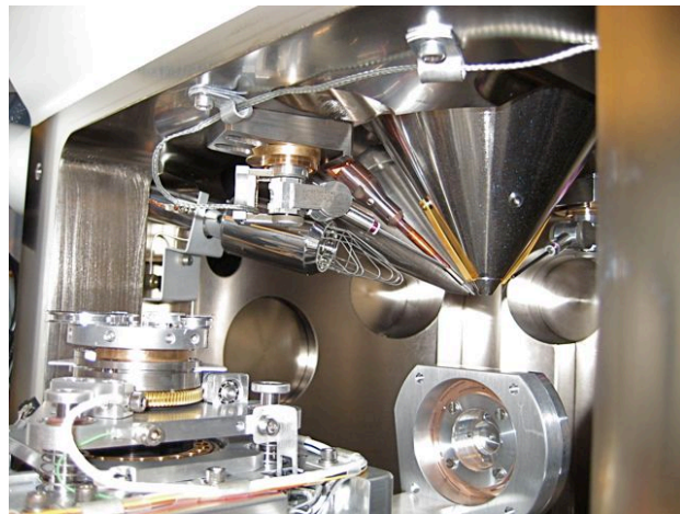
Figure 17-3: The vacuum chamber of the Zeiss NVision
