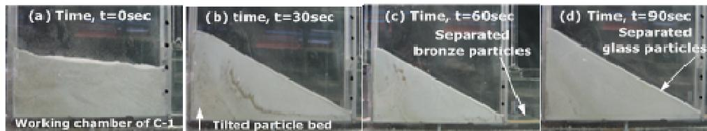
**Figure A.3: Time averaged (a-d) particle separation behaviour of a 90:10 %wt glass and bronze working mixture-A forming an initial average static particle bed height of 40mm in C-1.**
