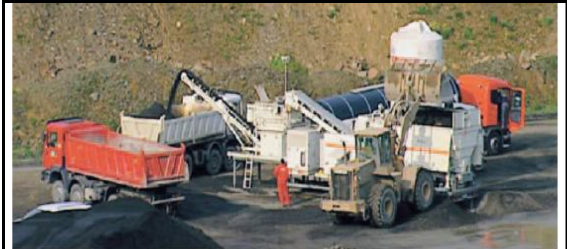
Figure 2.6: Cold Recycled Mix Plant (Wirtgen, 2005)
