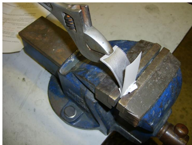
Figure 3-4. Detachment of a coating from the substrate by bending the substrate using a wrench tool.
