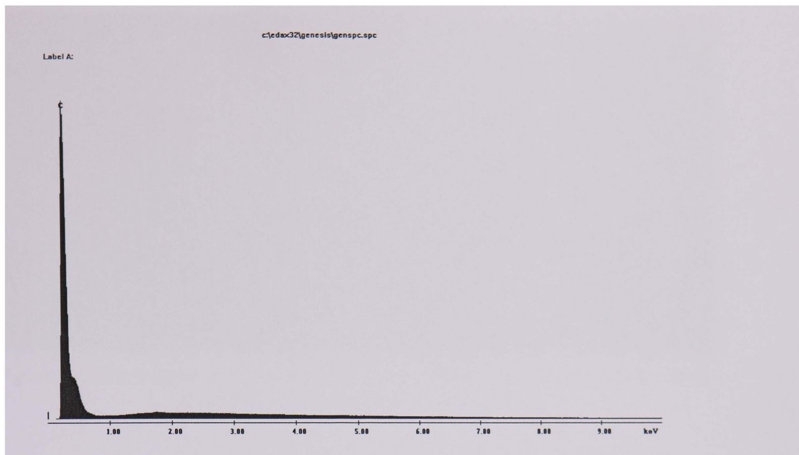
Figure 5.3 SEM EDAX spectrum of plain carbon cloth D
