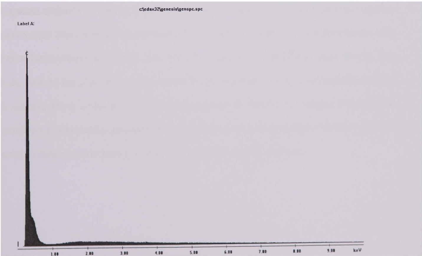
Figure 5.2 SEM EDAX spectrum of plain carbon cloth B
