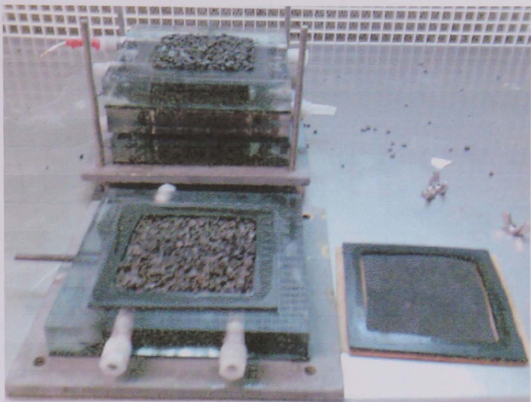
Figure 4.7 Actual assembly of stacked MFC
