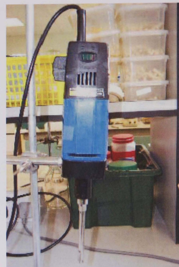
A.10 High shear mixer: Janke and Kunkel, Ultra-turrax T25
