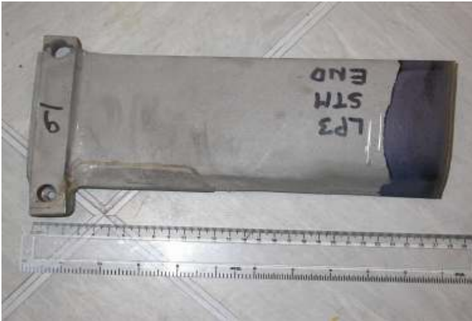
Figure 6.3 – A typical turbine blade tip to be hardness tested. The left end is the very end of the blade and the right end is where it has been cut from the rest of the blade.
