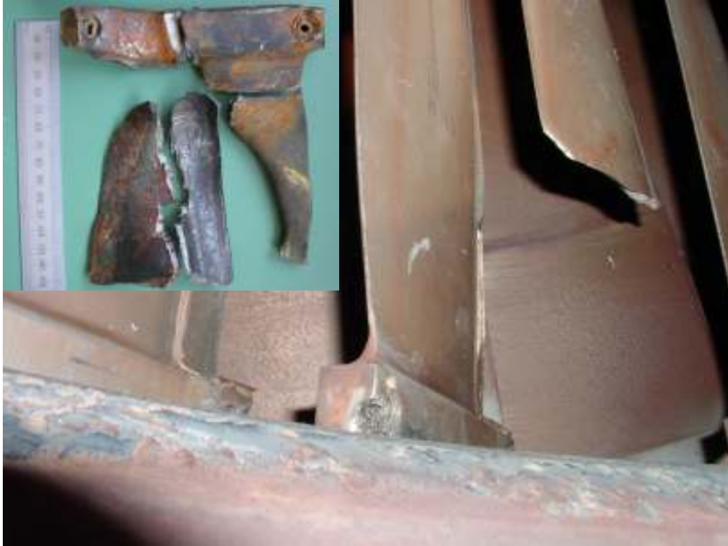
Figure 6.2 – Image of the Didcot A failure, inset -the failed turbine blade tip.
