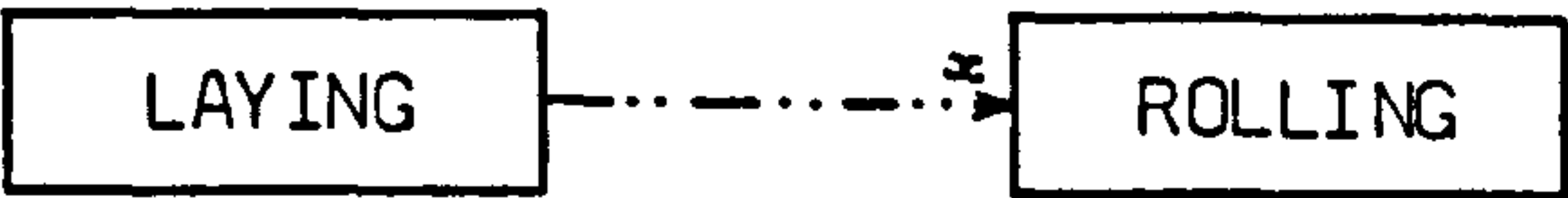
Figure (4.2.2.1) Must link for Macadam Laying
