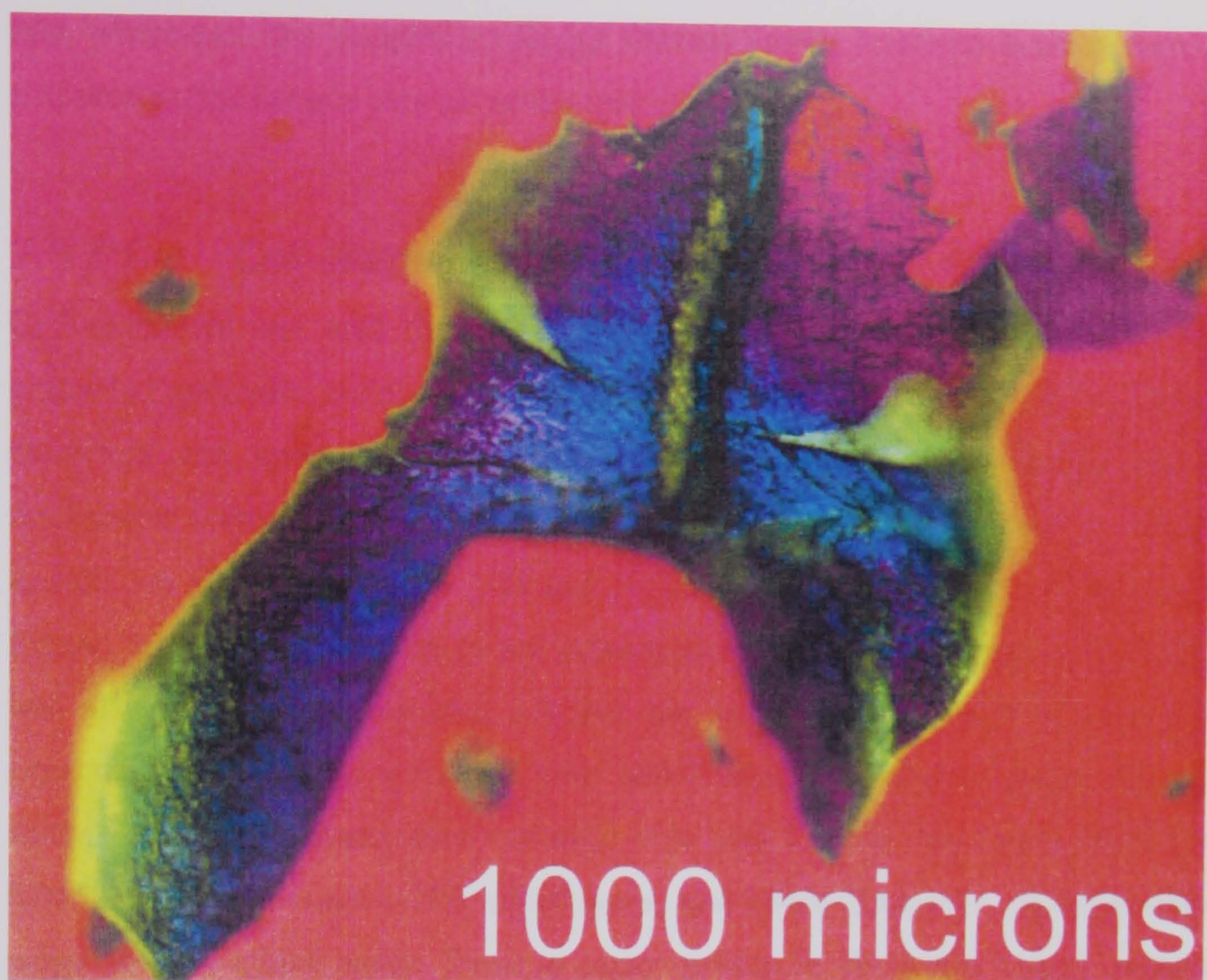
Figure 7-33 A fragment of conventionally puffed rice. Viewed through two polarising filters and a quarter wave plate.
