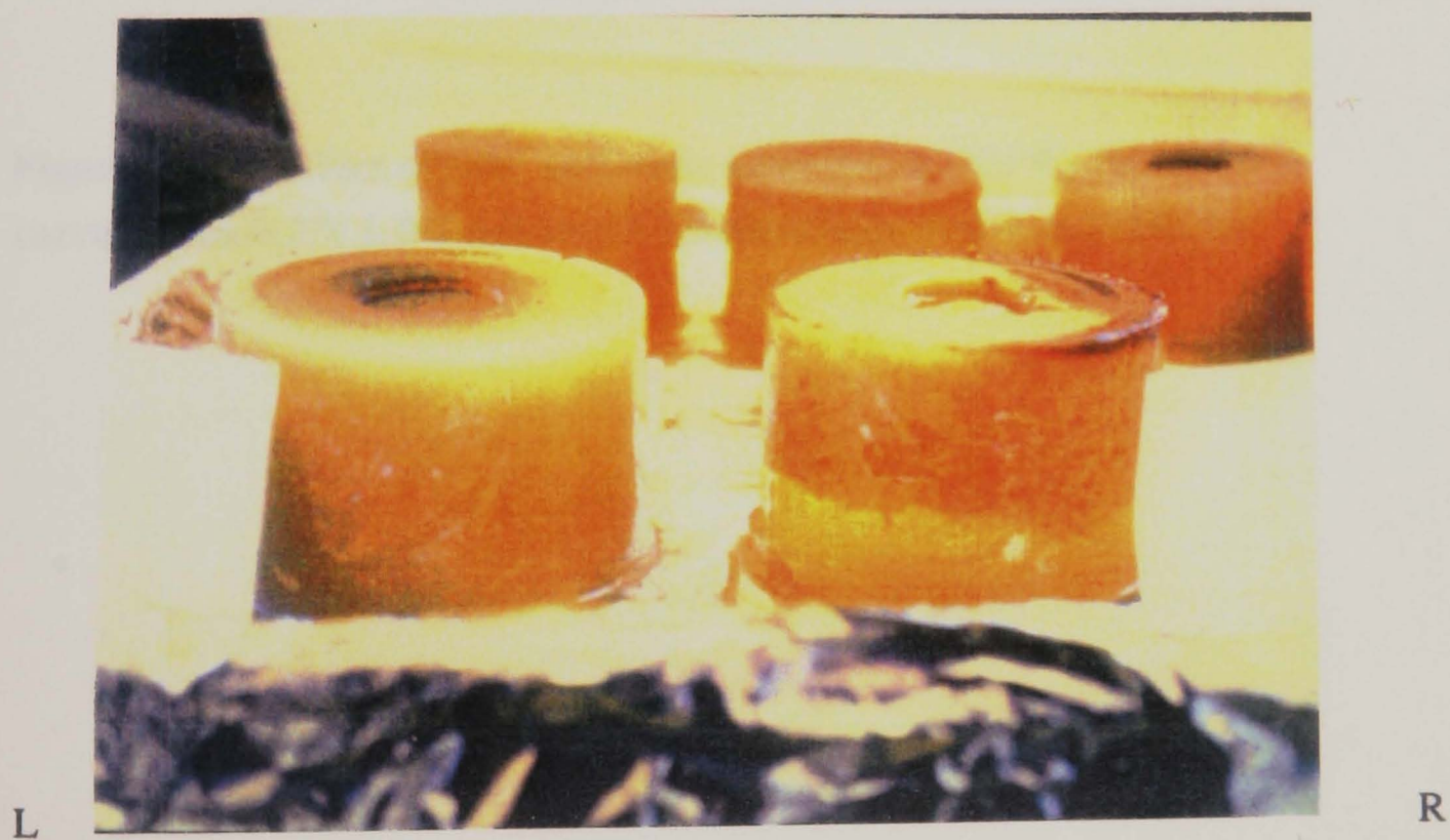
(b) Comparison of effects of autoclaving on 0.5% DBP gel (in the foreground of photograph). Gels shown inverted. Left = non-autoclaved; Right = autoclaved.
