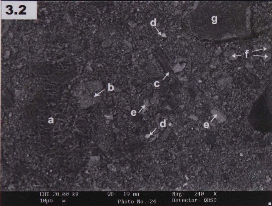
Figure 3.2: A CryoSEM BSE image of Smethwick canal sediment from a depth of 15cm, showing the general fabric of the mud. Detrital and authigenic particles in the mud include: a large mass of Fe and S rich mineralised organic matter (a); an agglomerate of clay and Fe-oxide (b); coal particles (c); Zn sulphides (d); vivianite crystals (e); quartz particles (f) and a large agglomerate of clay particles (g)
