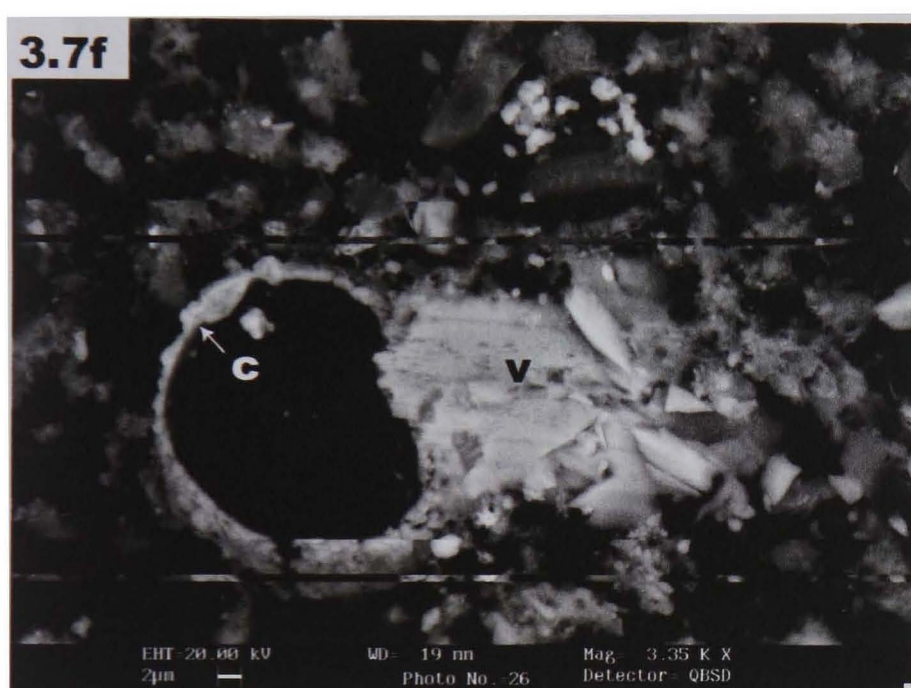
f: A partially etched grain of vivianite (v) adjacent to a hollow object, coated in Fe- carbonate (c), from a depth of 20cm in Great Bridge sediment
