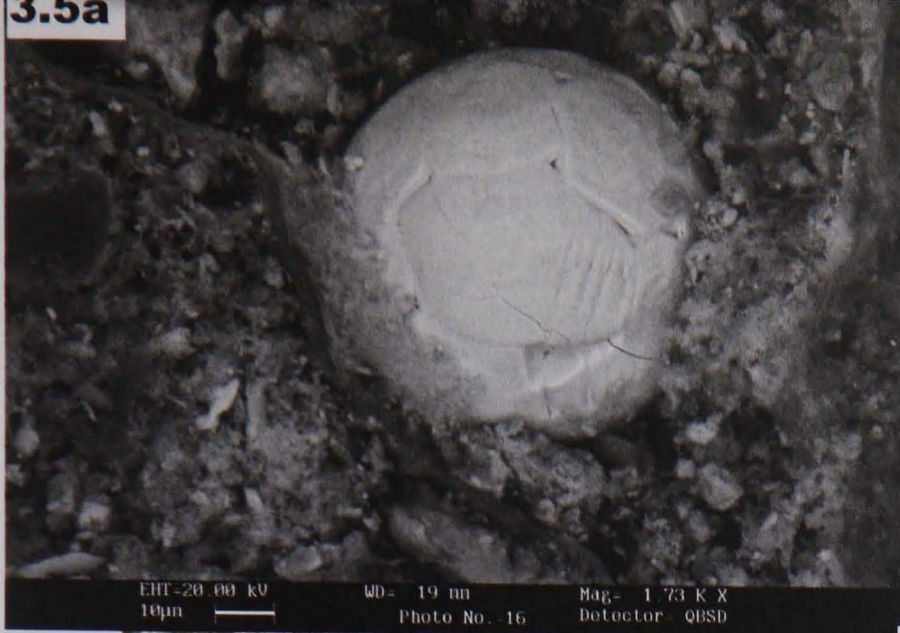
Figure 3.5: CryoSEM BSE images of detrital anthropogenic particles in Great Bridge canal sediment
