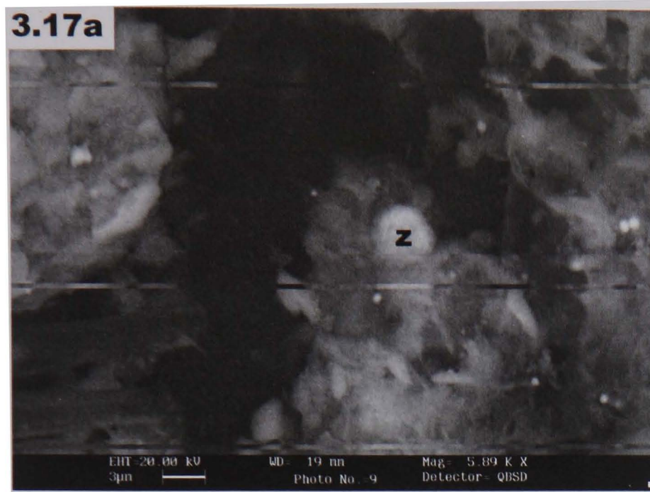
Figure 3.17: CryoSEM BSE images of zinc sulphides in Snarestone sediment
