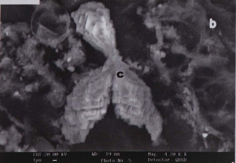
Figure 3.13: A CryoSEM BSE image of an authigenic calcite grain with a delicate stepped morphology (c) on a substrate of floccular clay and wispy biofilm (b), from the sediment water interface at Smethwick
