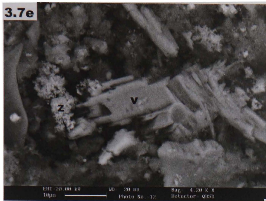
e: A partially etched grain of vivianite (v), adjacent to spongy grains of ZnFe-sulphide (z) from a depth of 25cm in Smethwick sediment
