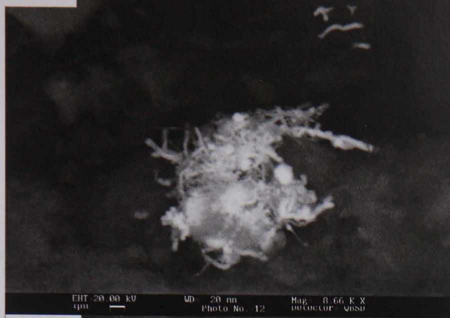
Figure 3.12: CryoSEM BSE images of authigenic silver and gold particles in urban canal sediment
